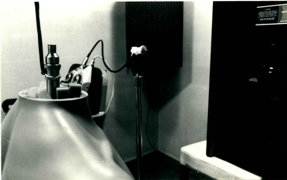
Figure 8. The sound field system used to measure signal sound pressure level.
