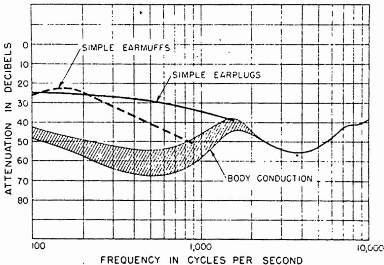
Figure 2. Theoretical maximum attenuation available from personal hearing protectors (Zwislocki, 1958).
