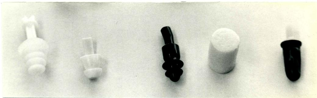
Figure 13. Earplugs used in the study. Left to right; Multiflanged disposable, single flanged, multiflanged, polymer foam and moldable.
