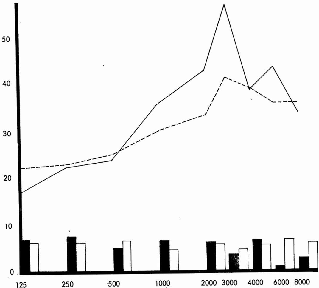
Figure 15. Means (solid line) and standard deviations (solid bars) of insertion losses resulting from placement of the single flanged V.51-R earplug in the manikin left ear. Comparative means and standard deviations (Broken lines and open bars) of attenuation values of the same earplug reported for NIOSH by Kroes, et. al. (1975).
