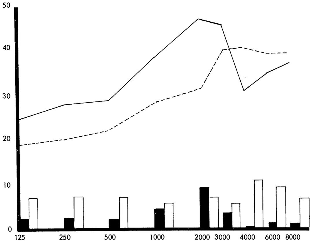
Figure 17. Means (solid line) and standard deviations (solid bars) of insertion loss resulting from placement of the multi-flanged disposable earplug in the manikin left ear. Comparative means and standard deviations (broken line and open bars) of attenuation values of the same earplug reported for NIOSH by Kroes, et. al. (1975).
