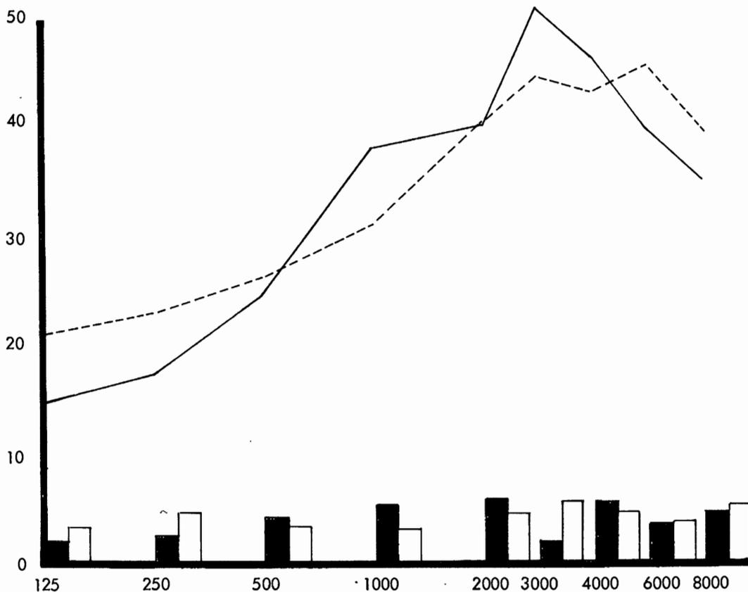
Figure 18. Means (solid line) and standard deviations (solid bars) of insertion loss resulting from placement of the moldable earplug in the manikin left ear. Comparative means and standard deviations (broken line and open bars) of attenuation values of the same earplug reported for NIOSH by Kroes, et. al. (1975).
