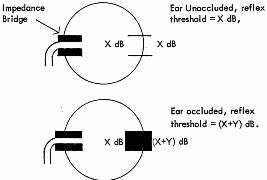
Figure 6. The acoustic reflex procedure of testing attenuation. The increased sound pressure level required to elicit the acoustic reflex ( $Y$  dB) represents the attenuation provided by the earplug.
