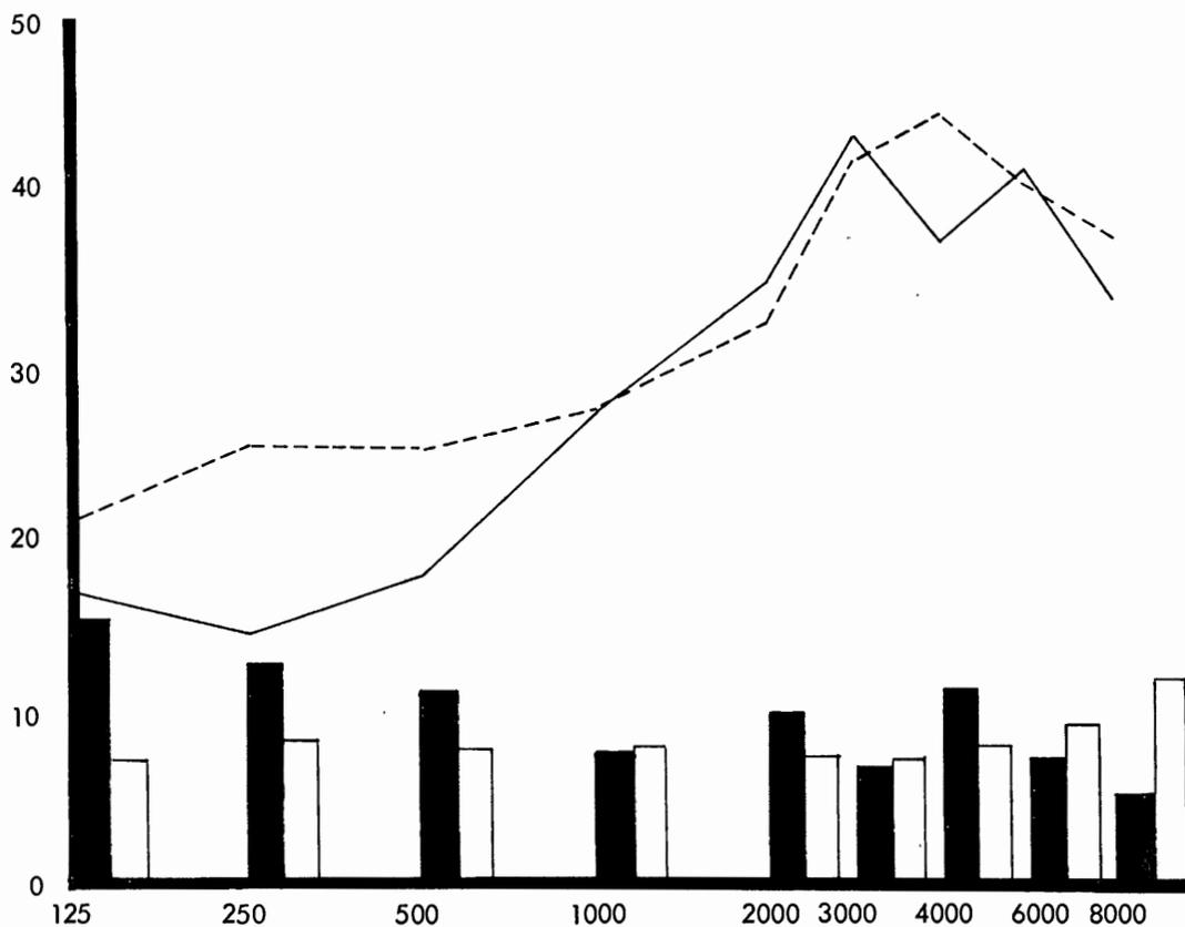
Figure 16. Means (solid line) and standard deviations (solid bars) of insertion loss resulting from placement of the multi-flanged earplug in the manikin left ear. Comparative means and standard deviations (broken lines and open bars) of attenuation values of the same earplug reported for NIOSH by Kroes, et. al. (1975).
