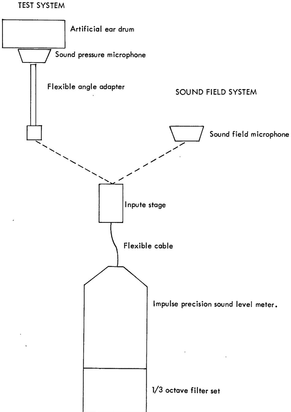
Figure 10. The experimental test system and coincident sound field system showing shared components (dotted line).
