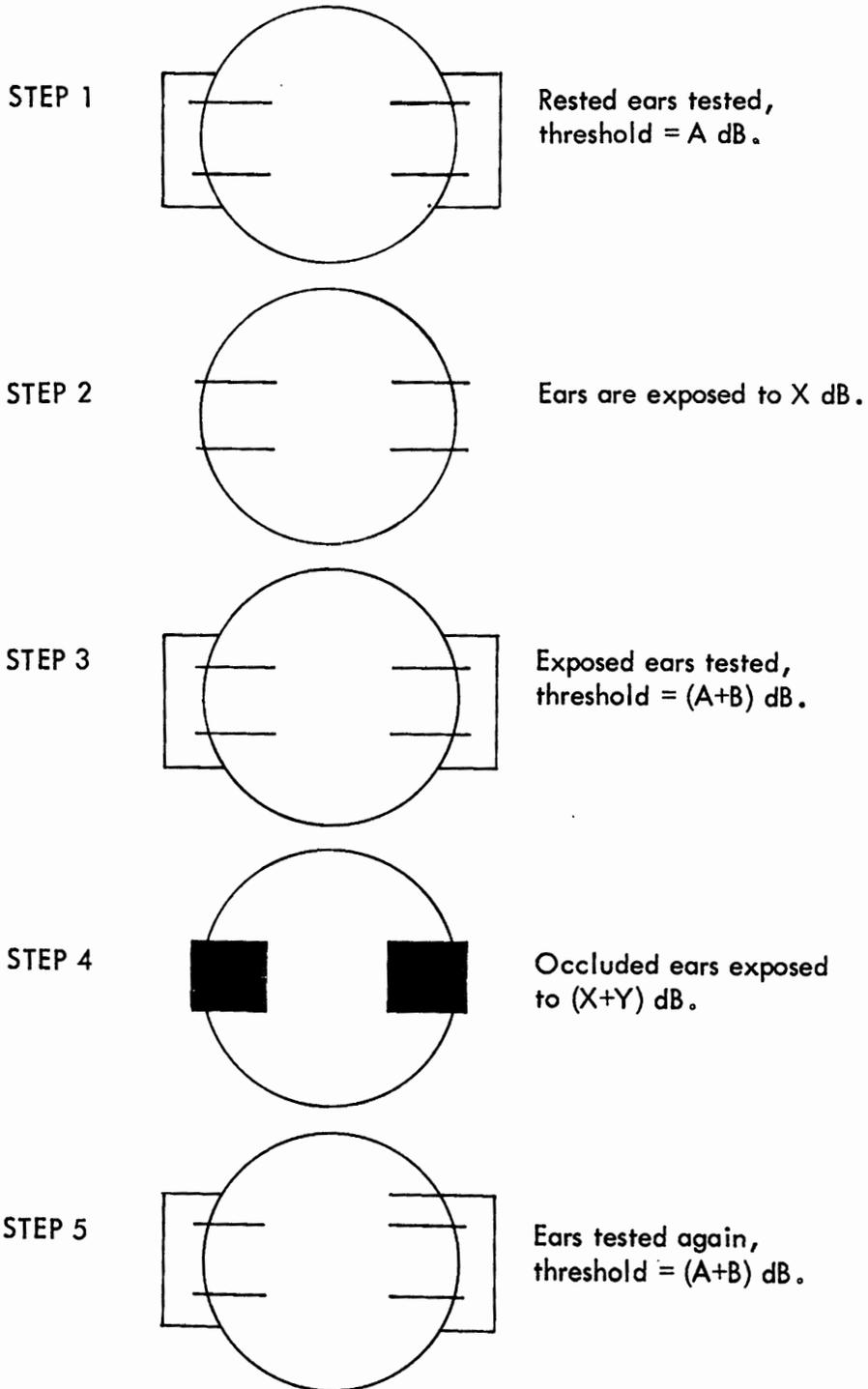
Figure 5. The temporary threshold shift procedure of testing attenuation. The increased sound pressure level (Y dB) required to produce a temporary threshold shift (B dB) represents the attenuation provided by the earplug.
