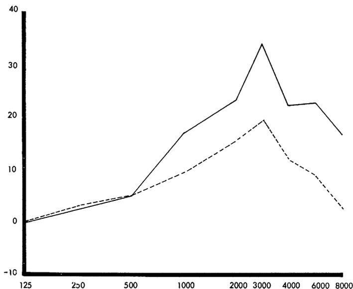
Figure 20. Adjusted insertion loss means of five earplugs (solid line) compared with the manikin open ear frequency response (broken line).
