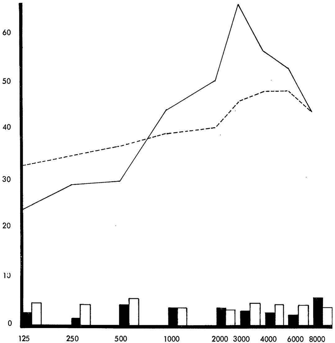
Figure 19. Means (solid line) and standard deviations (solid bars) of insertion loss resulting from placement of the polymer earplug in the manikin left ear. Comparative means and standard deviations (broken line and open bars) of attenuation values of the same earplug reported for NIOSH by Kroes, et. al. (1975).
