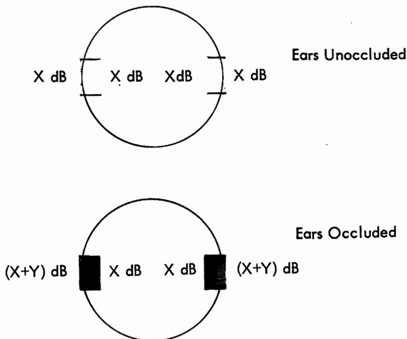
Figure 3. The threshold shift procedure of testing attenuation. The increased sound pressure level needed to produce X dB behind the earplug (Y dB) represents the attenuation provided by the earplug.
