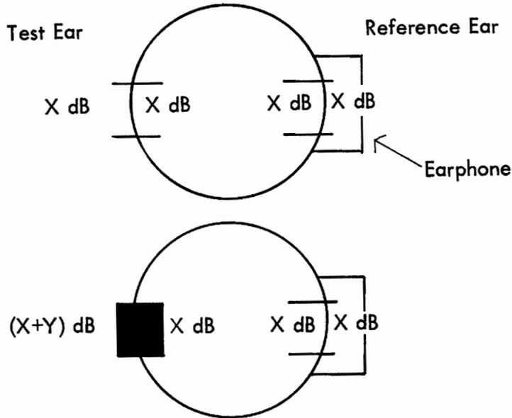
Figure 4. The loudness balance procedure of testing attenuation. The increased sound pressure level needed to produce  $X$  dB behind the earplug, causing the subject to perceive equal loudness between ears ( $Y$  dB), represents the attenuation provided by the earplug.
