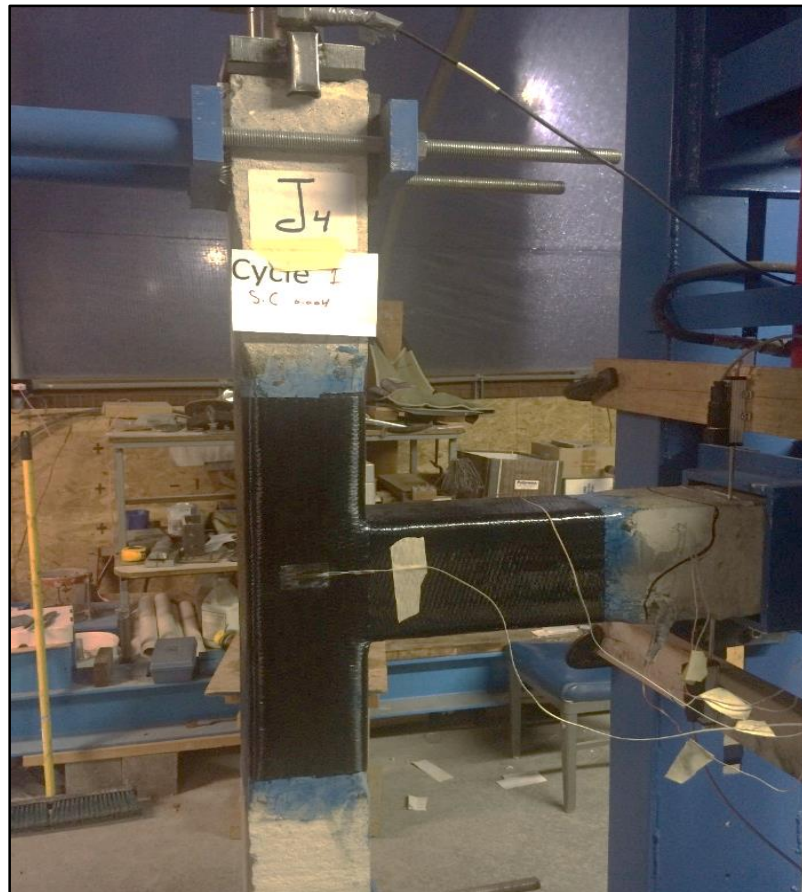
Figure 4-28 Specimen J4 at the Failure
