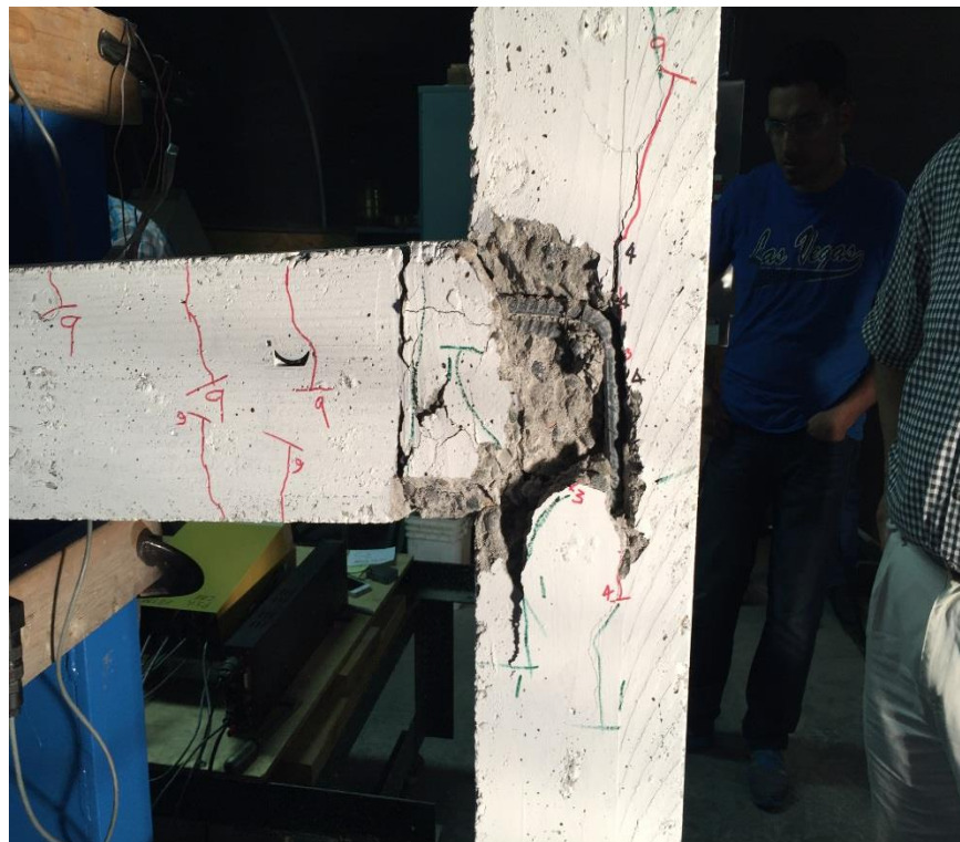
Figure 4-19 The Failure Pattern of Specimen J2
