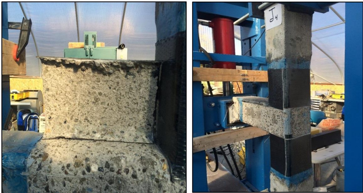
Figure 4-29 Areas under CFRP Sheets at the End of the Test, Specimen J4
