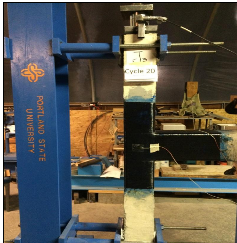
Figure 4-23 Specimen J3 at the End of Cycle 20, Strain Control Phase
