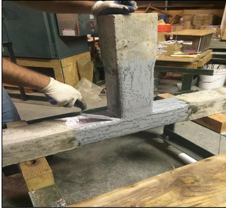
Figure 3-24 Applying the Putty Layer to the Concrete Surface
