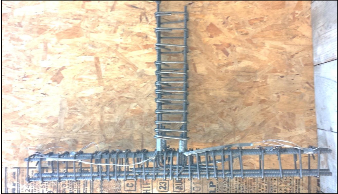
Figure 3-9 Reinforcement Cage of Specimen J1
