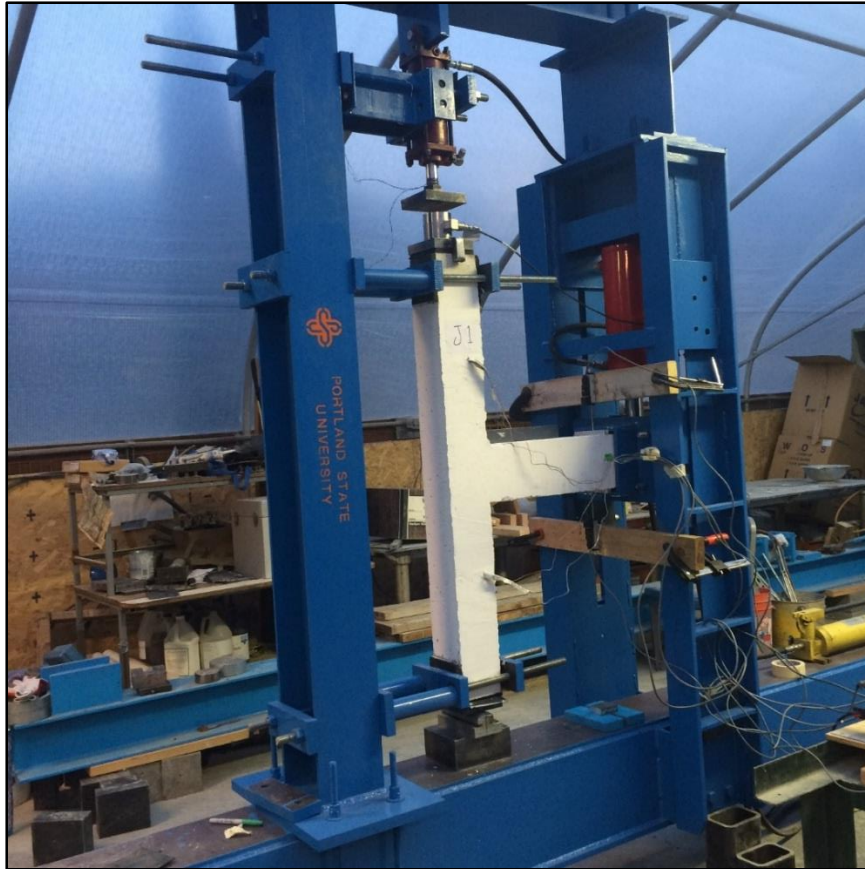
Figure 4-1 Test Setup of Joint J1
