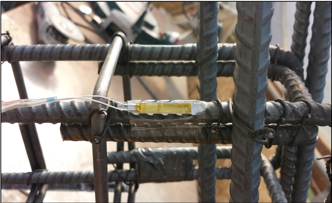
b- Strain Attachment
