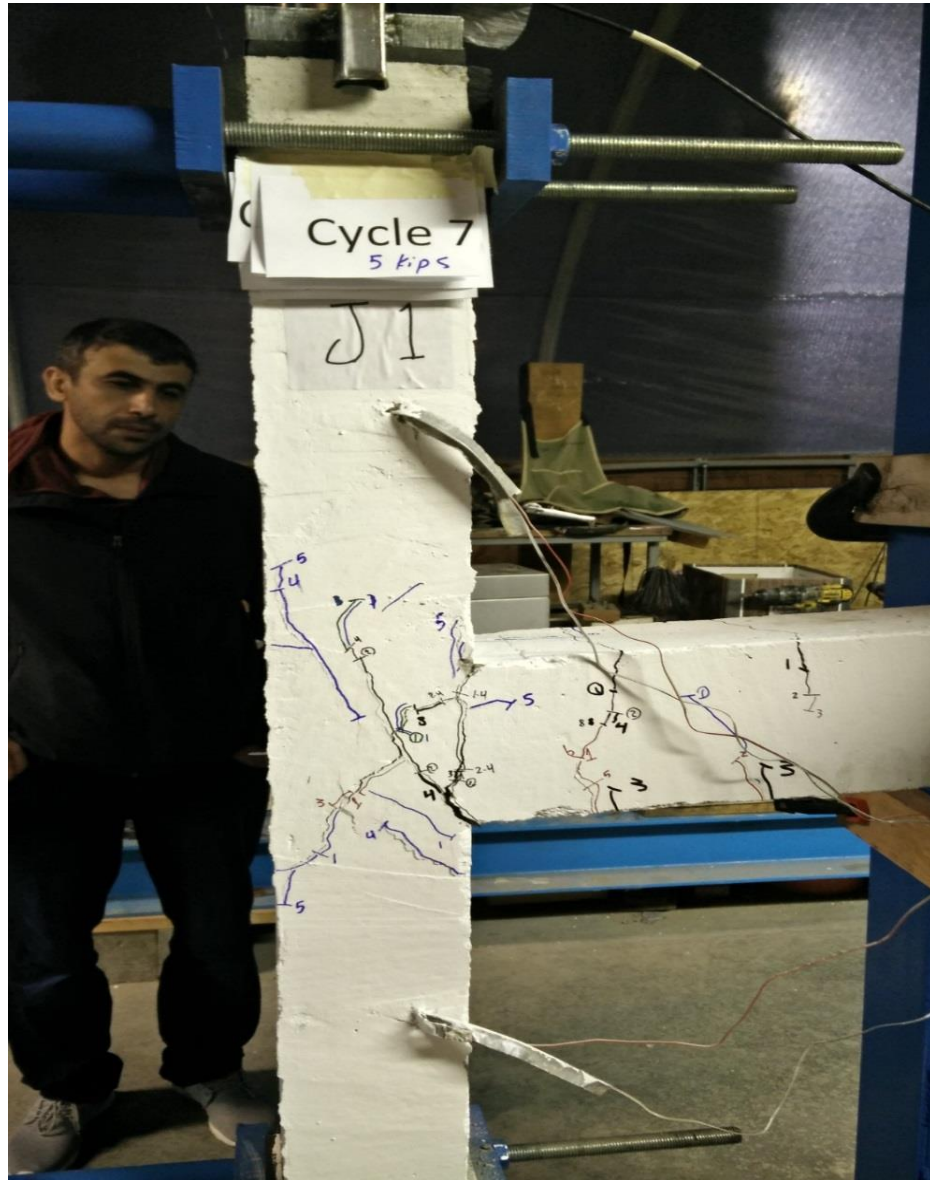
Figure 4-7 Concrete Cover Splitting, J1
