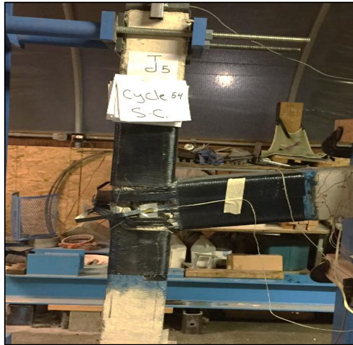
Figure 4-34 Failure of Specimen J5
