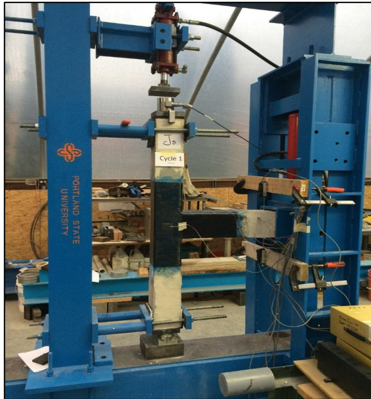
Figure 4-21 Test Setup of Specimen J3
