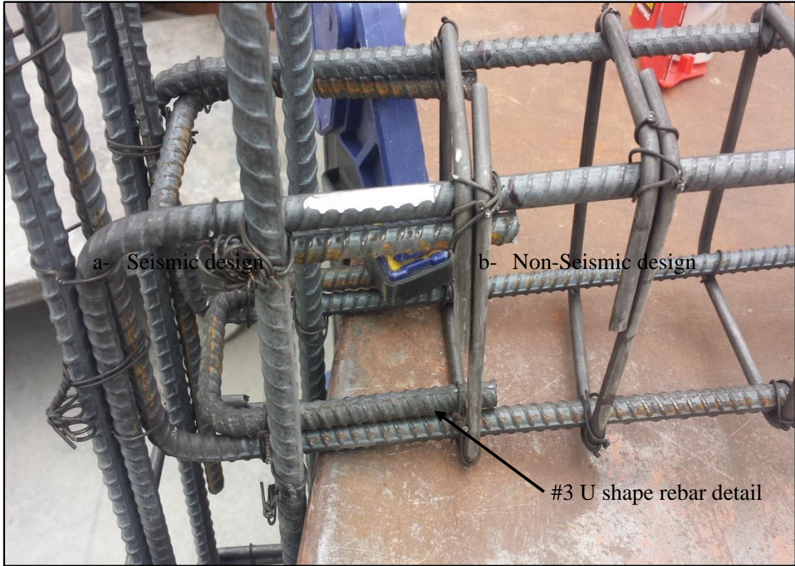
Figure 3-6 “U” Shape Rebar Detail
