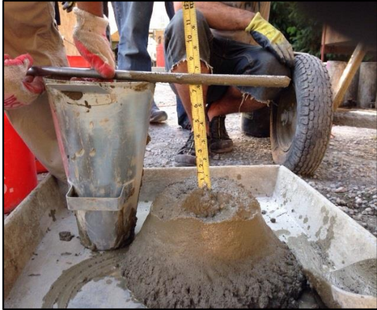
c- Slump test
