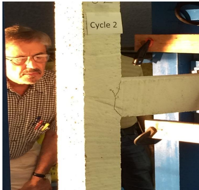
Figure 4-13 The Cracks of Joint J2 at the End of Cycle 2
