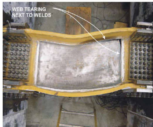
Figure 2.6: Ultimate failure of link L225.
