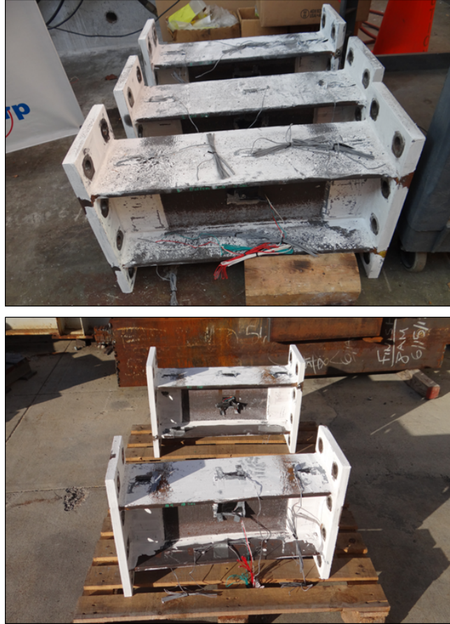
Figure 6.23: Deformed shear links after testing the LCF-5L specimen.
