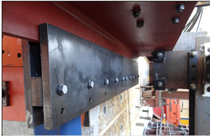
Figure 5.27: Sliding mechanism B at first floor level.
