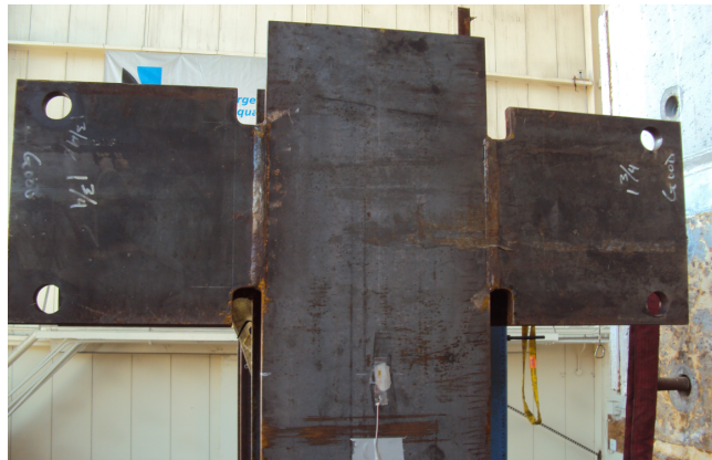
Figure 5.21: Actuator spreader beam located at the second floor.
