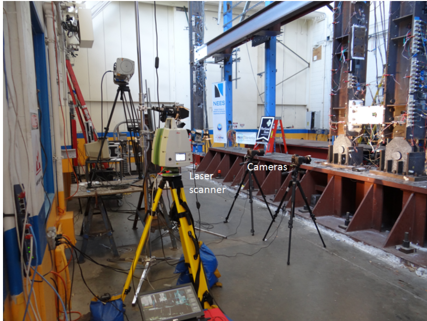
Figure 5.36: Cameras and laser scanner used on LCF test assembly.
