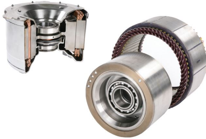
Figure 2.8: Remy HVH250 cutaway, internal permanent magnet rotor and stator with rectangular windings for increased torque density.[32]
