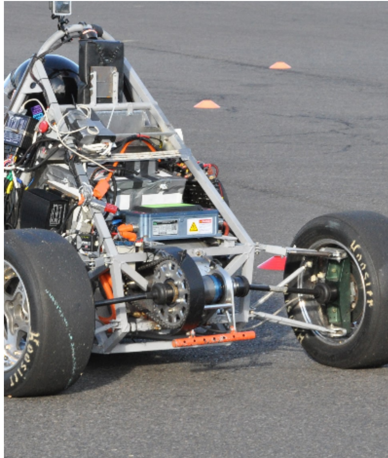
Figure 2.4: rear of car, view of drivetrain components, including chain drive, rear sprocket used in gear reduction, differential, half shafts.[16]
