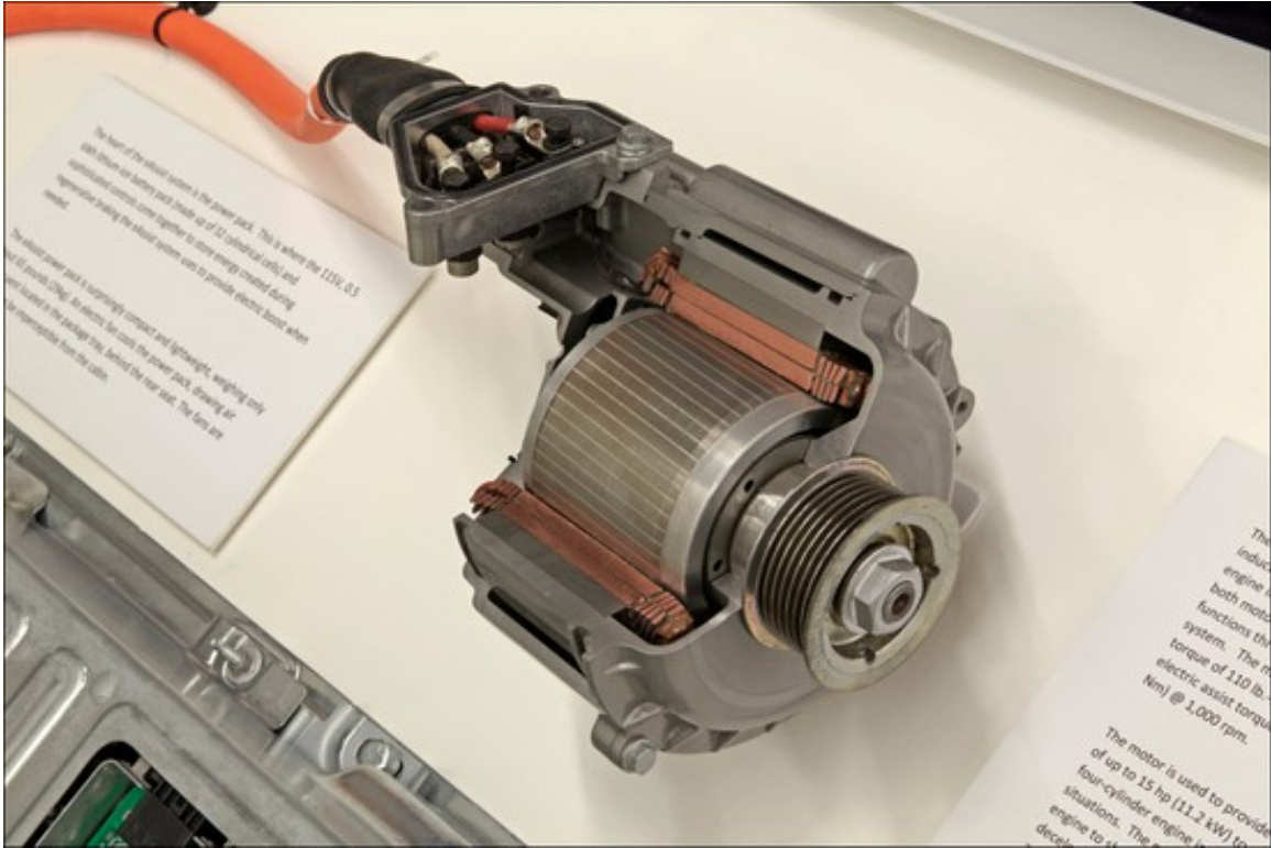
Figure 2.13: GM eAssist induction motor cutaway of motor housing showing stator windings and rotor cage with aluminum bars, which varies from the smooth exterior of the Remy PMSM.[37]
