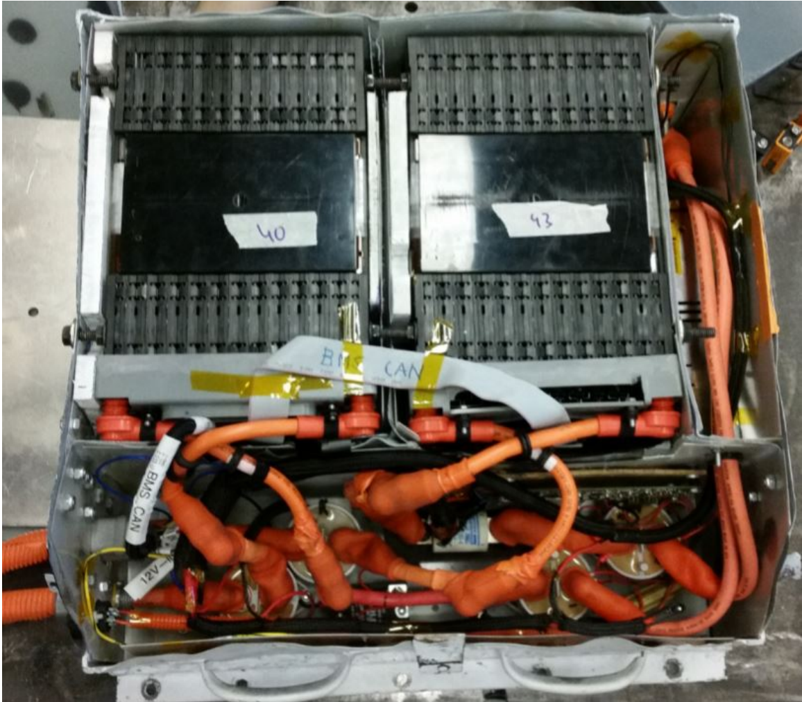
Figure 2.20: Battery container from the second generation car, designed from steel to secure the battery modules and high voltage components.
