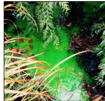
Figure 17: Tracer dye study 12 December 2015 showing full dispersal and good mixing
