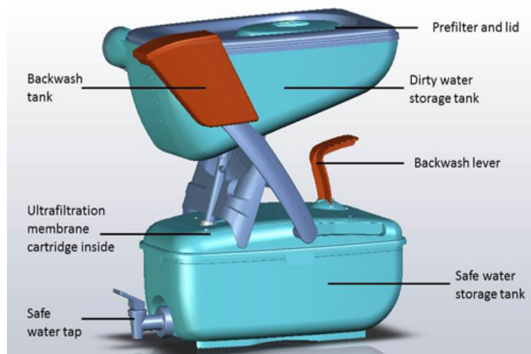
Figure 2: Vestergaard Frandsen LifeStraw Family 2.0 [2]. Tabletop water filter designed for households in developing countries.
