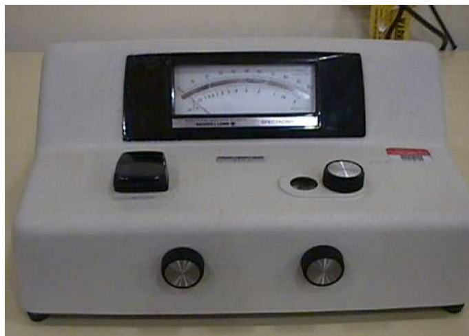
Figure C-2 Image of Spectronic-20, an example of a simple spectrometer that can be used for analysis of \text{NO}_2 passive samplers.
