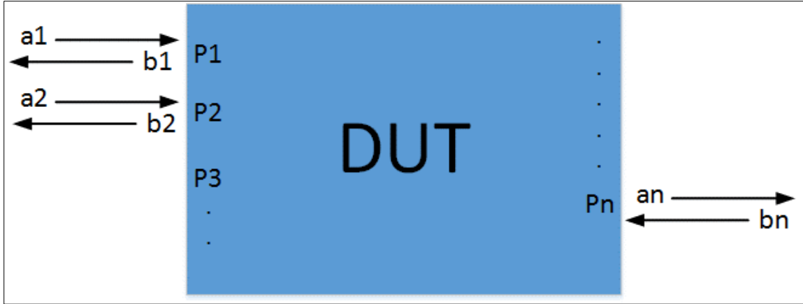
Figure 19, Incident and egressing voltage waves.
