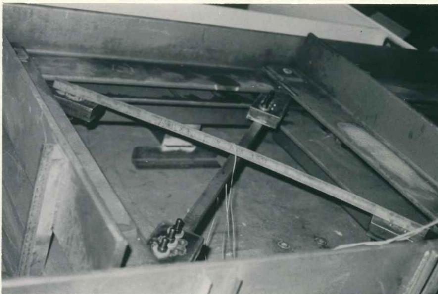
Figure 42. Indeterminate truss with diagonal bracing.
