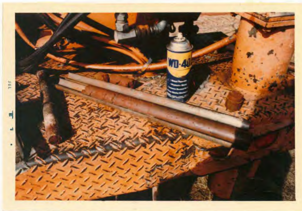
Figure 3. Drive core taken as part of drilling operation.
