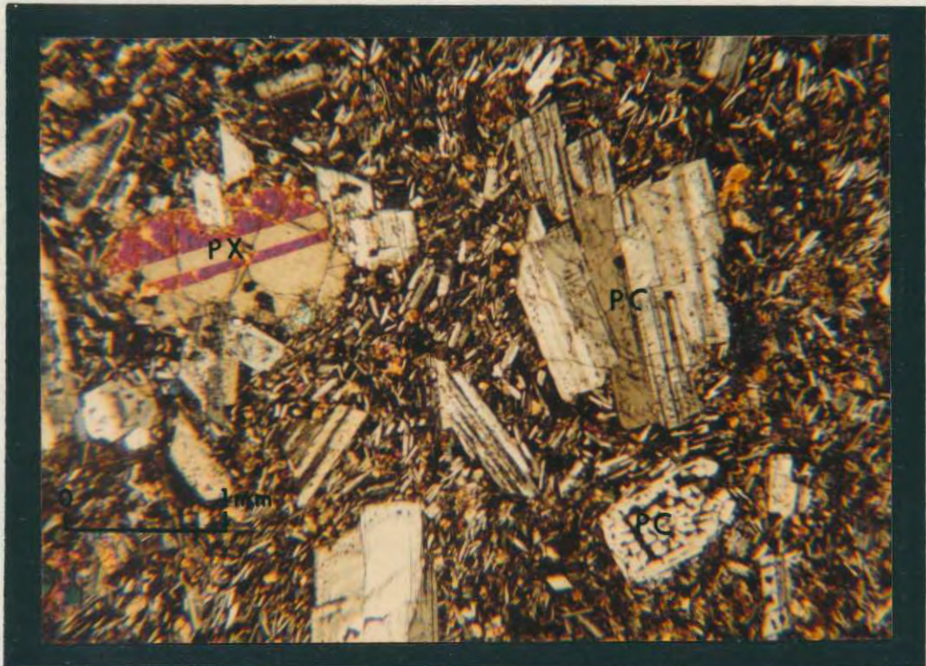
Figure 14. A Photomicrograph of a typical Skamania basalt (CG-10) under crossed nicols. Phenocrysts consist dominantly of plagioclase (PC) and pyroxene (PX) with occasional phenocrysts of olivine (Olv) or magnetite (MT). B. Photomicrograph of a typical Skamania andesite (CG-45) under crossed nicols. Note the corroded and broken outlines and sieve textures displayed by the plagioclase (PC) phenocrysts.
