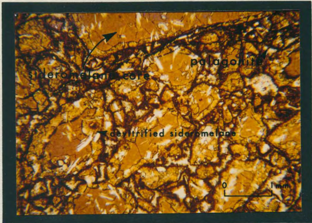
Figure 33. Photomicrograph of Priest Rapids hyaloclastite (PPL) collected from the base of the north face of Crown Point, Oregon. The sand-size hyaloclastite grains commonly have an outer layer of palagonite (opaque) which surrounds a layer of devitrified sideromelane (brownish-yellow) that varies in thickness. Most grains have a core of unaltered sideromelane (brown).
