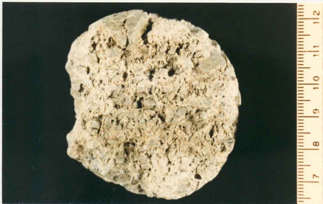
Figure 28. Photograph of core sample of the tectonic breccia. Sample taken from SM24. See Table I.
