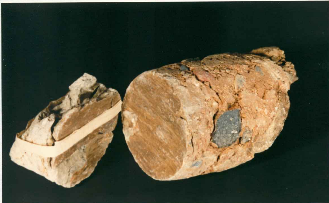
Figure 37. Photograph of the slip plane material. 2\frac{1}{2} " core sample taken from SM36, see Table I.
