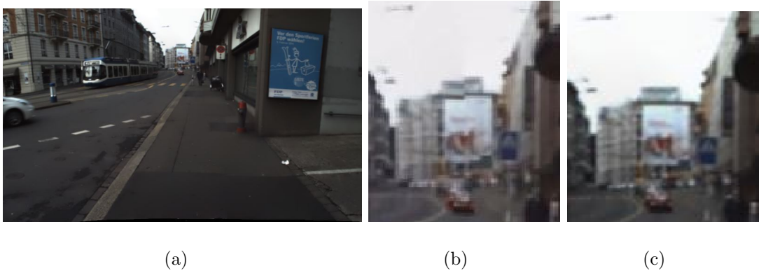
Figure 5.8: Comparisons between two video stitching methods. From left to right, the close-ups show comparisons to the methods: (b) Autopano Pro, (c) our result. Autopano Pro result has misalignment around the advertisement sign area. In contrast, our result does not introduce misalignment.
