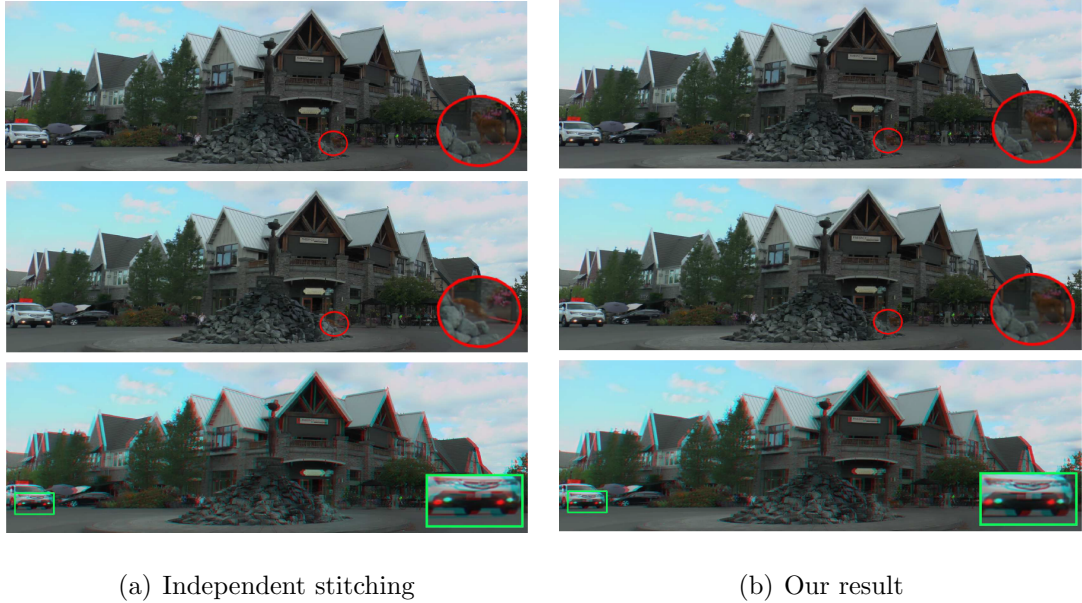
Figure 4.1: Stereoscopic panorama stitching. For each column, we show the left-view, right-view and red-cyan anaglyph of the stereo panorama. Stitching the left- and right-view panorama independently brings in inconsistency artifacts like monocular object (the cat) and vertical disparities (the car headlights), which will cause “3D fatigue” to viewers. Our result is free from these artifacts.
