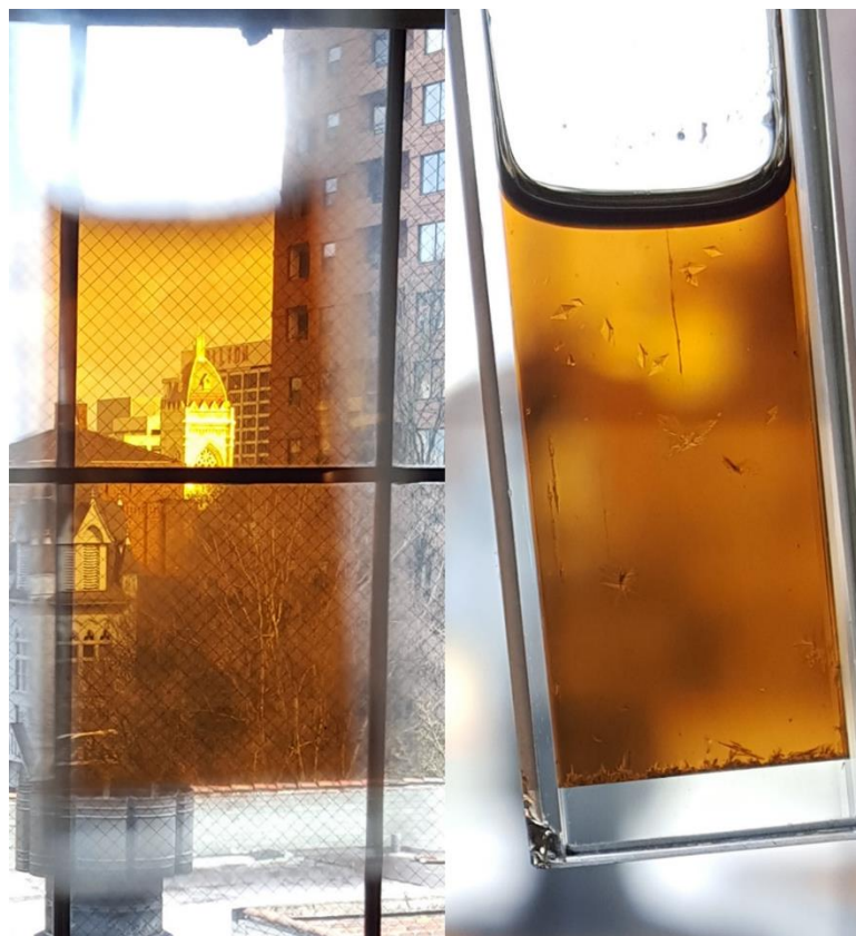
Figure S IV-6. Photograph of Oa-PbS QDs with 3-MPA/dDDdMABr added in a 20:20:1 ratio of [3-MPA]:[dDDdMABr]:[Oa - ] after ~48 hours of aging. The suspension remains optically transparent (left), while faceted crystals of dTdPA are observed floating in solution if the focal plane is aimed inside the cuvette (right).
