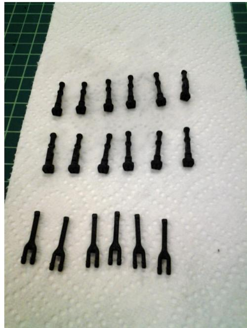
Figure 3.12: 3D printed parts after cleaning.
