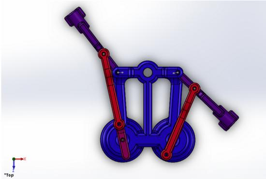
Figure 2.13: CAD model of the flapping wing mechanism [23]. Motors are connected to a planetary gear transmission (4:1 ratio), the output shaft of the transmission is then connected to rigid linkages that move the wings.
