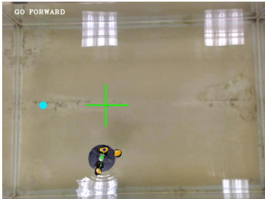
Figure 5.3: Best found solution for forward movement *Blue*: Initial position of the vehicle, *Green cross*: waypoint the vehicle was commanded to reach. The experiment was stopped once the center of vehicle crossed the  $y$ -axis of the waypoint. The four white rectangles are reflections of the ceiling lights and are not related to the experiment.
