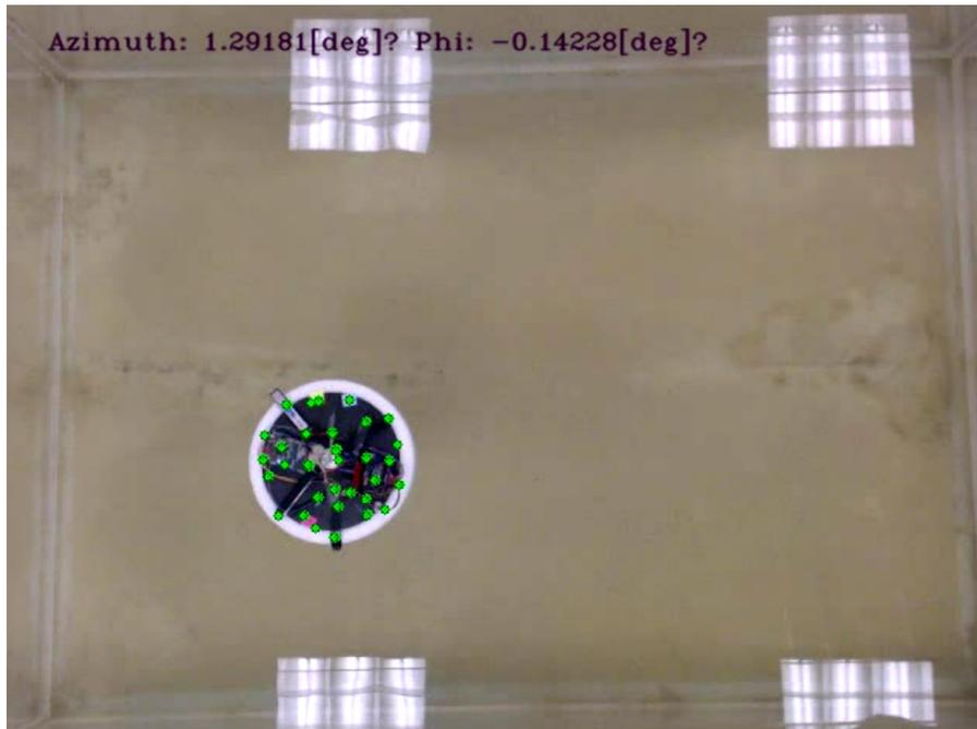
Figure 3.9: An example run of the tracking algorithm based on LKT and SURF: Shortly after the initialization the azimuth estimate is precise (0 deg means the robot is facing directly towards the right)
