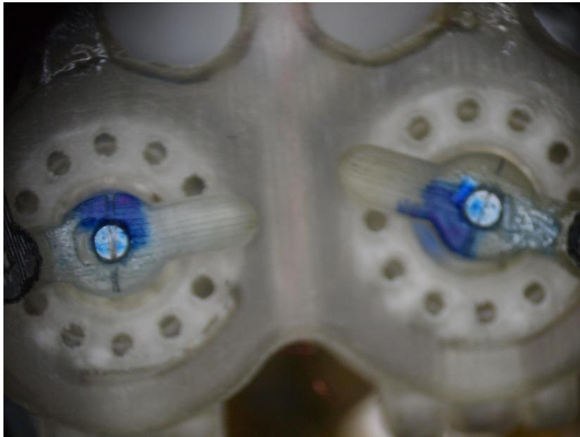
Figure A.10: Sealed shaft with markers to prevent shaft slippage
