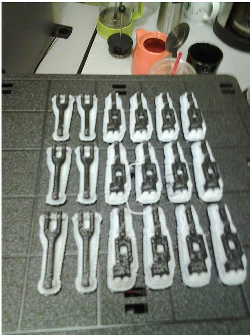
Figure 3.11: 3D printed parts. Notice the couplers on the left, and the left and right rockers on the right. Left and right rockers are identical.
