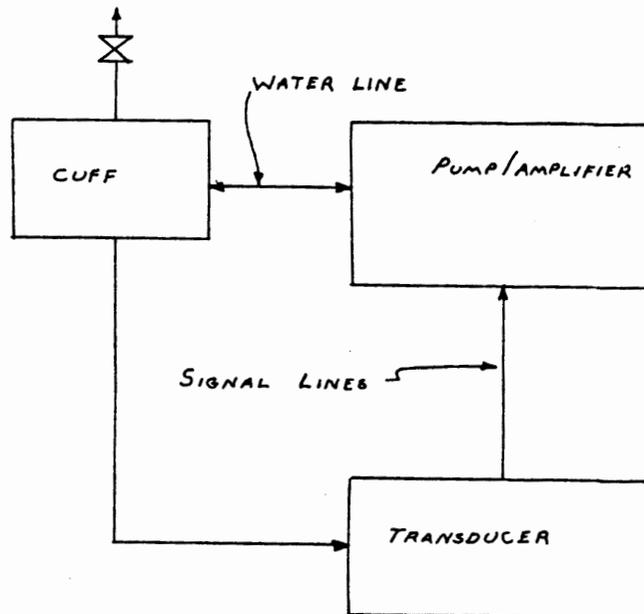
Figure 2. A block diagram of the HOC, transducer and pump/amplifier components.
