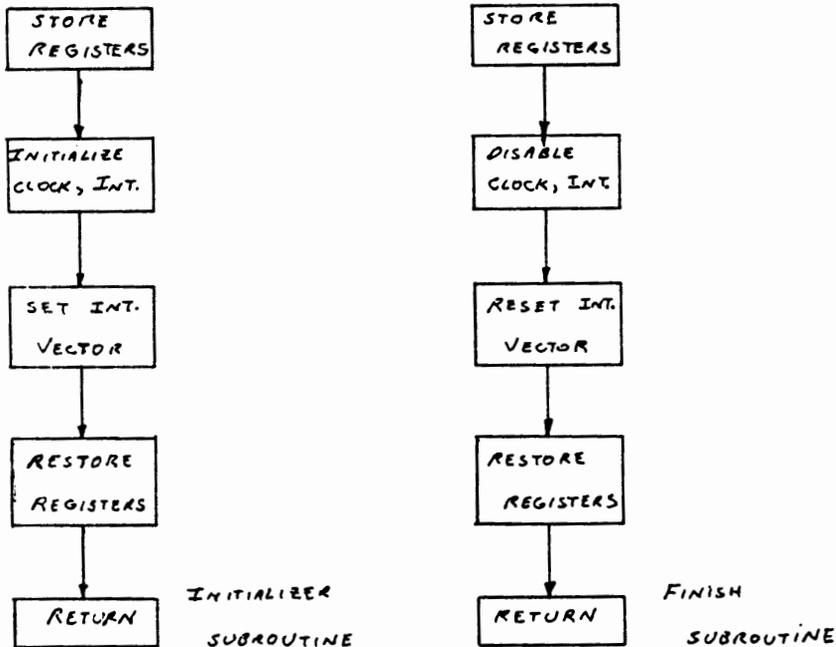
Figure 4. Flow charts detailing the Initialization and Finish machine language subroutines.
