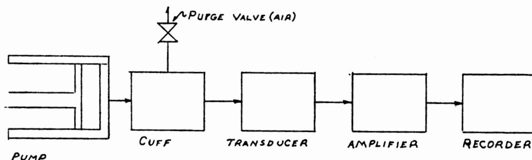
Figure 1. A block diagram of the experimental set-up used by Bhattarai, Chen, and Reynolds.
