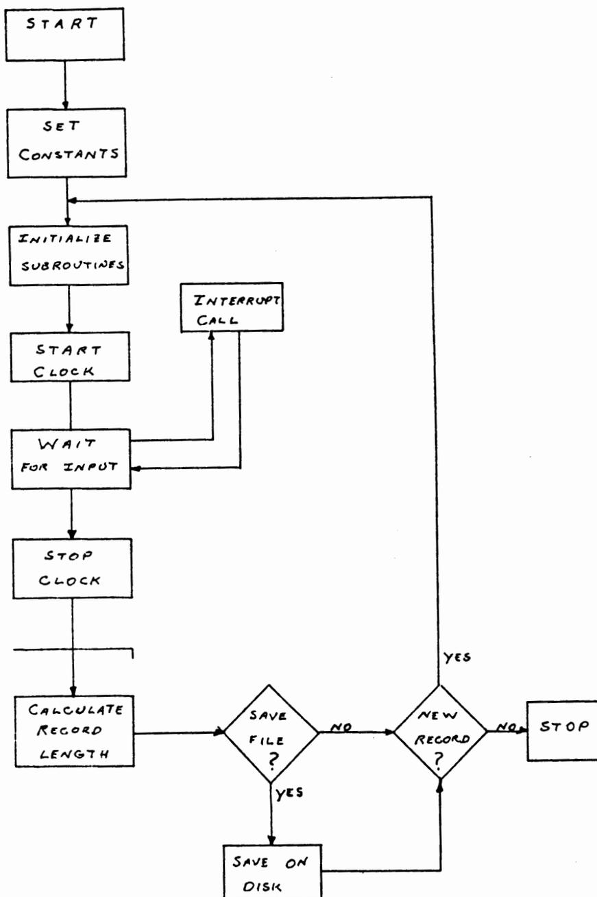
Figure 3. A flow chart for the BASIC driver program A/D. Dotted lines denote an interrupt call/
