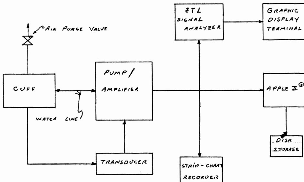
Figure 8. A block diagram of the experimental set-up used in this study.
