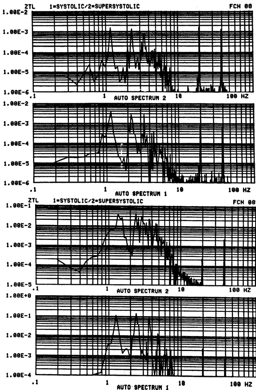
Figure 11. Comparison between hydraulic and pneumatically gathered spectra. The top two spectra are pneumatic, the bottom two hydraulic. Note the change in scale between the two spectral plots.
