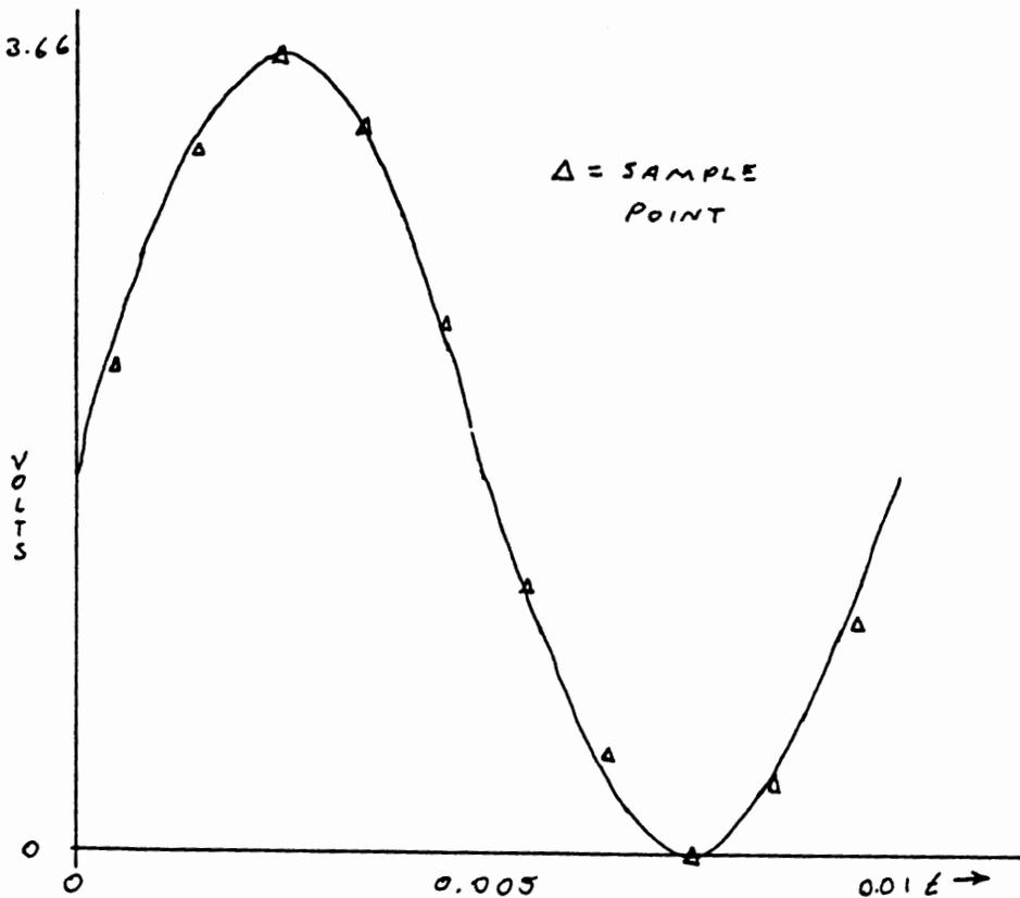
Figure 6. Digital representation plotted against the true 100 Hz sine wave. Sampling rate is 0.001 sec.
