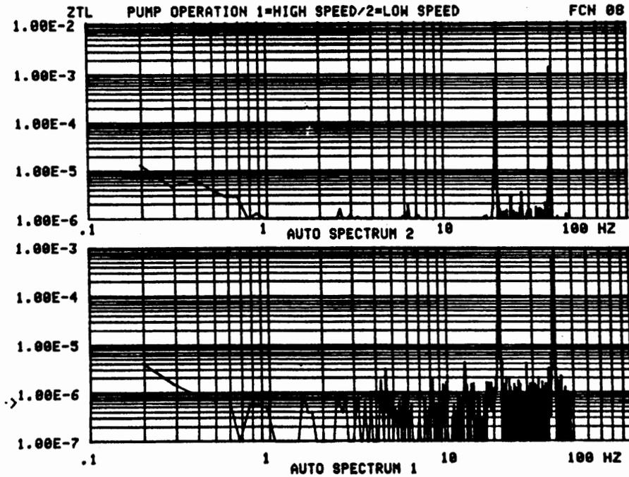
Figure 12. Noise spectra of the experimental system with atmospheric pressure at the transducer.
