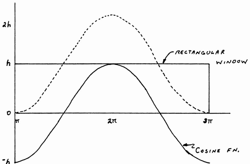
Figure 7. The Hanning window. The Hanning function is a graphical addition of the Cos function and unity.
