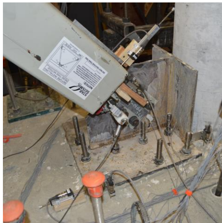
Figure 5.14 Additional instrumentation on brace-to-bent connection
