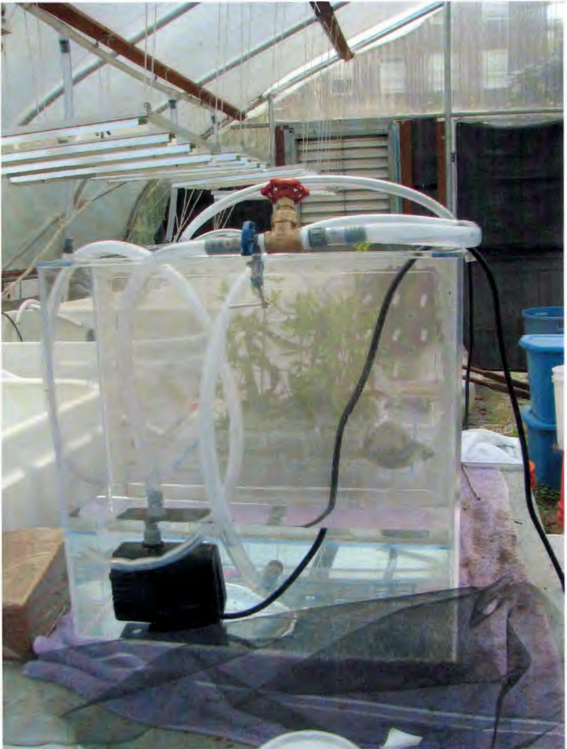
Figure 17. Horizontal velocity control; water is run from submersible pump through gate valve (top) and then through fitting in lower wall plate into the rest of the apparatus. (Photo courtesy of Leslie Bliss-Ketchum)
