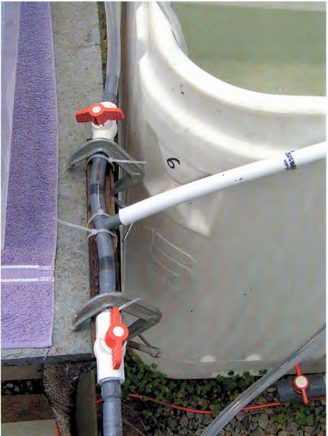
Figure 16. Vertical velocity control; ball valve at bottom diverts water back into large container while ball valve at top diverts water into experimental apparatus. Photo taken from above.
