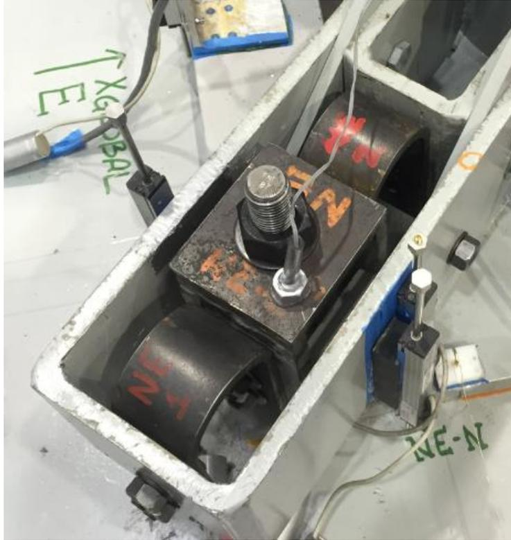
Figure 12-10: Installed Hysteretic UFP
