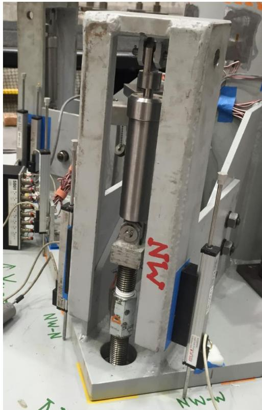
Figure 12-8: NW Viscous Damper
