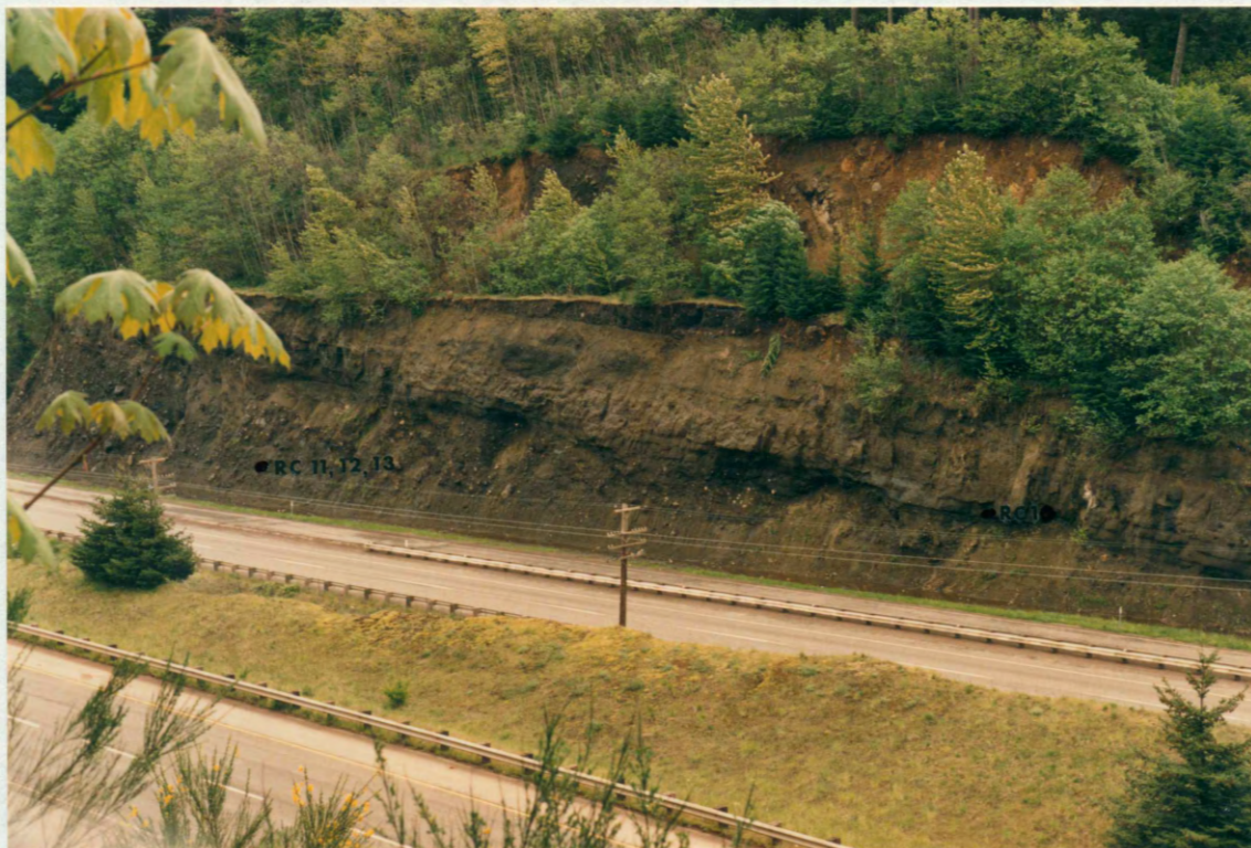
Figure 11. Sample location on east side of Eagle Creek. Large clast samples (RC 11-13) taken from unstratified lower unit which contains many petrified tree fragments and large sandstone rip-up clasts. Bedded unit is inversely graded and contains conglomerate lenses near top of cliff. Cliff above bench is part of the Ruckel Landslide.
