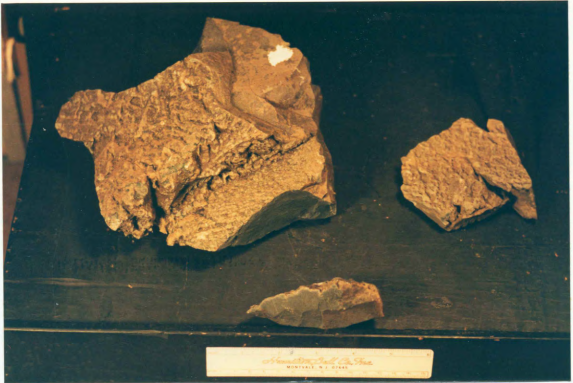
Figure 13. Samples from the confining walls zone showing the ripple-like marks along the joint traces. The two samples were collected from different locations with the Troy flow, but display similar patterns. The upper left sample has two parallel surfaces. A view parallel to the surface is seen in the center sample (a piece of the larger sample). The ruler is approximately 15 cm long.
