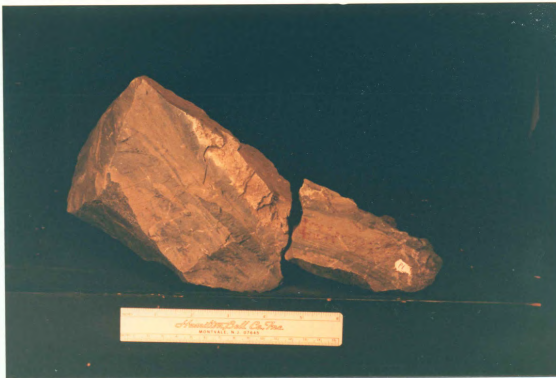
Figure 19. Two samples from the confining walls of an explosion structure showing different colored layers of basalt. These samples were collected near the contact with the overlying flow. The darker colored layers or streaks have greater proportions of glass, while the lighter basalt is more crystalline. The ruler is approximately 15 cm long.
