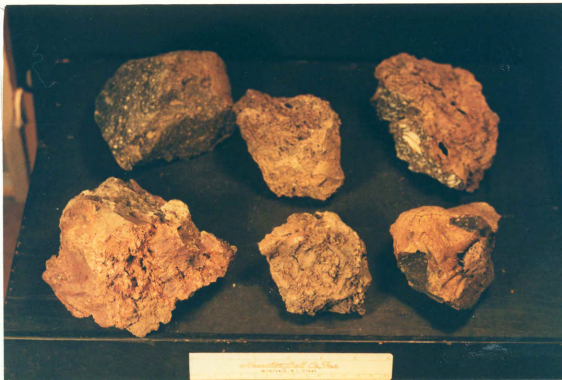
Figure 21. An assortment of three major clast types: pahoehoe clast (6), scoriaceous clasts (2,3), vesicular BVA (1), and nonvesicular BVA (4,5). Clast (4) shows intraclast cracks and fractures and clasts (5) has a rind of finely brecciated fragments. The ruler is approximately 15 cm long.
