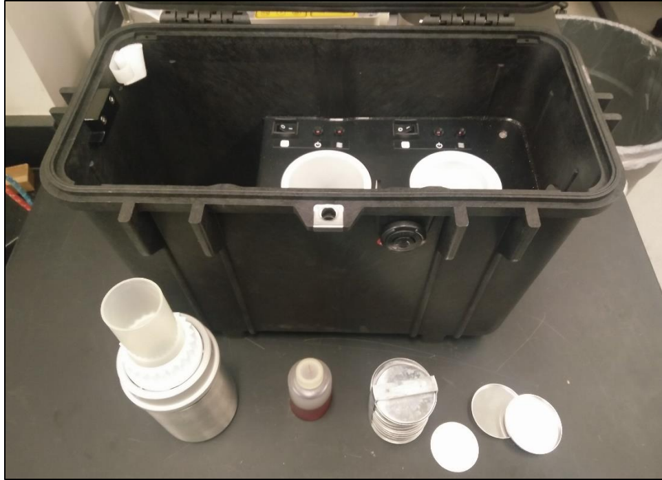
Figure 6: DelAgua water testing kit with Membrane Filtration Vacuum Chamber, MLSB growth medium, aluminum petri dishes, and sterile sample pad
