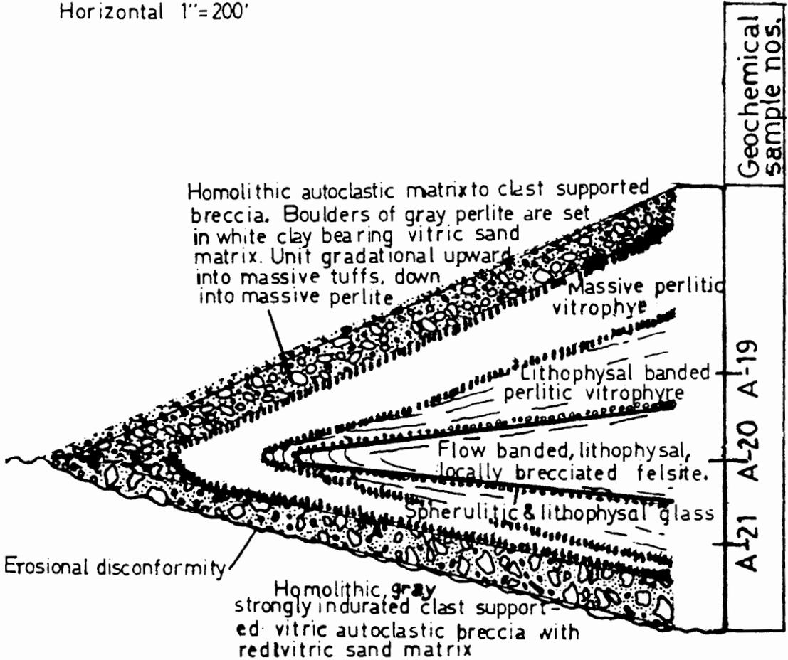
Figure 10. Measured cross section of a lateral rhyolite flow margin in section 18, T12S R40E.
