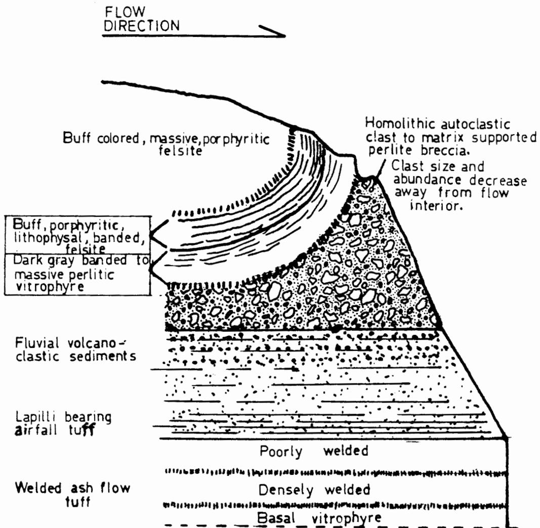
Figure 9. Cross section of a terminal margin of a block lava flow on the east side of Glassgow Creek in section 16, T12S R40E.
