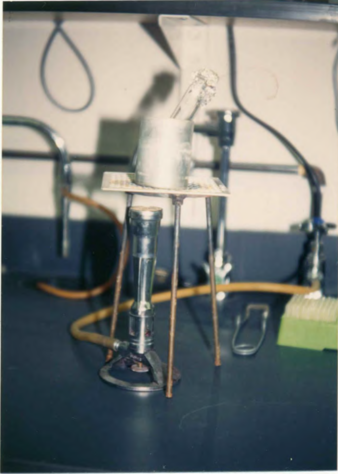
Figure 2. Double boiler set-up for agarose gels.
