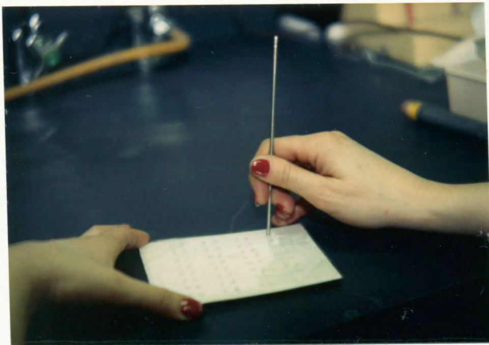
Figure 3. Using gel punch to make wells in gel.
