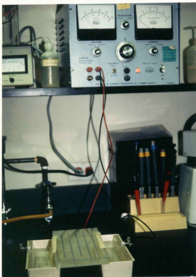
Figure 7. Gel is ready to run - complete electrophoresis set-up.
