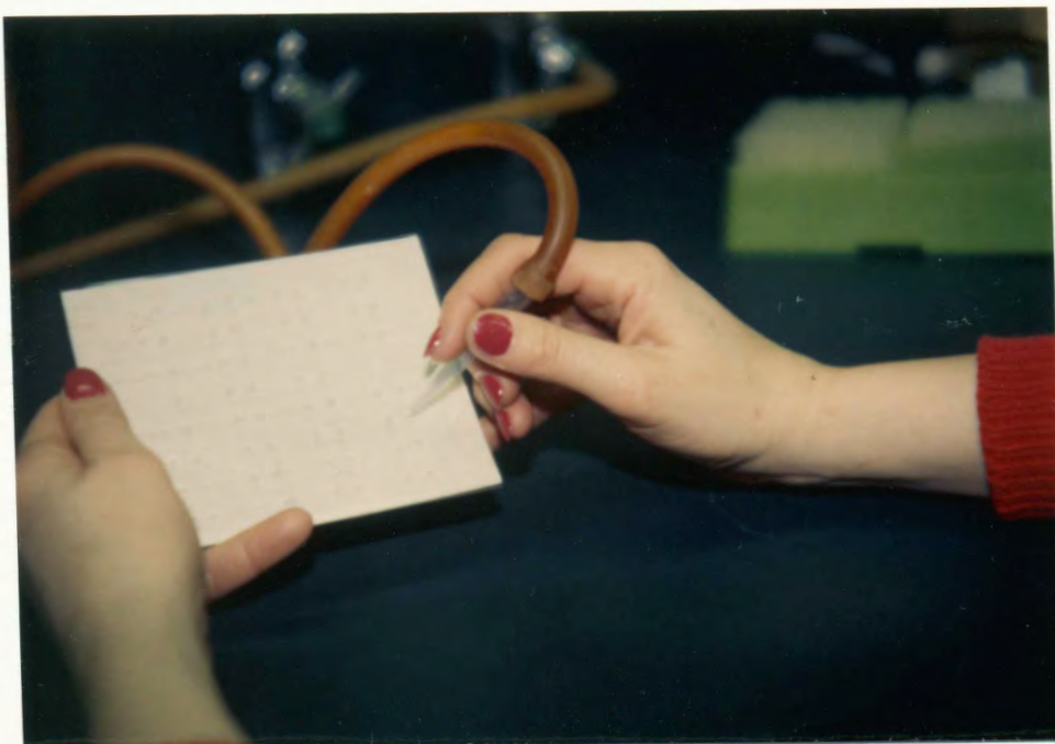
Figure 4. Using vacuum pipette to suction out plugs made in gel by gel punch.
