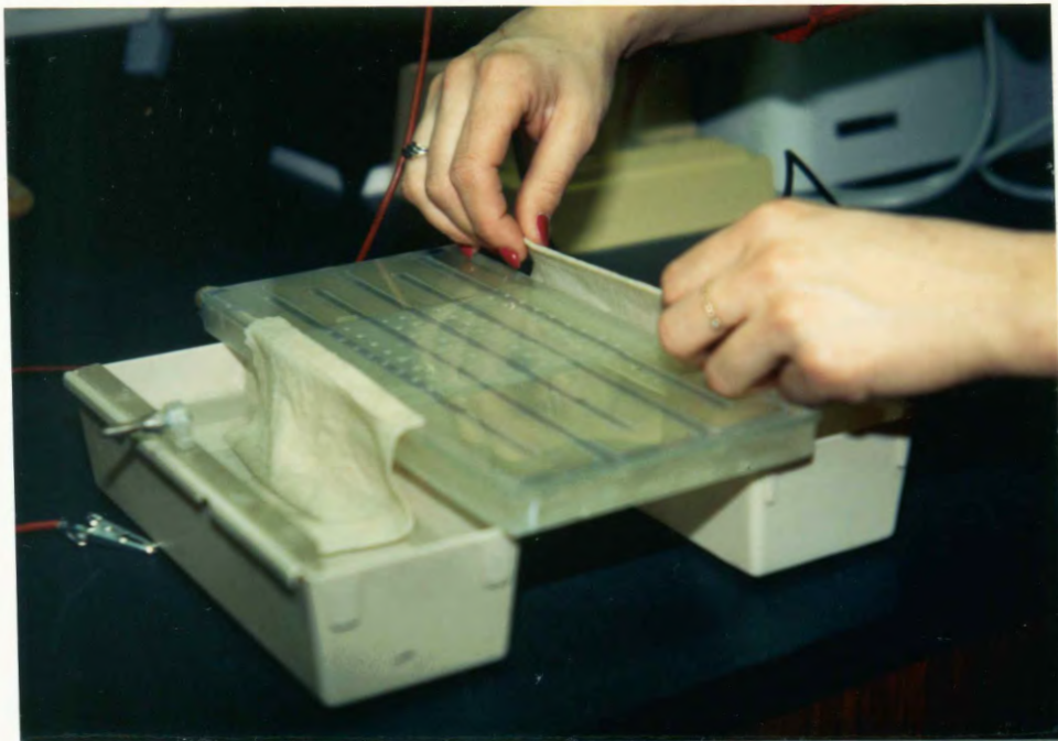
Figure 6. Placing wick material on end of gel for electrical contact.
