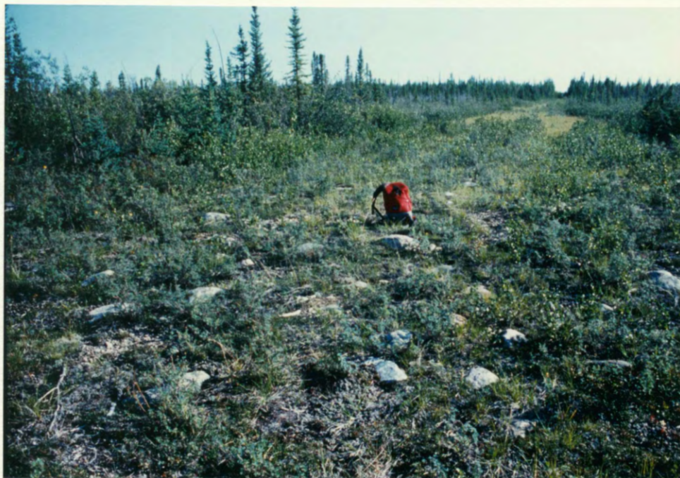
Figure 14. Unearthed rocks on a roadway underlain by coarse ground moraine (Site # 4).
