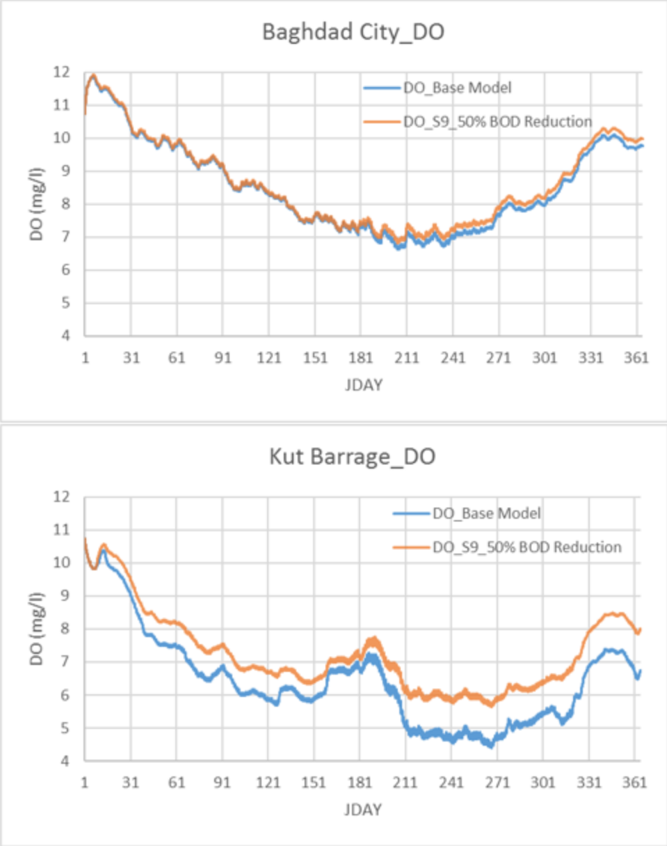
Figure 139: Model dissolved oxygen (DO) predictions for base model and management scenario 9 (50% BOD Reduction) at Baghdad City and Kut Barrage.
