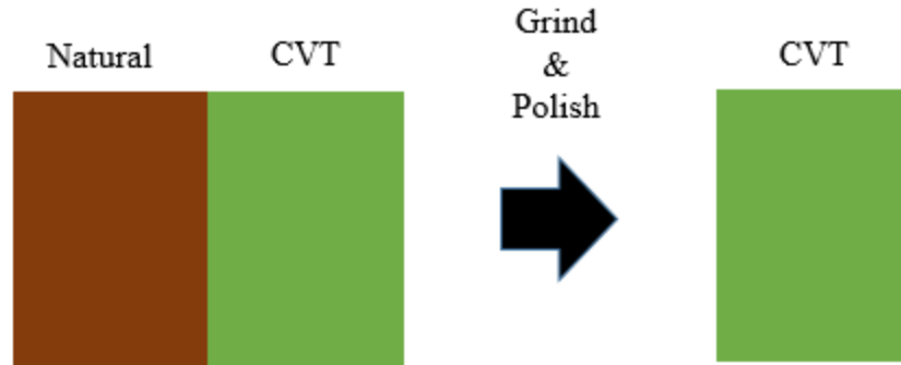
Figure 3.1. Schematic for CVT growth onto natural pyrite and then removal of natural pyrite to leave only the CVT pyrite for use in the HTSG.
