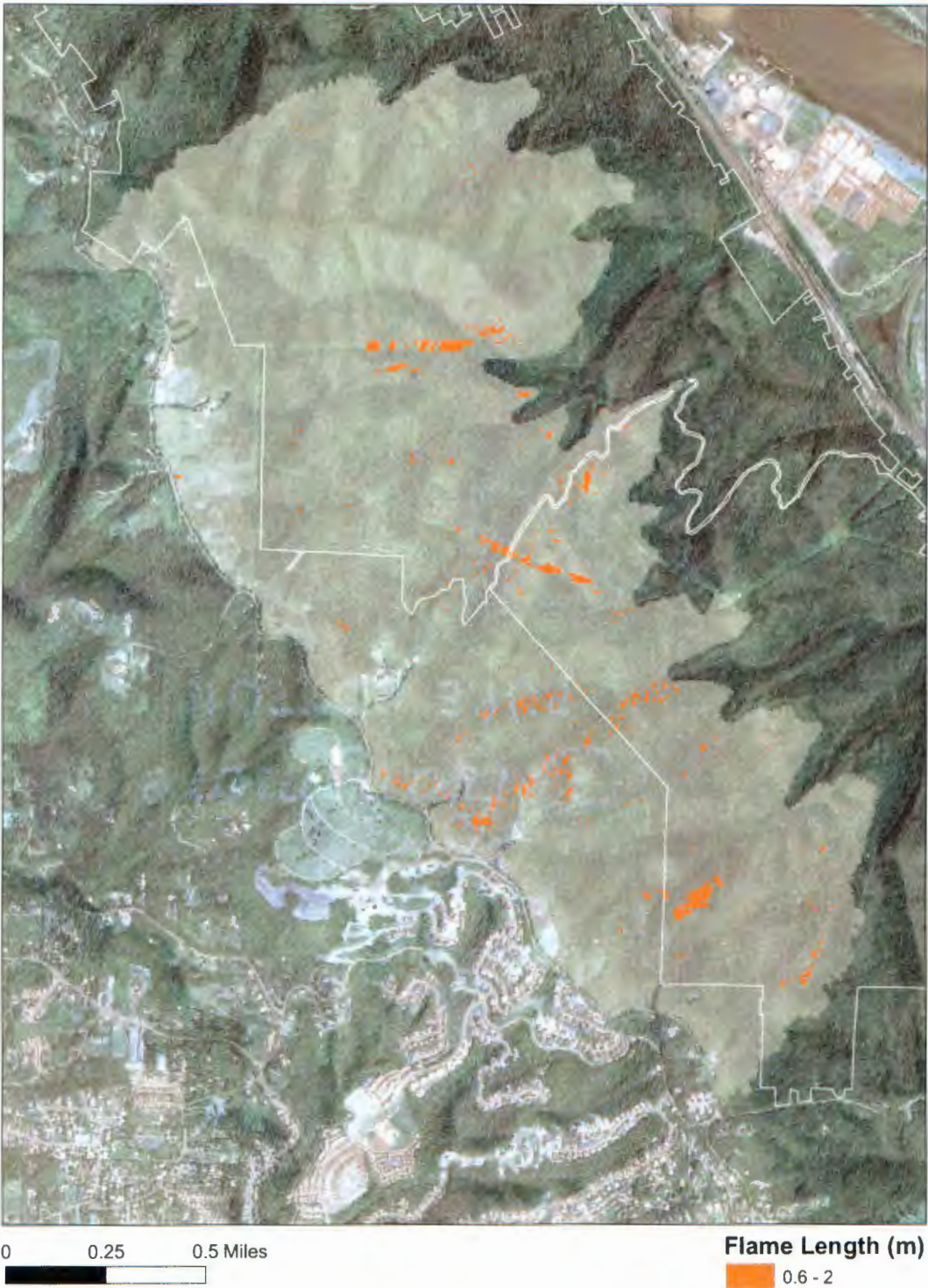
Figure 53: The flame length of the standard simulation. Most flame lengths calculated for the standard simulation represent a low risk fire. Any area not colored experienced flame lengths less than 0.6 meters. Increased flame length is observed in the utility corridors. The standard simulation exhibits increased fire behavior on the north facing slopes due to the prevailing wind direction. (Base map source: City of Portland, USGS, fire data from Author using Farsite)
