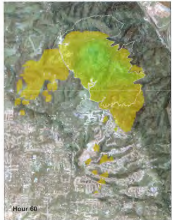
Figure 58: The images show a four hour sequence (hours 57 to 60) in the fire spread of the custom simulation. No spotting has occurred in hour 57. In hour 58 the first few spot fire have ignited and started to spread. In hours 59 and 60 the spot fires continue to grow and some of them backfire into the main fire. (Base map source: City of Portland, USGS, fire data from Author using Farsite)
