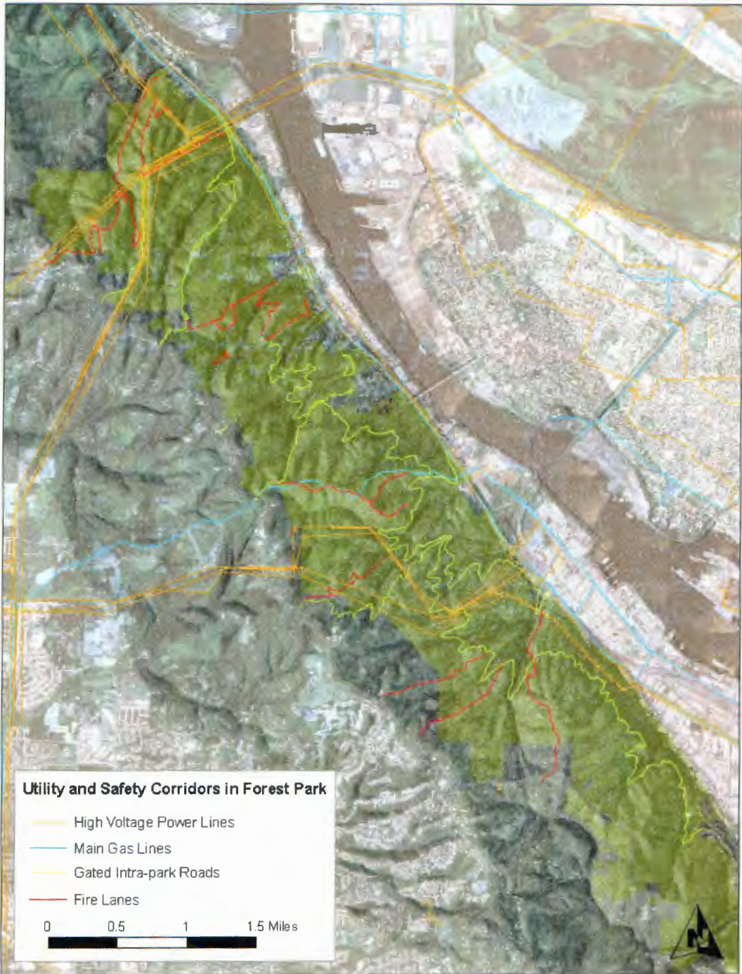
Figure 22: Two utility corridors transect the park, one at the extreme northern end of the park and the other in the central management unit, which includes a subterranean gas line. Wood is naturally a poor conductor of electricity, except at extremely high voltages. The utility owners clear many of the trees and branches from the area under the power lines. However, during hot summer days lines sag and in windy conditions trees can blow into or fall across power lines and creating potential for arcing and fire. After larger fires occurred in the park, firelanes and roads were improved to support firefighting efforts within the park. (Source: City of Portland, Metro RLIS, Friends of Forest Park)
