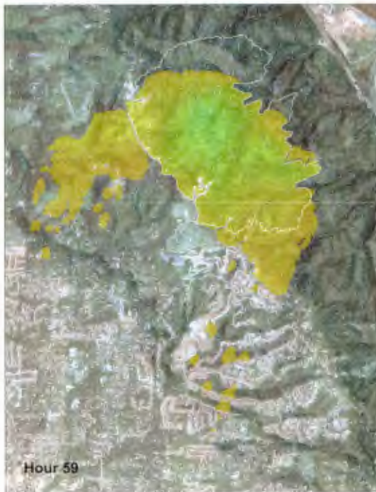
Figure 58: The images show a four hour sequence (hours 57 to 60) in the fire spread of the custom simulation. No spotting has occurred in hour 57. In hour 58 the first few spot fire have ignited and started to spread. In hours 59 and 60 the spot fires continue to grow and some of them backfire into the main fire. (Base map source: City of Portland, USGS, fire data from Author using Farsite)
