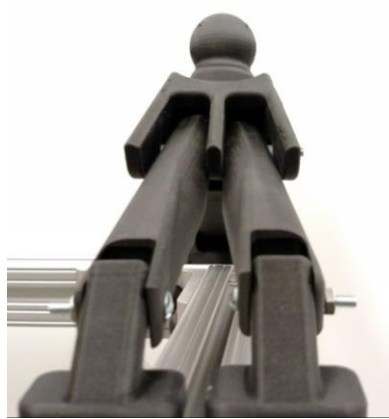
Figure 58 - Anterior view of the 3D printed version 1 foot showing the two toes
