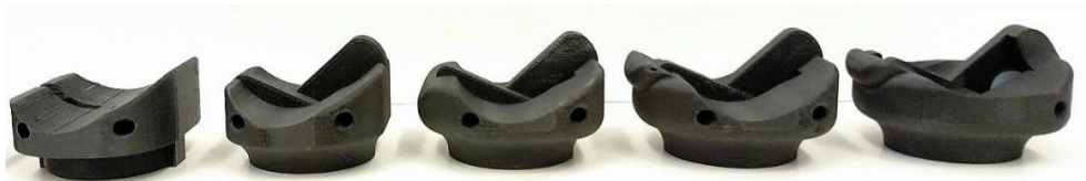
Figure 49 - Tibial head changes as the prototype testing progressed
