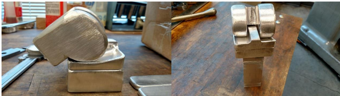
Figure 26 - Initial completion of the knee joint prior to welding
