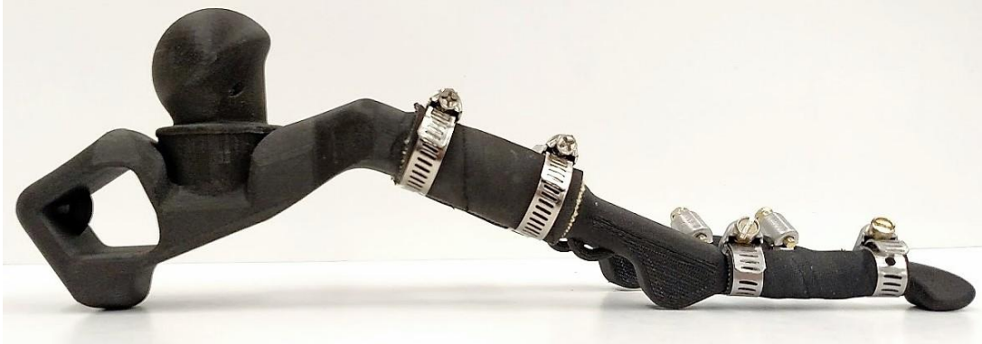
Figure 59 - Foot design version 2 seen laterally after the assembly using the pneumatic actuators as synovial joints
