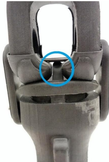
Figure 44 - Second version of the 3D printed knee showing locking mechanism (circled)
