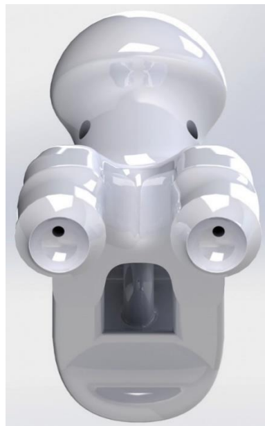
Figure 36 - By combining the talus and calcaneus, the pneumatic spring element used for the arch is now protected.
