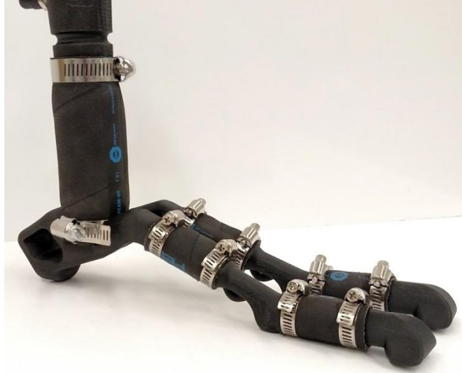
Figure 61 - 3D Printed foot version 2 with the pneumatic actuator sleeve for the ankle added
