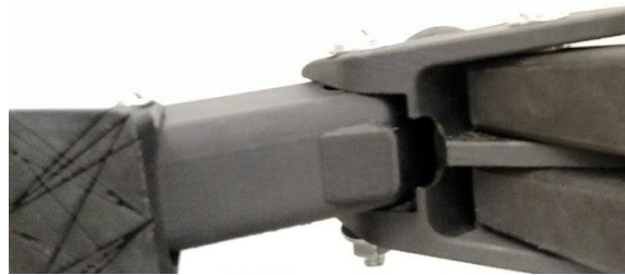
Figure 57 - Distal view of version 1 of the 3D printed foot showing the lever arm addition on the calcaneus
