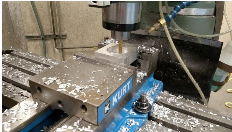
Figure 25 - Aluminum slug being machined for the tibial end using a 2-axis CNC machine.
