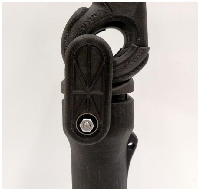
Figure 41 - Fully assembled second version of the knee joint with the cylinder inflated.
