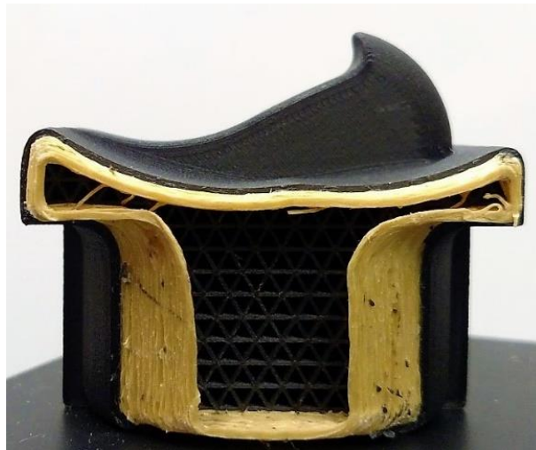
Figure 10 - Cutaway of a 3D printed part showing the continuous Kevlar fiber inlay (yellow) inside the nylon and chopped carbon fiber composite (black)
