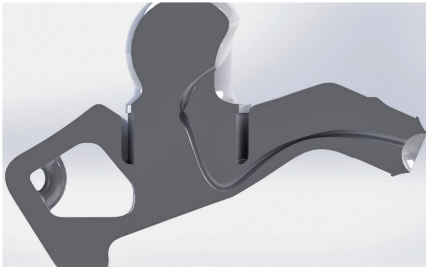
Figure 60 – Section view of the talus in SolidWorks showing the tube inside the model that lets air flow down into the other joints of the foot
