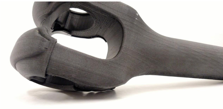
Figure 43 - 3D printed femoral end with the clips inlaid with Kevlar added back into the femoral end
