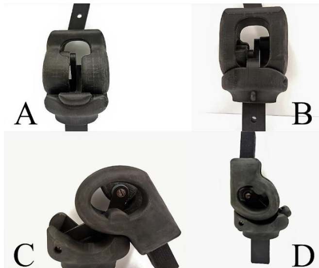
Figure 51 - Constructed joint (A) rear view, (B) front view, (C) full flexion, and (D) full extension
