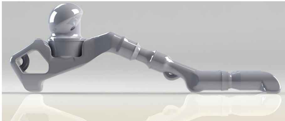
Figure 35 – 3D model of version 2 of the foot as seen laterally (and without the pneumatic sleeve, that attaches the joints).
