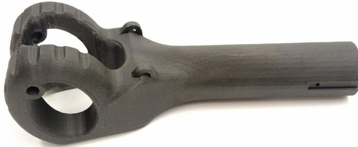
Figure 42 - 3D printed femoral end with the clips removed from the end
