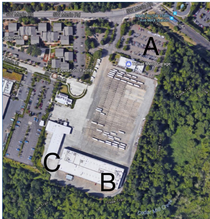
Figure 4. Stormwater sample collection locations on the TriMet Merlo property in Beaverton, OR: the employee/visitor parking lot (A); the bus throughway from the washing station to the property exit (B); and immediately after the bus washing station (C).
