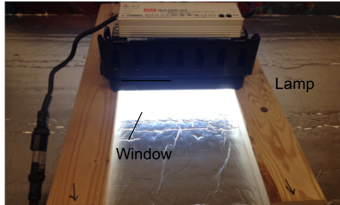
Figure B.4 LED lamp positioned above the window cut into the freezer lid.
