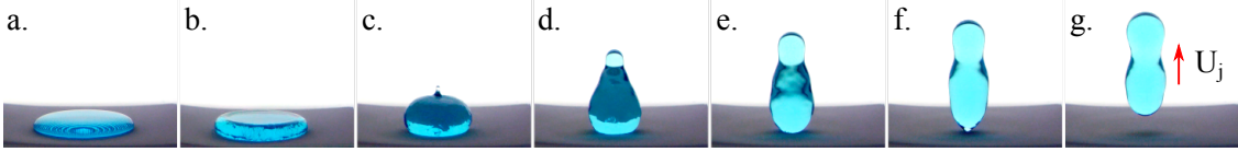
Figure 1: Time sequence (20 Hz) of a 5 mL dyed water puddle jump from a textured PTFE coated hydrophobic substrate with \theta = 150^\circ following the step reduction in gravity during a simple drop tower test. Sequence of images demonstrate the following: a. static 1-g interface, b. inward radial capillary wave formation, c. geyser formation and generation of satellite drop ejections, d.-f. large amplitude deflections, and g. drop detachment at steady velocity U_j .
