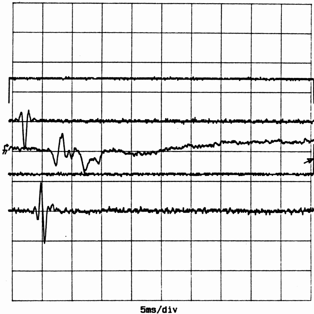
Figure 4. Similar to the previous figure (Figure 4), the trigger (top trace) causes the computer to generate a click, here, the AP electrical signal (second trace). The ABR waveform morphology (third trace) is different then that of the WGI ABR morphology. The fourth trace represents the validation signal. The last trace is the microphone signal.
