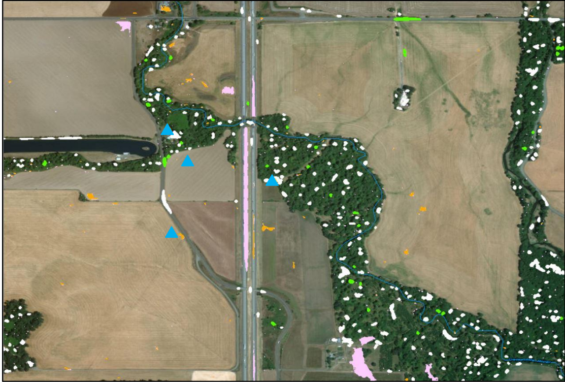
Figure 13. Elevation extraction (white) polygons versus slope (green) and area (orange) extraction, as well as sink identification (pink) shown for comparison. Blue triangles indicate the location of a previously identified mound.
