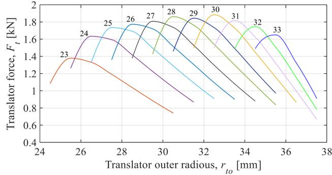
Fig. 2-23. Translation force as a function of translator outer radius,  $r_{to}$  and inner rotor outer radius  $r_{io}$  for iteration V
