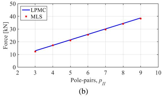
Fig. 4-27. Case 2: calculated force of LPMC and MLS a) using FEA and b) using analytical model
