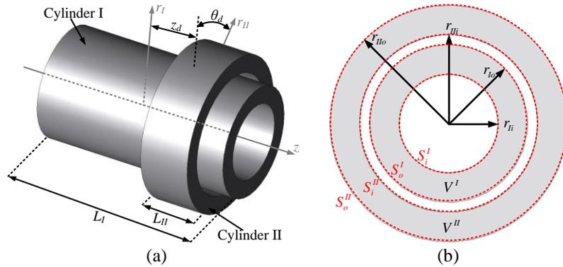
Fig. 4-22. Magnetic lead screw, a) axial parameters, and b) cross sectional parameters
