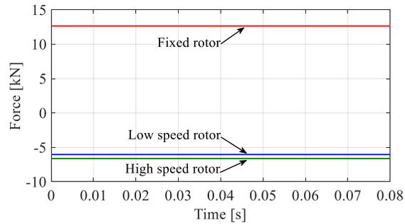
Fig. 3-17. Axial force characteristics of the AFMG for the case when both rotors were rotated with practical design considerations.
