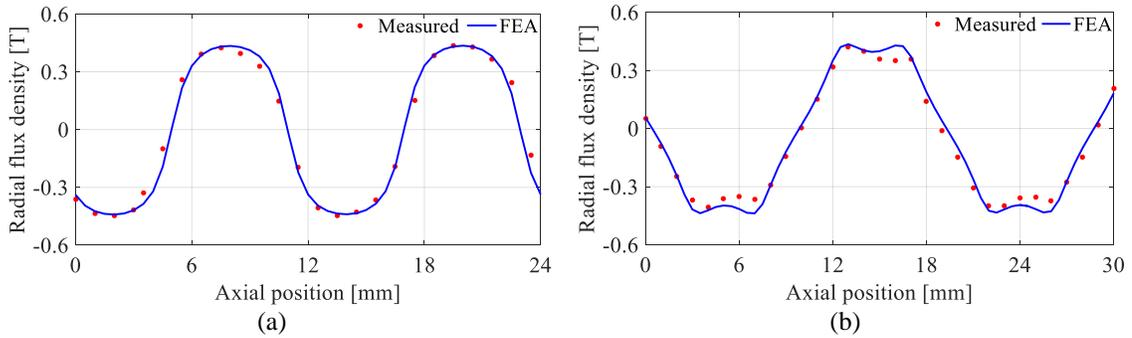
Fig. 2-31. Radial flux density along z-axis at radial distance of 0.85 mm from the surface of the a) inner rotor and b) outer cylinder
