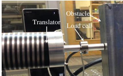
Fig. 2-32. Translator force measurement using a load cell when it was pushing against an obstacle.
