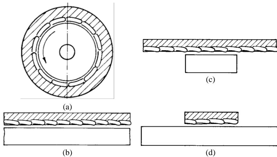
Fig. 1-7. Construction of linear motor's geometry; a) conventional motor, b) unrolled conventional motor, c) long stator motor, and d) short stator motor [20].
