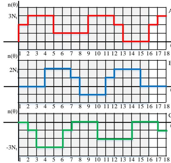
Fig. 3-31. Turns function of the three phases over the first four poles.
