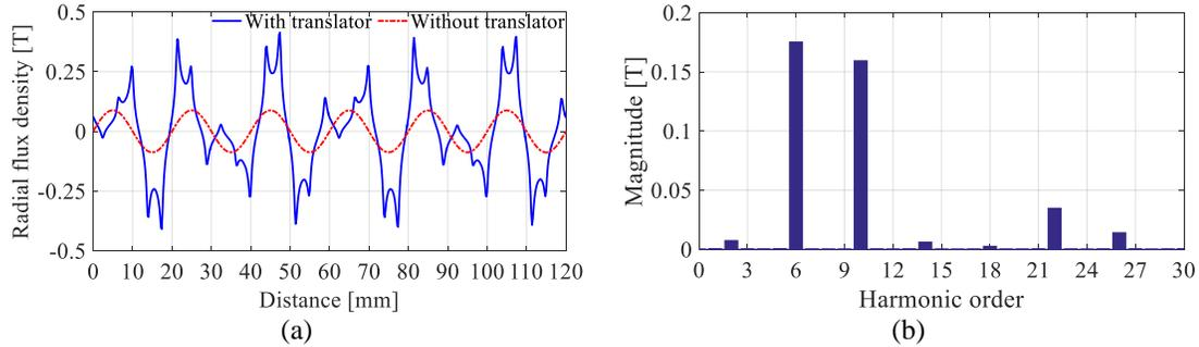
Fig. 2-41. a) Radial flux density in the inner airgap ( $r=26.25$  mm) when only outer cylinder magnets. b) Harmonic content with translator presents
