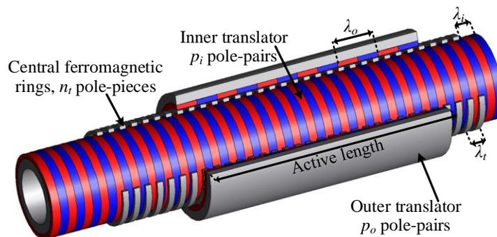
Fig. 1-19. A LMG with  $p_i=15$ ,  $p_o=6$  pole pairs and  $n_t = 21$  central ferromagnetic rings.
