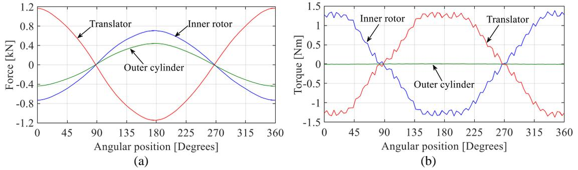
Fig. 2-27. a) Force, and b) torque on different parts of the MGLS due to rotation of the inner rotor
