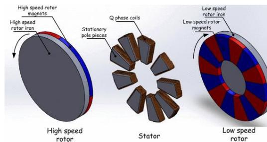
Fig. 3-7. Exploded view of the axial flux magnetically geared machine proposed by Zaytoon *et al.* [72]
