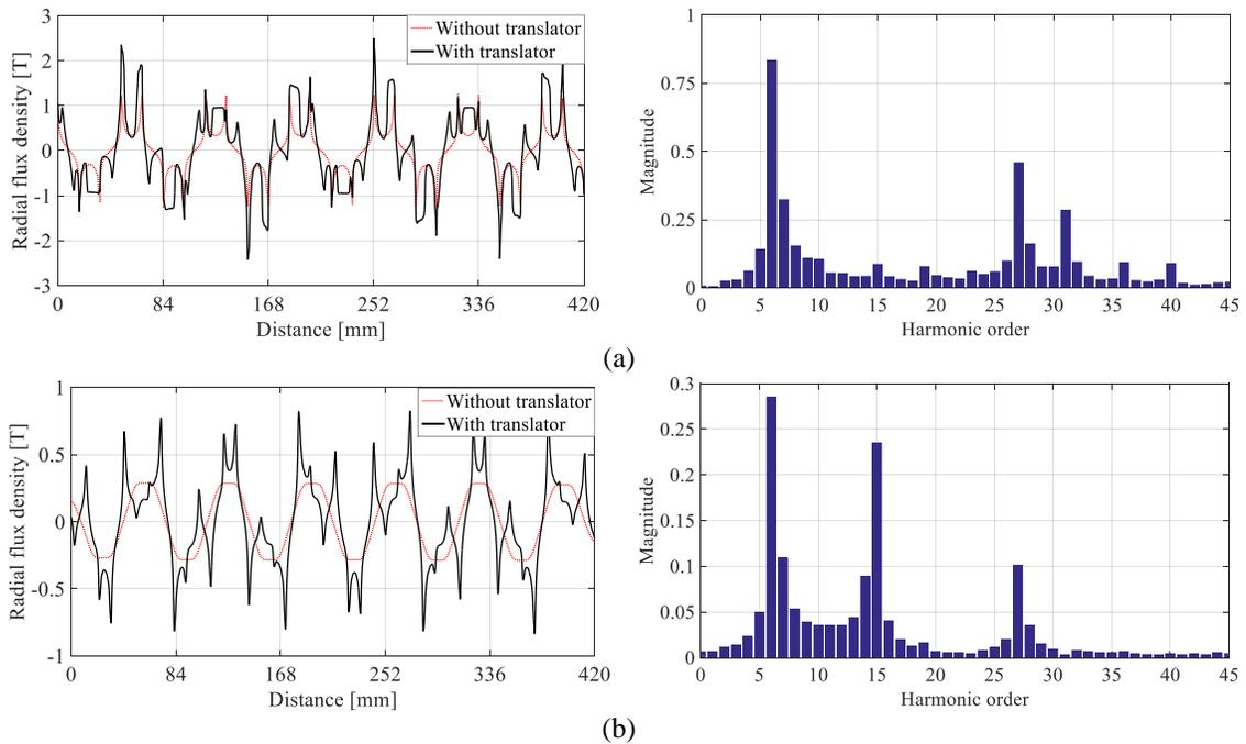
Fig. 2-16. Radial flux densities and related spectrums a) adjacent to outer rotor due to outer rotor (at  $r=54.9$  mm), b) adjacent to inner rotor due to outer rotor (at  $r=48.1$  mm)
