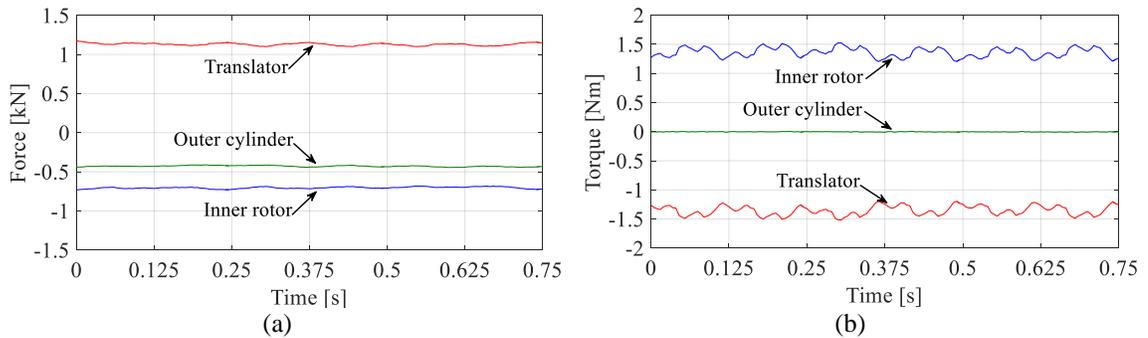
Fig. 2-28. a) Force, and b) torque on different parts of the MGLS due to rotation of the inner rotor and translation of the translator at the same time
