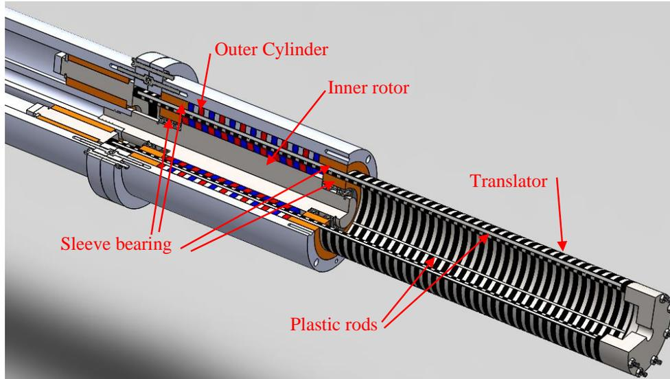
Fig. 2-49. 3D cut view of the MGLS showing the plastic rods and sleeve bearings
