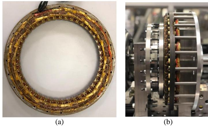
Fig. 3-40. The experimentally assembled stator a) lamination with winding, b) mounted on the AFMG.
