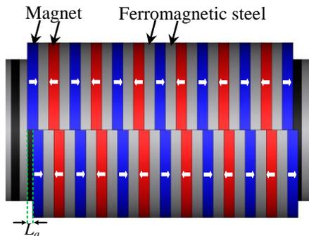
Fig. 2-37. Parametric design to investigate the effect of the axial shift,  $L_a$ , between the top and bottom set of half rings
