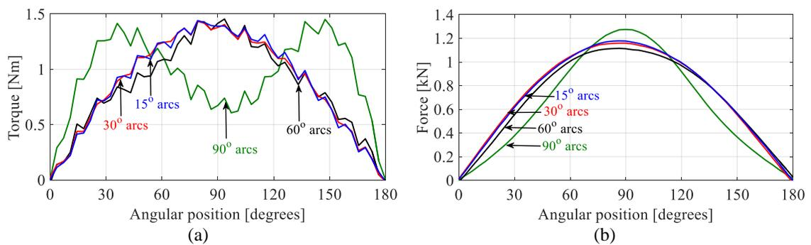
Fig. 2-25. a) Torque, and b) force when the inner rotor was rotated by 180 degrees for various designs with different inner rotor magnet arc length
