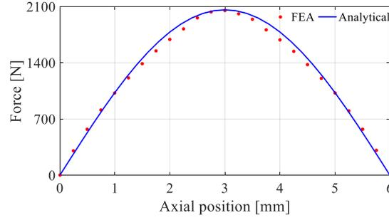
Fig. 4-9. FEA and analytically calculated force
