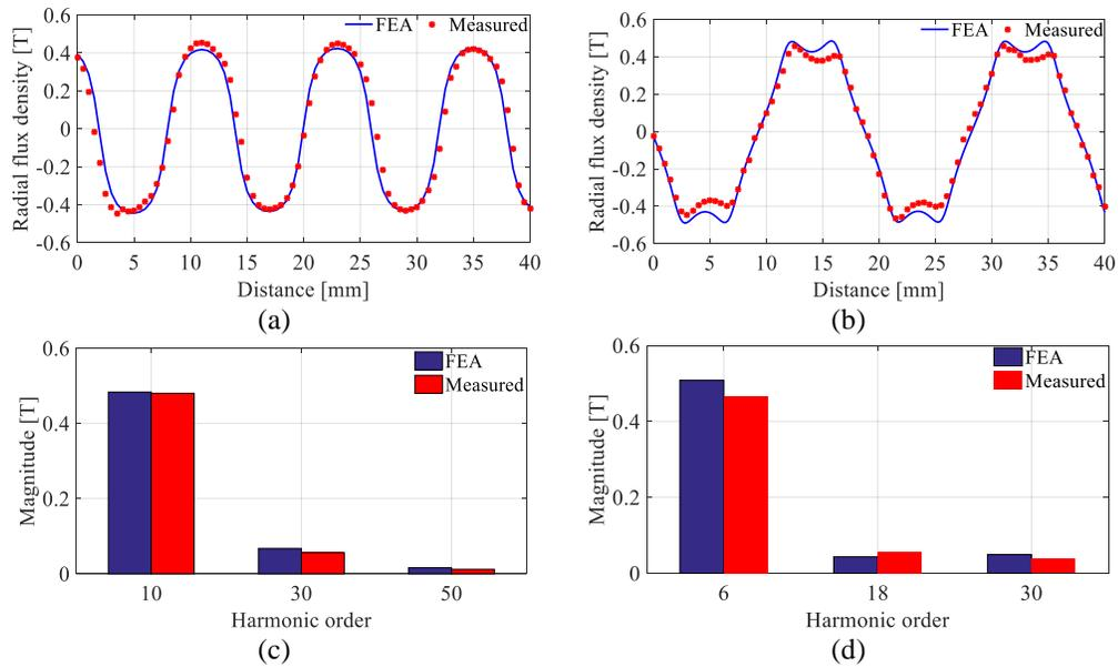
Fig. 2-45. Calculated and measured flux density and the corresponding main harmonics at 0.85 mm above the surface of (a) inner rotor and (b) outer cylinder when they are surrounded by air. The corresponding harmonics for the inner rotor and (fixed) outer cylinder are compared in (c) and (d) respectively.
