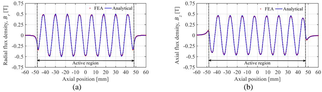
Fig. 4-24. FEA and analytically calculated flux density a) radial b) axial
