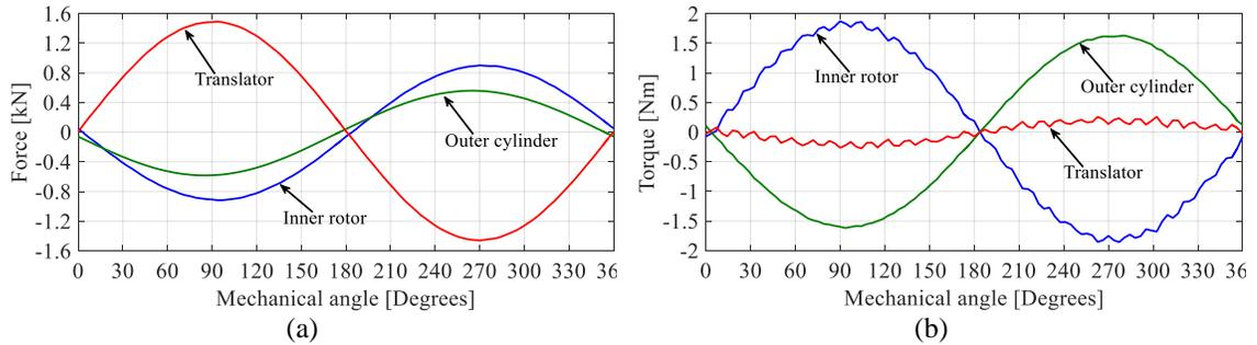
Fig. 2-42. a) Force and b) torque on each MGLS part as a function of inner rotor phase angle.
