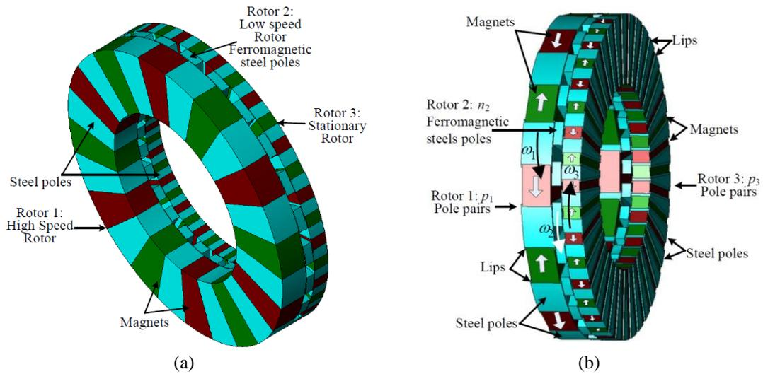
Fig. 3-9. An axial flux magnetic gear with a flux-focusing typology proposed by Acharya *et al.* [76], [77]. a) Optimized design, b) assembly design with rectangular magnets and steel poles' lips.  $p_1=6$   $n_2=25$  and  $p_3=19$ .
