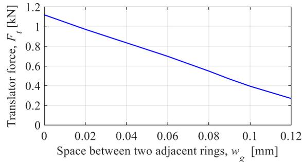
Fig. 2-35. Variation of the translator force as a function of space between two adjacent rings
