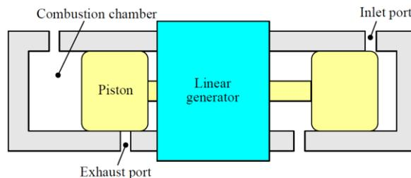
Fig. 1-21. Schematic of a free-piston generator [45]
