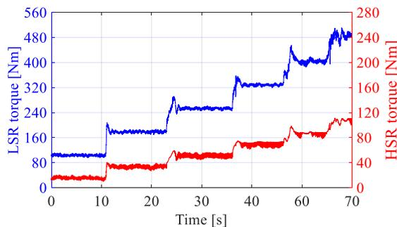
Fig. 3-22. Measured torque on high speed and low speed rotors.
