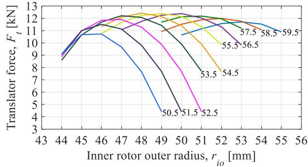
Fig. 2-14. Translation force as a function of inner rotor outer radius,  $r_{io}$  and translator outer radius  $r_{to}$  for iteration V. The curves for different  $r_{to}$  are shown on the figure.
