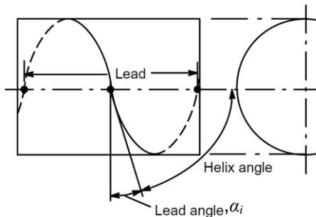
Fig. 2-36. Definition of the lead angle per ANSI/AGMA 1012-G05 [61]
