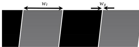
Fig. 2-34. Close up view (not to scale) of the translator pole-pieces and  $w_g = 0.1$  mm space between plastic (black) and steel rings (gray).
