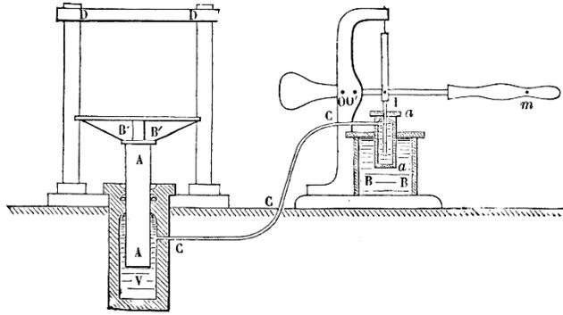
Fig. 1-3. Hydraulic Bramah Press [10]
