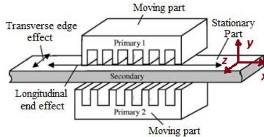
Fig. 1-8. A double sided linear induction motor topology [21]
