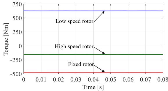
Fig. 3-16. Torque on the low speed rotor (LSR), high speed rotor (HSR) and fixed rotor for the case when both rotors were rotated with practical design considerations.
