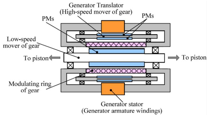
Fig. 1-22. Li's proposed magnetically geared linear generator [45]
