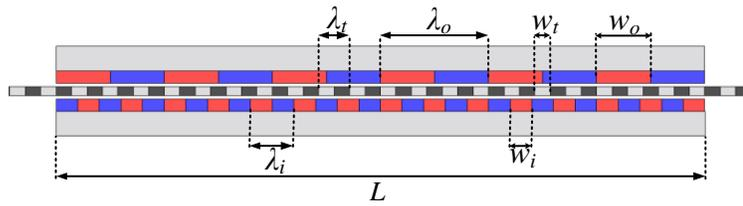
Fig. 2-2. Cut-through view of the magnetically geared lead screw showing the lead lengths for the inner, outer, and translator.
