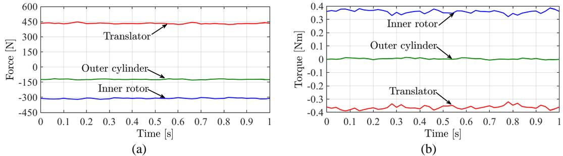
Fig. 2-10. a) Force, and b) torque on different parts of the MGLS due to rotation of the inner rotor and translation of the translator at the same time
