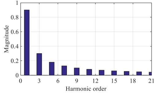
Fig. 4-3. Harmonic spectrum of the magnetization
