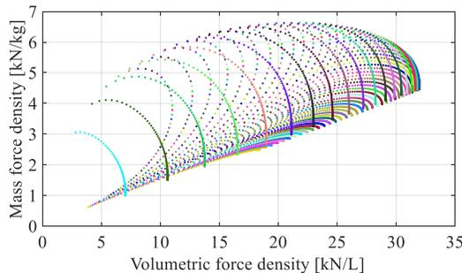
Fig. 4-12. Volumetric force density versus mass force density for different configurations within the design space, when  $r_{IIo} = 30$  mm and  $\tau_p/r_{IIo} = 0.3$ .
