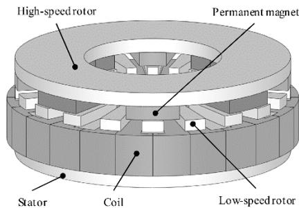
Fig. 3-5. AFMGM proposed by Niguchi *et al.* [70]
