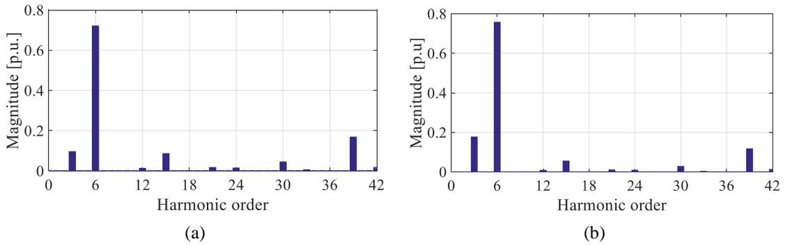
Fig. 3-37. Harmonic contents of the normalized MMF a) using FEA results b) using winding function analysis.
