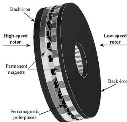
Fig. 3-1. Schematic of an AFMG [38].
