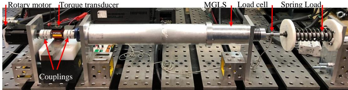
Fig. 2-47. MGLS on the test bed connected to a spring load
