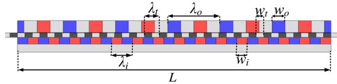
Fig. 2-12. Cut-through view of the magnetically geared lead screw showing the lead lengths for the inner outer and translator.
