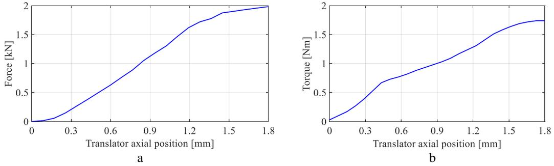
Fig. 2-51. a) Measured translator force, b) measured inner rotor torque, when translator was pushed in using a mechanical actuator.
