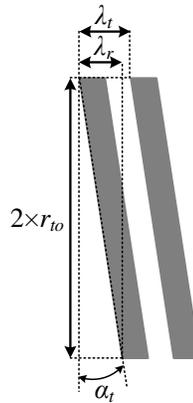
Fig. 2-4. Side view showing two consecutive skewed ferromagnetic translator rings. The definition for the translator rotor lead length  $\lambda_r$  and translator lead  $\lambda_t$  is also shown.
