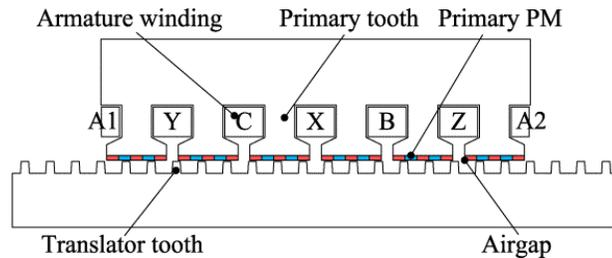
Fig. 1-14. Configuration of a linear PM Vernier motor [28].
