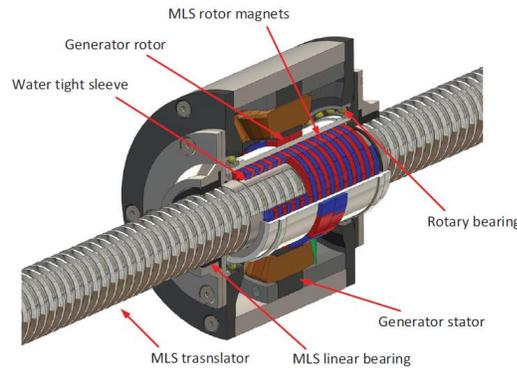
Fig. 1-31. Reluctance magnetic lead screw by Berg *et al.* [50]
