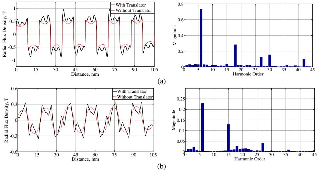
Fig. 2-8 Radial flux densities and related spectrums a) adjacent to outer rotor due to outer rotor (at  $r=19.95$  mm), b) adjacent to inner rotor due to outer rotor (at  $r=17.55$  mm)
