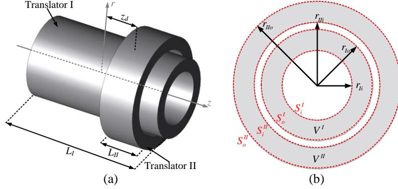
Fig. 4-6. Linear coupling, a) axial parameters, and b) cross sectional parameters
