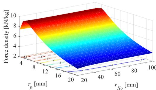
Fig. 4-16. Maximum mass force density for different values of  $r_{Ilo}$ .
