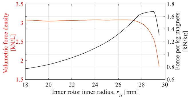
Fig. 2-22. Trade-off between maximizing volumetric force density and force-per-kg of magnet material. Results shown for iteration IV
