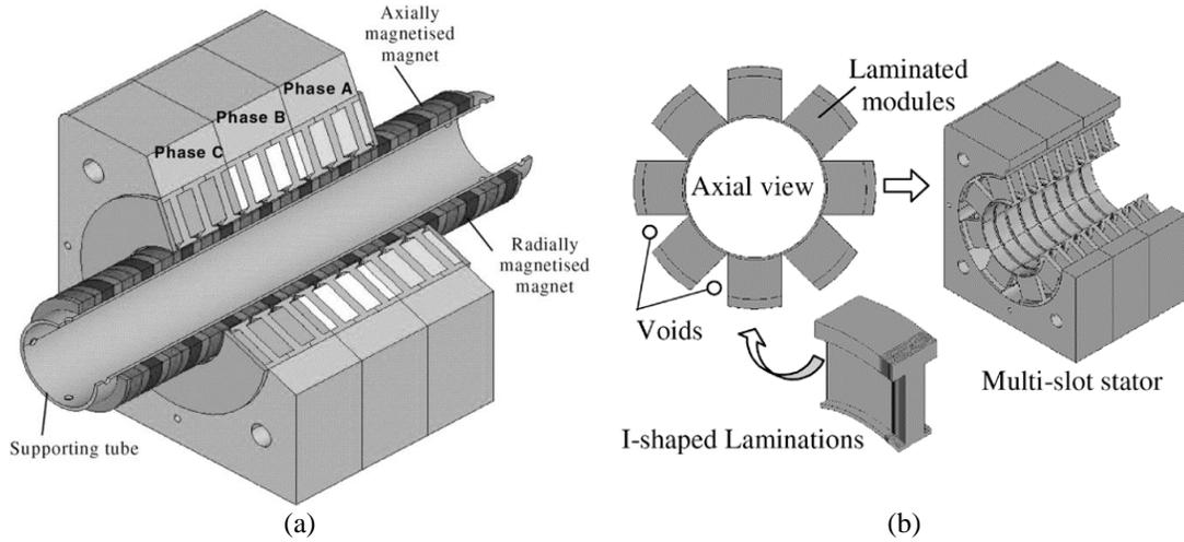
Fig. 1-12. Three-phase tubular PM machine a) structure b) Slotted stator core for prototype [26]
