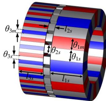
Fig. 3-10. Geometric parameters used for the axial flux magnetic gear with a flux-focusing typology [76], [77]. .
