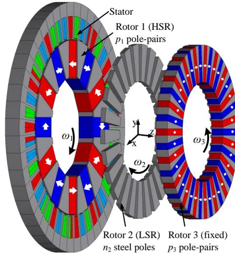
Fig. 3-27. Exploded view of the proposed AFMGM with 45 slot stator around the 6 pole-pair high speed rotor where  $p_1=6$ ,  $n_2=25$ , and  $p_3=19$ .
