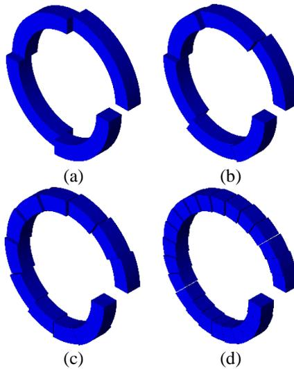
Fig. 2-24. One turn of the inner rotor helix using a) 4, b) 6, c) 12, and d) 24 magnet segments
