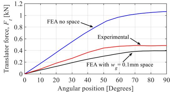
Fig. 2-33. Measured and calculated translator force with and without 0.1 mm space between rings.
