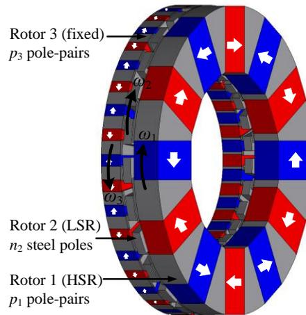
Fig. 3-11. An axial flux magnetic gear with a flux-focusing typology based on [76], [77].  $p_1 = 6$ ,  $n_2 = 25$ , and  $p_3 = 19$ .
