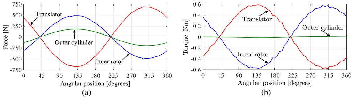
Fig. 2-9. a) Force, and b) torque on different parts of the MGLS due to rotation of the inner rotor
