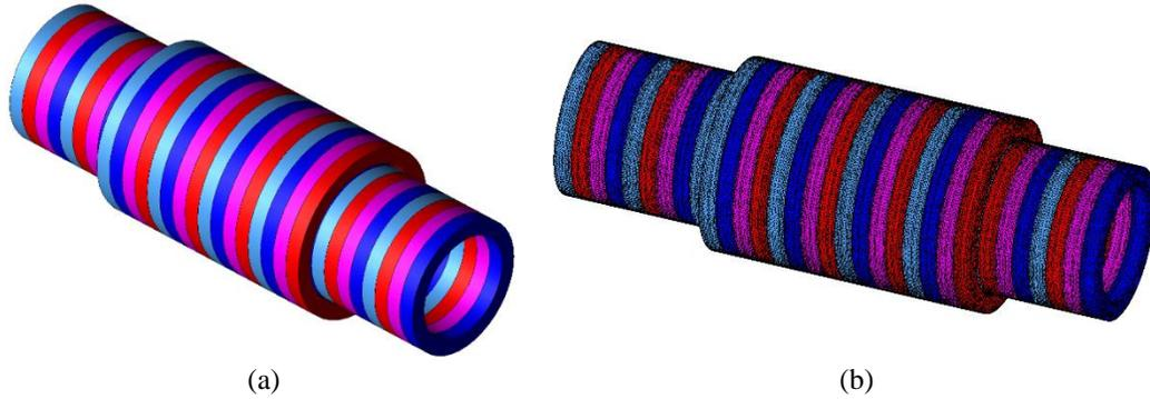
Fig. 4-7. a) 3D FEA model of a Halbach linear coupling b) the mesh.
