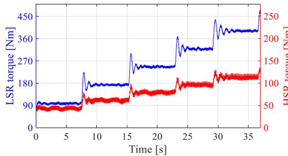
Fig. 3-46. Measured torque at HSR speed of 50 r/min at different loads.
