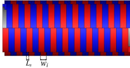
Fig. 2-26. Side view of the segmented helical inner rotor with 60° magnet arcs
