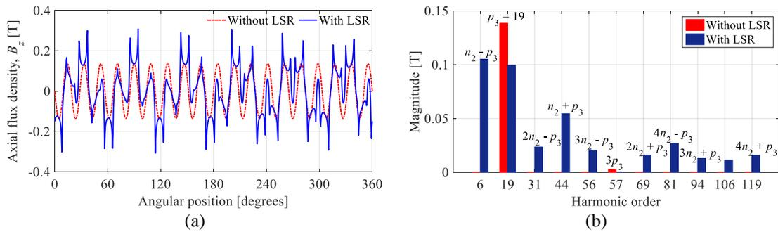
Fig. 3-14. a) Magnetic flux density near the high-speed rotor due to magnets only on the fixed rotor 3 at a radius of  $r=137$  mm and an axial distance of 0.5 mm. b) Corresponding harmonic contents.
