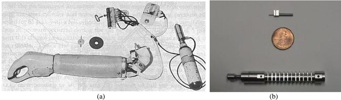
Fig. 1-1. a) Heidelberg pneumatic arm prosthesis [2], b) small hydraulic actuators with diameters of 2.3 mm and 9.6 mm for the application of prosthetic fingers [3]
