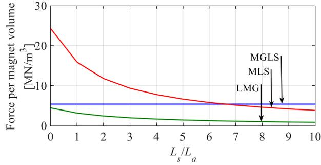
Fig. 2-21. Force per magnet volume as a function of  $L_s/L_a$
