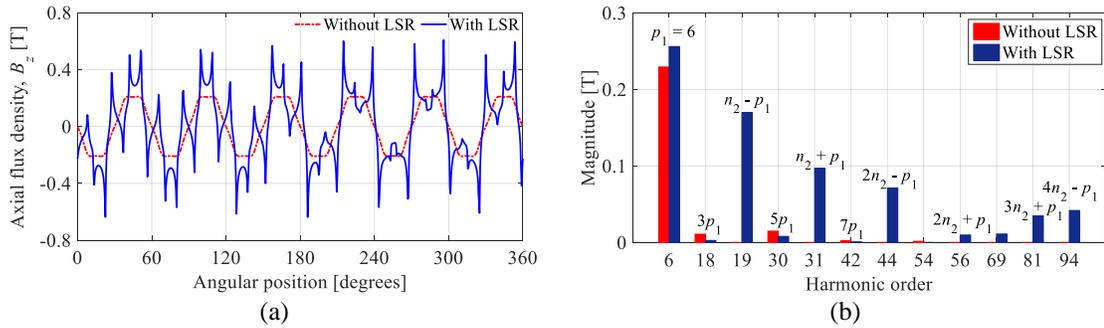
Fig. 3-13. a) Axial flux density near fixed rotor 3 due to magnets only on the high-speed rotor (rotor 1) at a radius of  $r=137$  mm and an axial distance of 0.5 mm. b) Corresponding harmonic contents.
