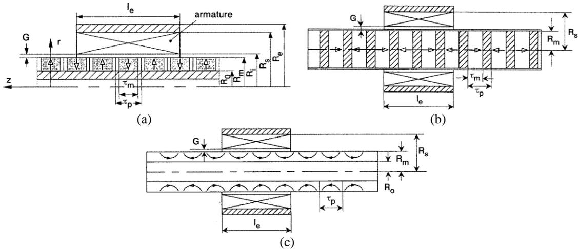
Fig. 1-11. Parametric tubular machines with a) surface mounted, b) flux focusing, and c) Halbach PM translator arrangements investigated by J. Wang *et al.* [25].
