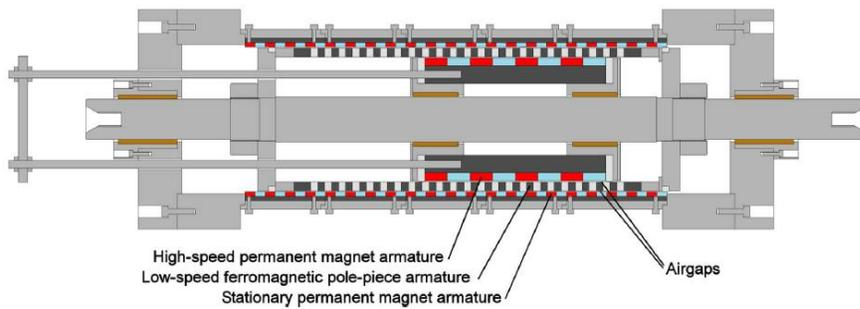
Fig. 1-23. Linear magnetic gear proposed by Holehouse *et al.* [43]
