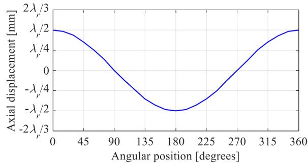
Fig. 2-6. Axial displacement of a translator ring as the function of translator angular position
