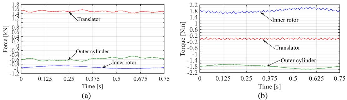
Fig. 2-43. a) Force and b) torque on each MGLS part due to rotation of the inner rotor and translation of the translator at the same time.
