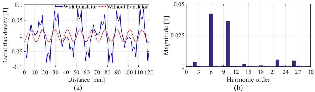
Fig. 2-40. a) Radial flux density in the outer airgap ( $r=32.75$  mm) when only inner rotor magnets present. b) Harmonic content with translator present
