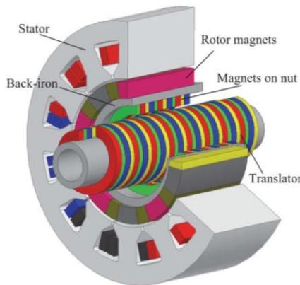
Fig. 1-30. PM machine integrated with a magnetic lead screw with Halbach pole arrangement [53].
