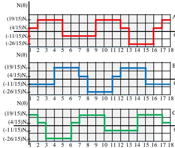
Fig. 3-32. Winding function of the three phases over the first four poles.
