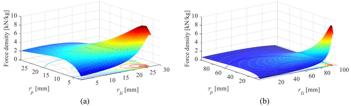
Fig. 4-15. Mass force density while geometric parameters satisfy (4.111) for a)  $r_{Ilo} = 30$  mm and b)  $r_{Ilo} = 100$ .
