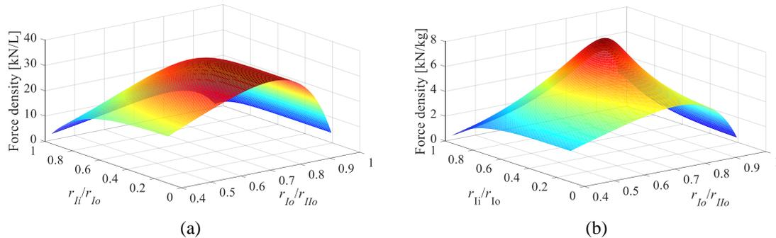
Fig. 4-11. a) Volumetric force density, and b) mass force density as a function of  $r_{ii}/r_{lo}$  and  $r_{lo}/r_{IIo}$ , when  $r_{IIo} = 30$  mm and  $\tau_p/r_{IIo} = 0.3$ .
