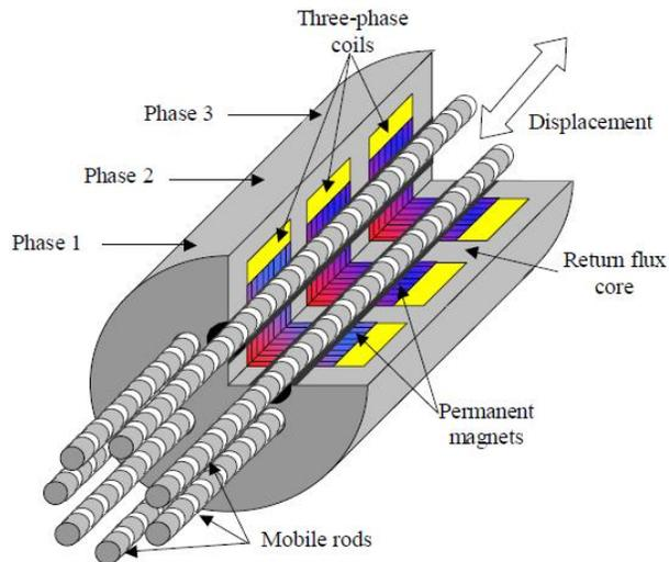
Fig. 1-17. Multi-rod linear actuator proposed by Cavarec *et al.* [17].
