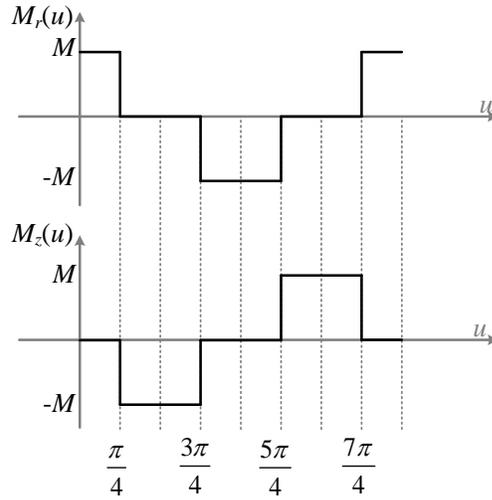
Fig. 4-19. Magnetization plots of the Halbach array
