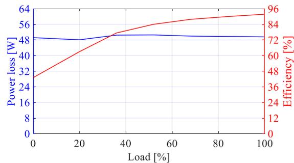
Fig. 3-24. Power loss and efficiency as a function of the load torque at 50 r/min high speed rotor speed.
