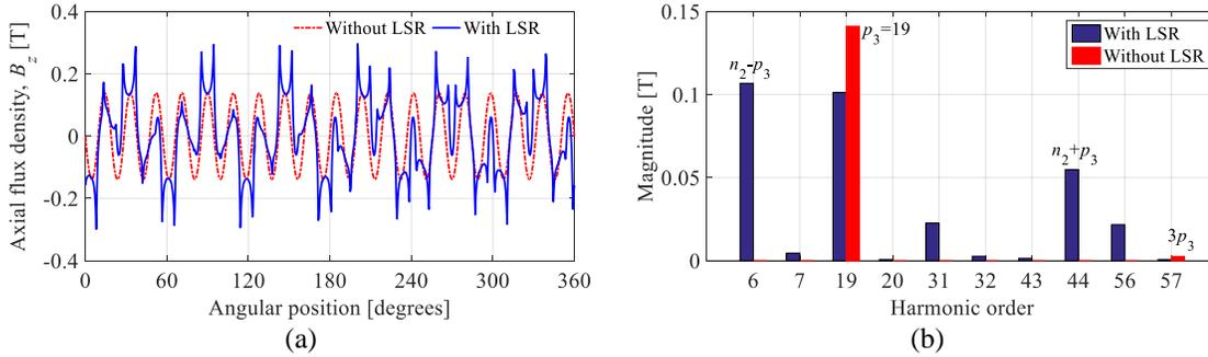
Fig. 3-35. a) Magnetic flux density near the high-speed rotor due to magnets only on the fixed rotor 3 at a radius of  $r=137$  mm and an axial distance of 0.5 mm. b) Harmonic contents of the modulated flux density.
