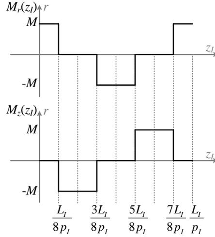
Fig. 4-2. Magnetization plots of the Halbach array
