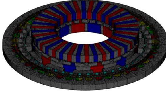
Fig. 3-33. Mesh plot for axial flux magnetically geared machine using JMAG
