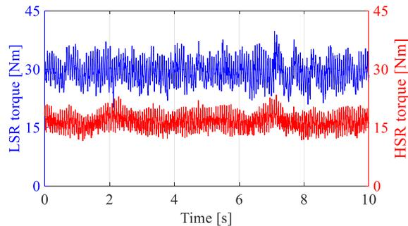
Fig. 3-23. Measured no load torque on low speed and high-speed rotors
