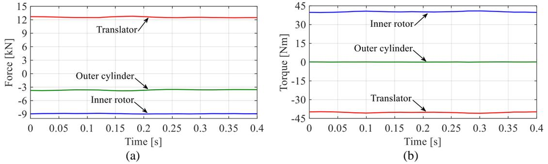
Fig. 2-20. a) Force, and b) torque on different parts of the MGLS due to rotation of the inner rotor and translation of the translator at the same time
