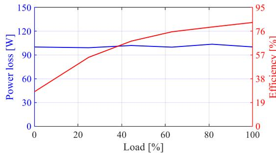
Fig. 3-47. Measured loss and efficiency as a function of load
