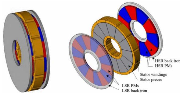
Fig. 3-8. Axial flux magnetically geared machine proposed by Khatab *et al.* [73]
