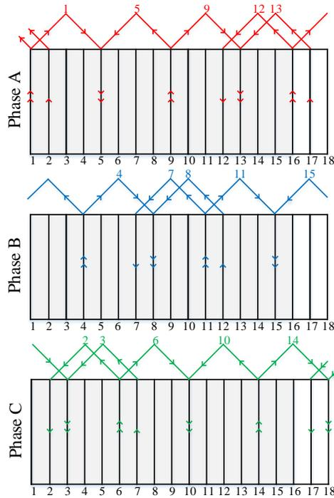
Fig. 3-30. Winding layout of the three phases over the first four poles.
