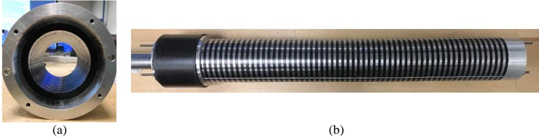
Fig. 2-44. MGLS components; a) outer cylinder, b) translator.
