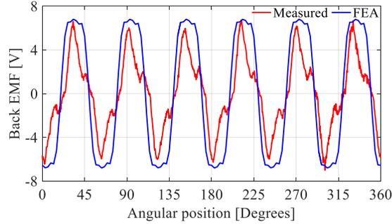
Fig. 3-42. Measured and calculated no-load three phase back-emf waveforms when the HSR is rotating at 50 r/min.
