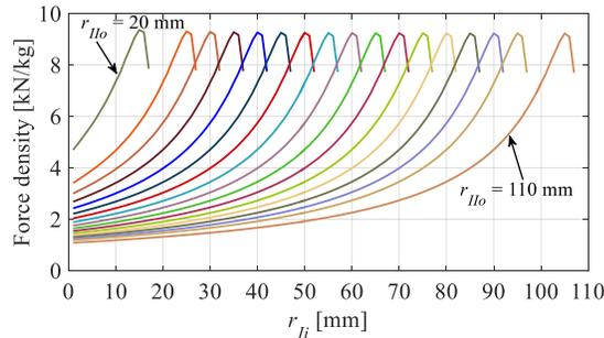
Fig. 4-17. Maximum mass force density for different values of  $r_{Ilo}$  as a function of  $r_{Ii}$ .
