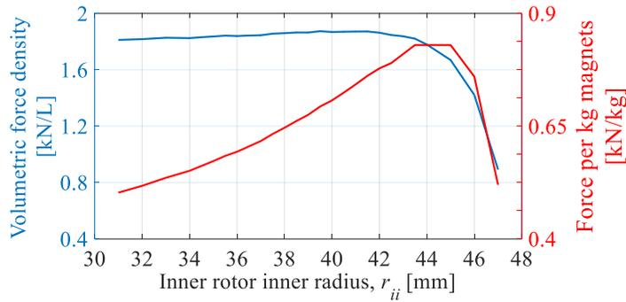
Fig. 2-15. The trade-off between maximizing volumetric force density and force-per-kg of magnet for iteration VI when  $(r_{io}, r_{to}) = (48, 54.5)$  mm.
