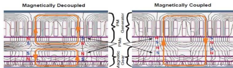
Fig. 3-3. Magnetic field distribution in coupled and decoupled designs [67]
