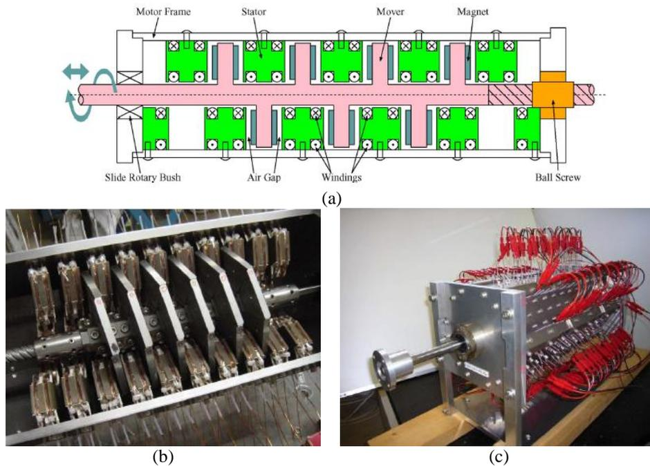
Fig. 1-15. Spiral actuator proposed by Fujimoto *et al.* a) Structure, b and c) prototype [29]
