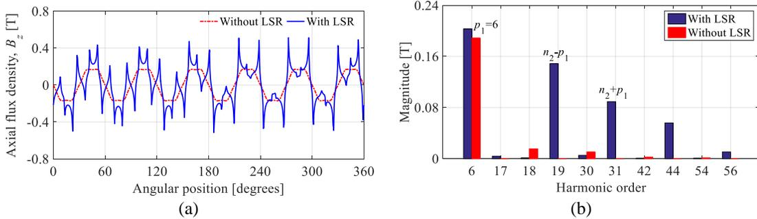
Fig. 3-34. a) Axial flux density near fixed rotor 3 due to magnets only on the high-speed rotor (rotor 1) at a radius of  $r=137$  mm and an axial distance of 0.5 mm. b) Harmonic contents of the modulated flux density.
