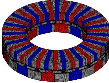
Fig. 3-12. Generated mesh using JMAG FEA software
