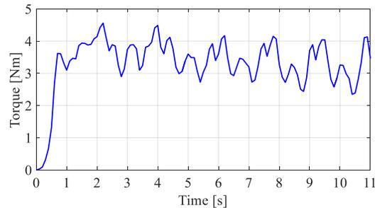
Fig. 2-50. Measured torque while inner rotor was rotated and translator was free to move.
