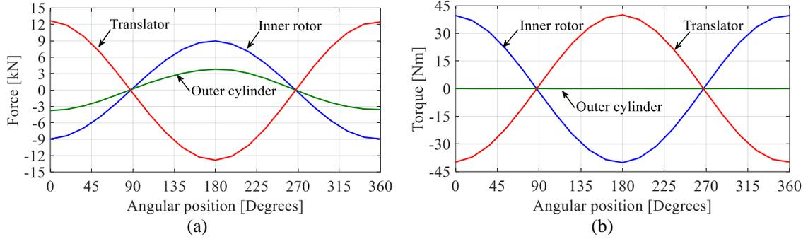
Fig. 2-19. a) Force, and b) torque on different parts of the MGLS due to rotation of the inner rotor
