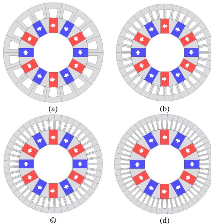
Fig. 3-28. Stator and the high speed rotor of the proposed axial flux magnetically geared motor with a) 18, b) 36, c) 45, and d) 54 stator slots.
