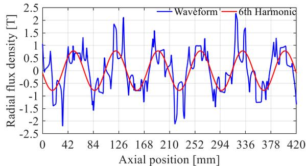
Fig. 2-18. Radial flux density in the outer air-gap due to magnets on both the inner and outer rotor.
