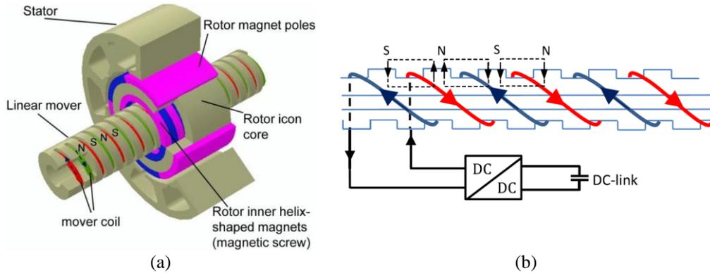
Fig. 1-29. a) Lue's proposed electromagnetic lead screw. b) helical winding structure [51]
