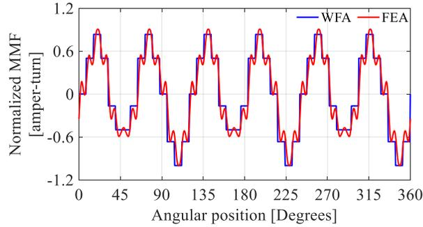
Fig. 3-36. Normalized MMF using the winding function analysis and FEA.
