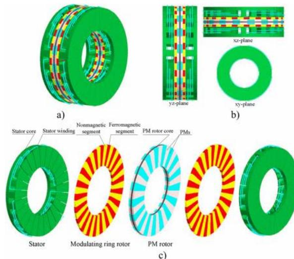
Fig. 3-6. Structure of the proposed AFMGM by Tong *et al.* [65]
