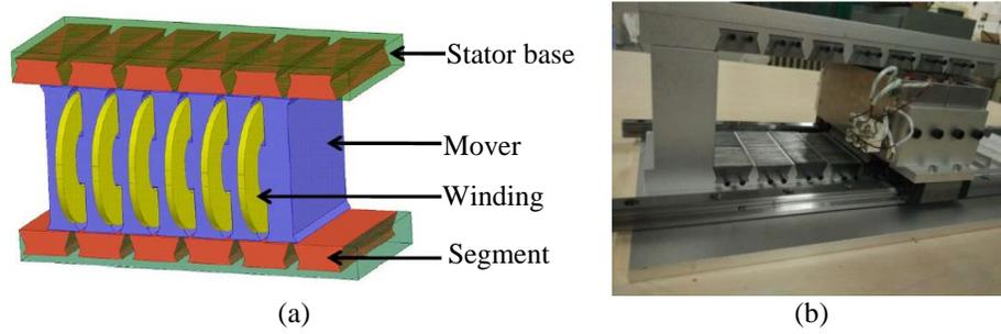
Fig. 1-10. Linear switched reluctance motor presented by D. Wang *et al.* [23] ; a) 3D FEA, and b) prototype.
