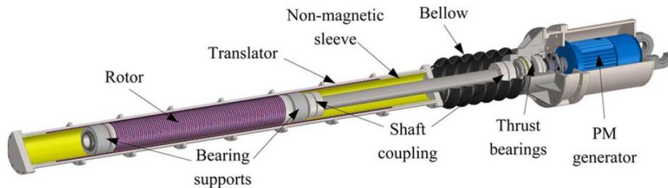
Fig. 1-26. CAD model of the proposed magnetic lead screw by Holm *et al.* [47]
