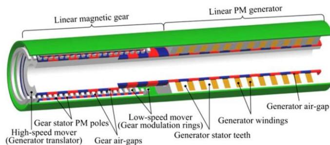
Fig. 1-20. Integration of LMG with linear tubular generator [44]
