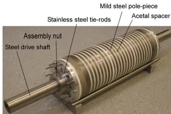
Fig. 1-24. Pole-piece translator of the Holehouse's linear magnetic gear [43]
