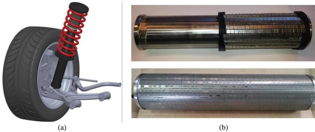
Fig. 1-28. a) Magnetic lead screw suspension system. b) Translator assembly procedure[49]
