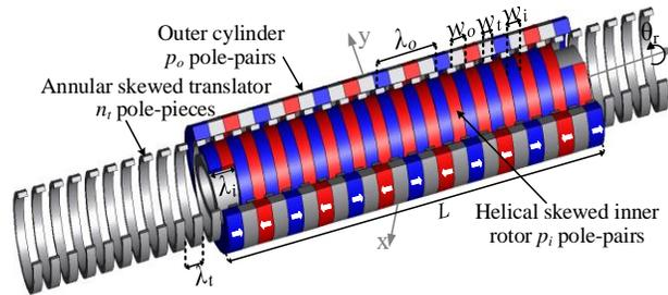
Fig. 2-11. Structure of the magnetically geared lead screw with  $p_i=15$  inner rotor pole-pairs,  $p_o = 6$  pole pairs and  $n_t= 21$  segments across the axial length.
