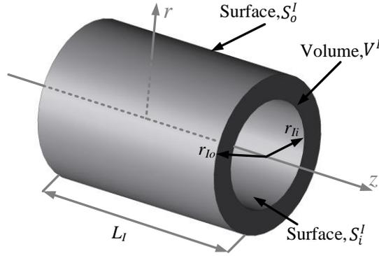
Fig. 4-20. Geometry definition for inner part of the MLS
