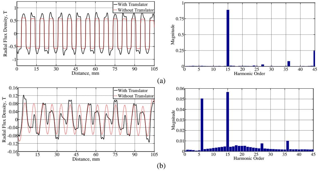
Fig. 2-7 Radial flux densities and related spectrums: a) adjacent to inner rotor due to inner rotor magnets at  $r=17.55$  mm), b) adjacent to outer rotor due to inner rotor magnets (at  $r=19.95$  mm).
