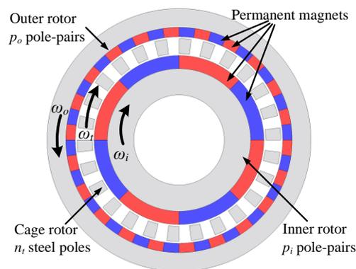
Fig. 1-18. Coaxial magnetic gear with  $p_1 = 4$ ,  $n_2 = 26$ , and  $p_3 = 22$ .
