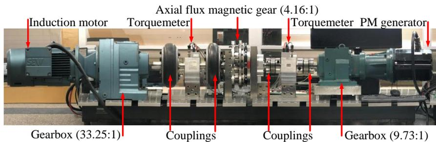
Fig. 3-21. Axial magnetic gear on the test bed
