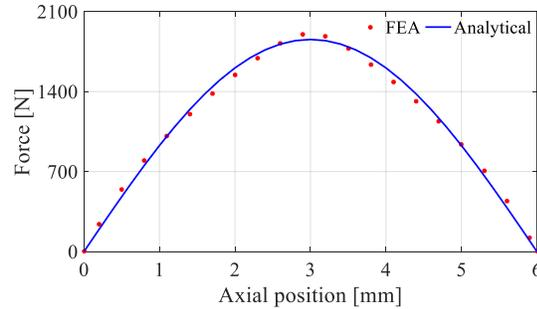
Fig. 4-25. Calculated force using FEA and analytical model
