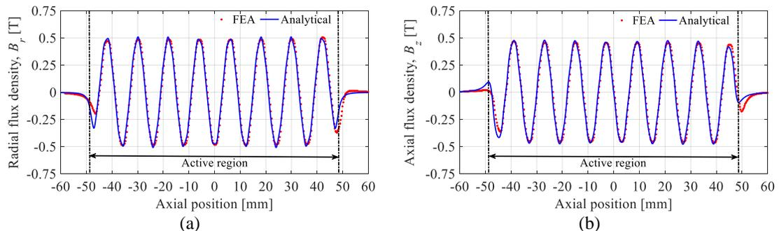
Fig. 4-8. FEA and analytically calculated magnetic flux density a) radial b) axial
