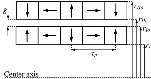
Fig. 4-10. A 2D cut-view of a Halbach cylinder
