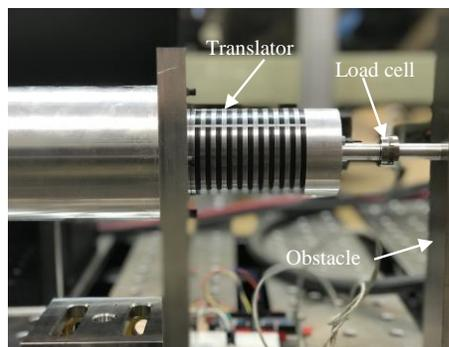
Fig. 2-46. Test setup for force measurement
