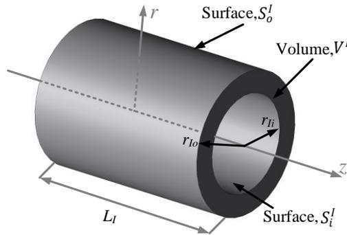
Fig. 4-4. Geometry definition for inner part of the linear coupling
