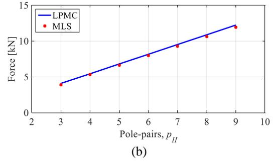
Fig. 4-26. Case 1: calculated force of LPMC and MLS a) using FEA and b) using analytical model
