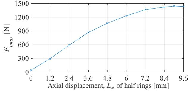
Fig. 2-38. Maximum translator force versus axial shift,  $L_a$  of the half rings
