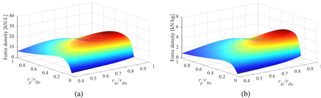
Fig. 4-14. a) Volumetric force density, and b) mass force density as a function of  $\tau_p/r_{II0}$  and  $r_{I0}/r_{II0}$ , when  $r_{II0} = 30$  mm and  $r_{II}/r_{I0} = 0.7$ .
