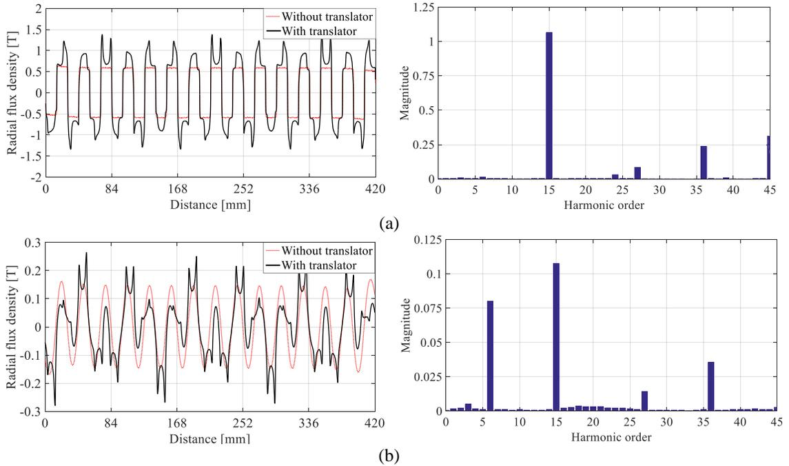
Fig. 2-17. Radial flux densities and related spectrums: a) adjacent to inner rotor due to inner rotor magnets at  $r=48.1$  mm, b) adjacent to outer rotor due to inner rotor magnets (at  $r=54.9$  mm).
