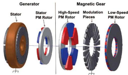
Fig. 3-2. An axial flux magnetically geared machine proposed by Wang *et al.* [67]
