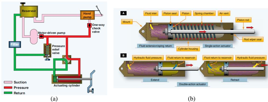
Fig. 1-4. a) basic hydraulic system, b) linear hydraulic actuator [11]
