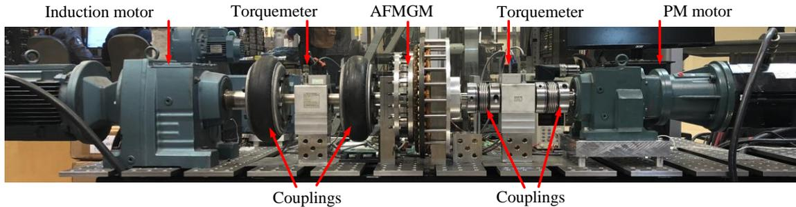
Fig. 3-41. Axial flux magnetically geared machine on the test bed.
