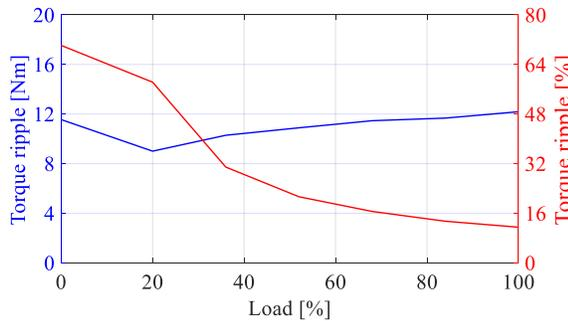
Fig. 3-26. Torque ripple as a function of load for high-speed rotor.
