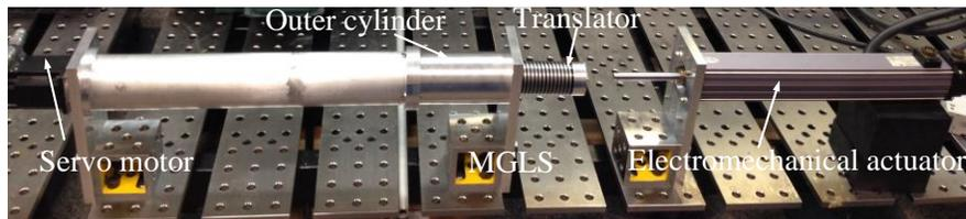
Fig. 2-30. The MGLS on the testbed before testing.
