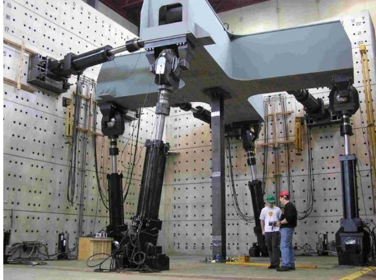
Fig. 1-2. 6 DOF earthquake simulator built at the University of Minnesota [4]
