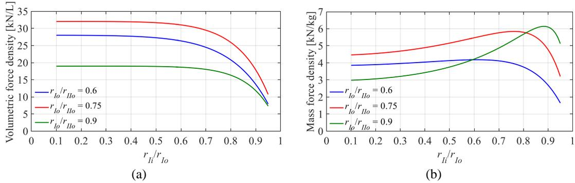
Fig. 4-13. a) Volumetric and b) Mass force density as a function of  $r_{II}/r_{I0}$  for three different value of  $r_{I0}/r_{II0}$ , when  $r_{II0} = 30$  mm and  $\tau_p/r_{II0} = 0.3$ .
