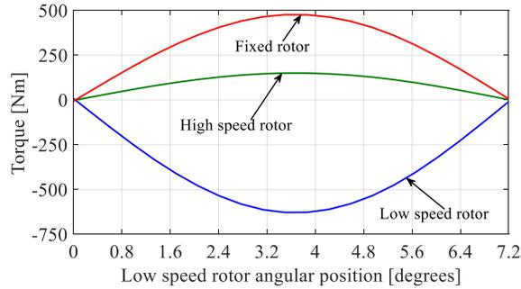
Fig. 3-15. Torque on the low speed rotor (LSR), high speed rotor (HSR) and fixed rotor for the case when only the low speed rotor is rotating with practical design considerations.
