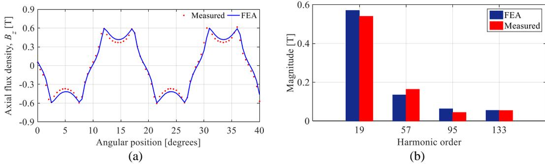
Fig. 3-20. a) Fixed rotor axial magnetic flux density field when the rotor surrounded by air at  $r = 135\text{mm}$  and  $z = 1.04\text{mm}$  above the rotor b) Corresponding harmonic analysis showing the 19th, 57th, 95th, and 133rd harmonic for measured and FEA calculated axial flux density for the fixed rotor (when surrounded by air).
