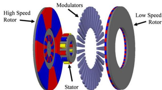
Fig. 3-4. AFMG proposed by Johnson *et al.* [69]
