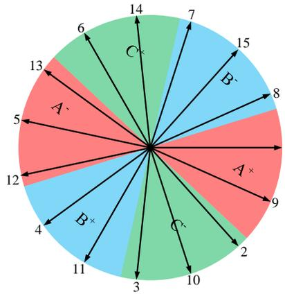
Fig. 3-29. Star of slots phasor diagram of a 45-slots/12-poles motor.
