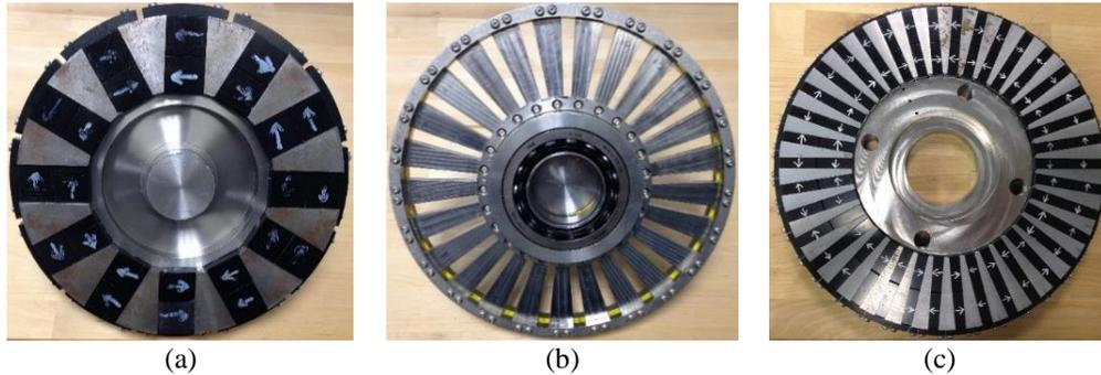
Fig. 3-18. The experimentally assembled axial flux focusing magnetic gear with a) high-speed rotor, b) low-speed rotor, and c) fixed rotor.
