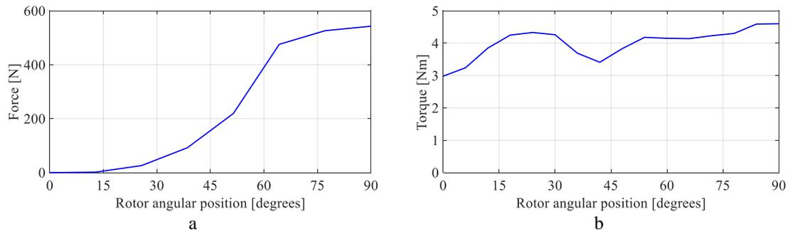
Fig. 2-48. a) Measured translator force, b) measured inner rotor torque, when inner rotor was rotated while translator pushed against an obstacle.
