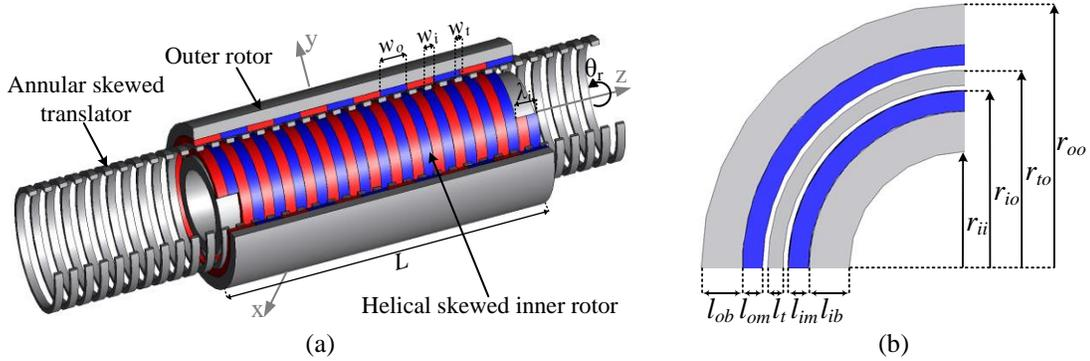
Fig. 2-1. MGLS proof of concept design; a) 3D view, b) cross-sectional parameters
