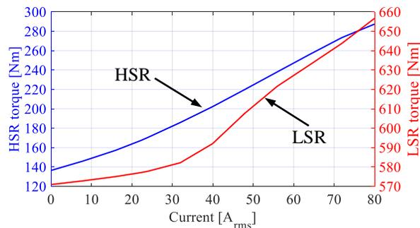
Fig. 3-39. Torque on the low-speed rotor and high-speed rotor as a function of stator current for the case when a fill factor of 0.3 was used. This lower fill factor was used as it was closer to the experimental value used in the prototype. A stator current of 25.4 A<sub>rms</sub> corresponds to a current density of 6.5A/mm<sup>2</sup>
