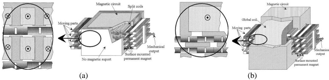
Fig. 1-16. One phase of the multi-airgap actuator a) distributed, b) global coil [17].
