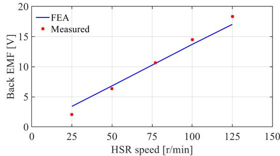
Fig. 3-44. Simulated and measured peak back-EMF at different speeds
