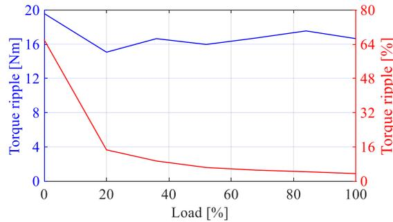
Fig. 3-25. Torque ripple as a function of load for low speed rotor.
