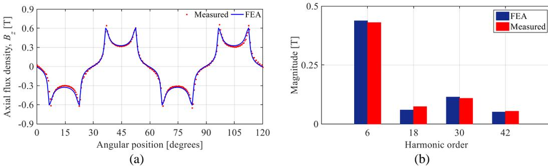
Fig. 3-19. a) High speed rotor axial magnetic flux density at  $r = 135\text{mm}$  and  $1.04\text{mm}$  above the axial rotor and b) corresponding spatial harmonic comparison showing the 6th, 18th, 30th, and 42nd harmonic for the measured and FEA calculated axial flux density (when surrounded by air).
