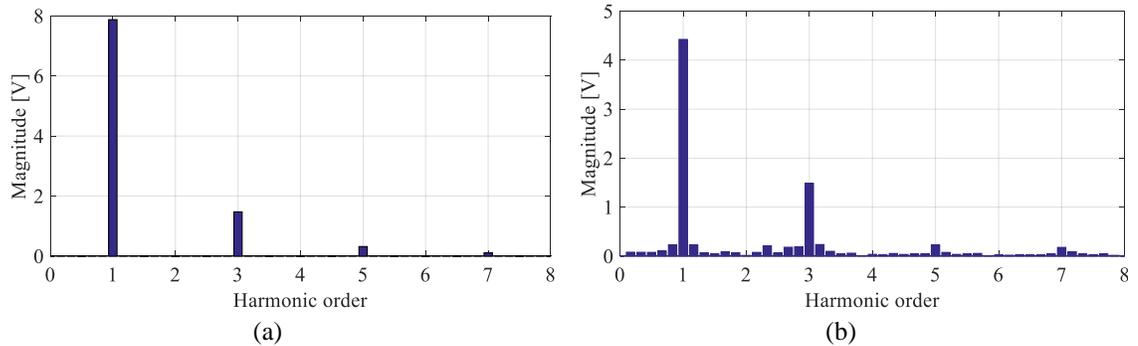
Fig. 3-43. Harmonic spectrum of the a) calculated and b) measured no load back-emf voltage.
