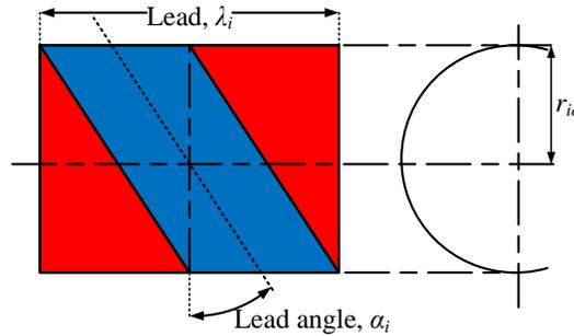
Fig. 2-3. Side view of the helical lines of the inner rotor
