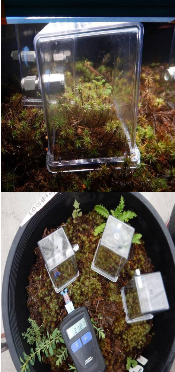
Figure 4.3 Magenta vessel™ used to collect isoprene emission data from P. juniperinum populations before and after nitrogen addition. Seen here inverted with Pressure-Lok® precision analytical syringe (VICI Precision Sampling Inc., Baton Rouge, LA, USA).
