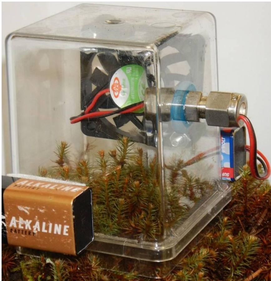
Figure 4.2 Small 77mm × 77 mm × 97mm static chamber (magenta jar) created for headspace analyses using (Magenta vessel™). Equipped with battery-operated fan to ensure equal mixing of air in the chamber and avoid settling.
