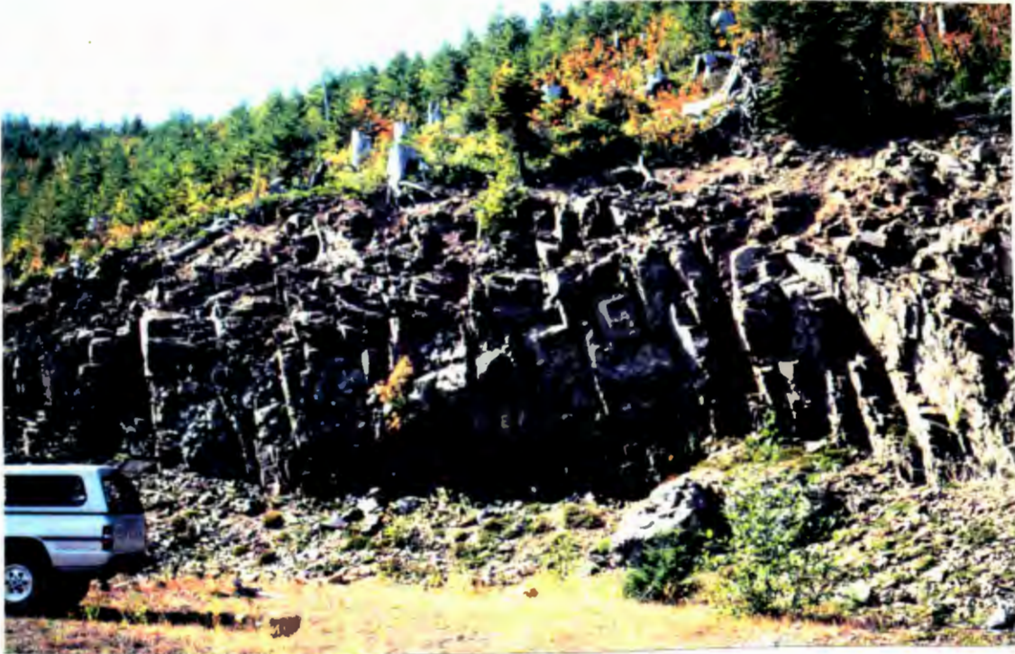
Figure 21. Vertically oriented jointing - FS Rd. 53, SE 1/4 sec. 28, T.5 N. R..5 E. Many bedrock units display a pronounced near vertical joint habit. Lack of a continuous, normal joint direction results in the unexpected degree of stability. Minor rockfall occurs but is very limited.
