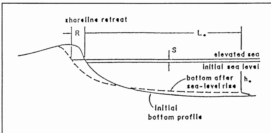
Figure 3. Translation of a beach and nearshore profile after a relative rise in sea-level, where  $R$  is retreat,  $L$  is the across-shore distance to water depth  $h$ , and  $S$  is amount of sea-level rise (Komar and others, 1991).
