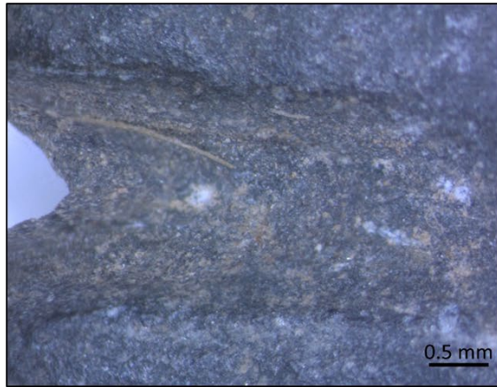
Photo 183. Photomicrograph of striations and groove on 35CO2-481, 25.2x.
