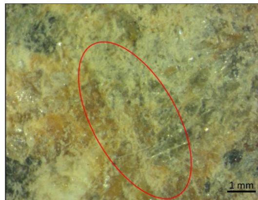
Photo 42. Photomicrograph of KPM-19 post modification showing remnant chopper scar, 31.5x.
