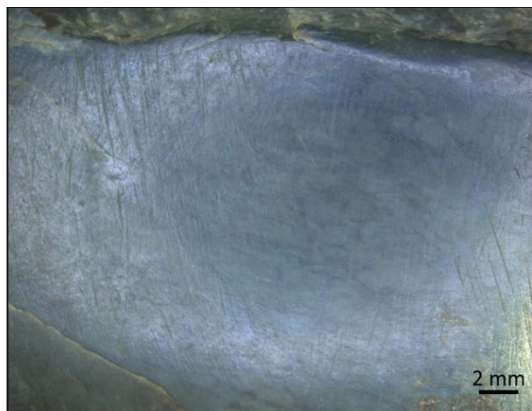
Photo 73. Photomicrograph of 35CO2-427 showing striations, 4.095x.
