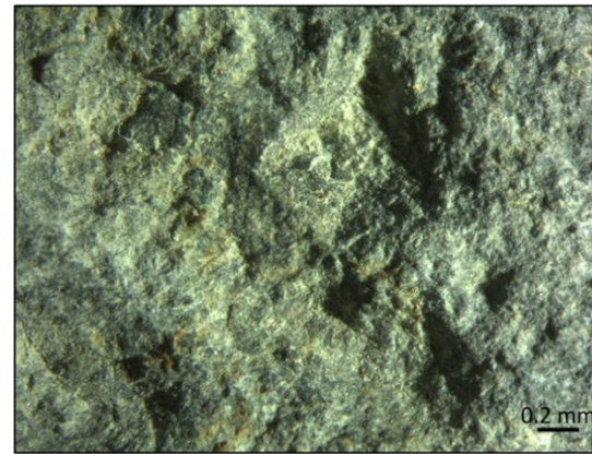
Photo 46. Photomicrograph of KPM-4 post modification showing sharp asperities and grain crushing, 13x.
