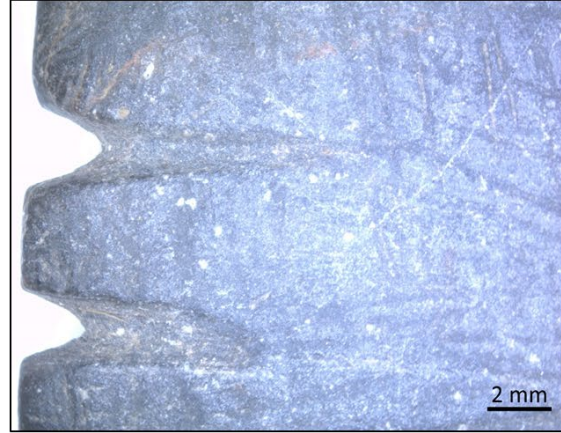
Photo 182. Photomicrograph of striations and grooves on 35CO2-481, 6.3x.
