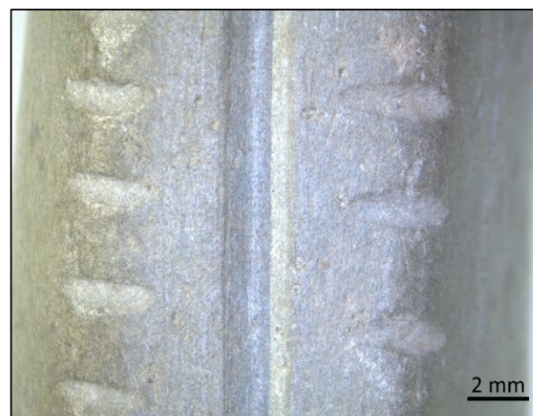
Photo 70. Photomicrograph of 35CO2-426 showing notching at mane, 6.3x.
