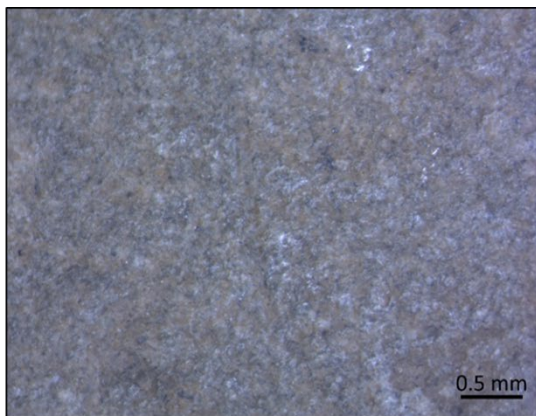
Photo 69. Photomicrograph of 35CO2-426 showing rounded grains and polish, 25.2x.
