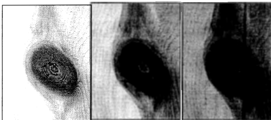
Figure 101. Image of knot with sap stain in Pine wood shown as red, green, and blue color channel images, respectively.
