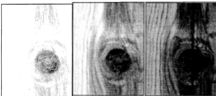
Figure 98. Image of ring knot with sap stain in Pine wood shown as red, green, and blue color channel images, respectively.
