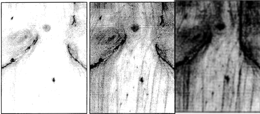
Figure 59. Image of core defects in Oregon Ponderosa Pine wood shown as red, green, and blue color channel images, respectively.
