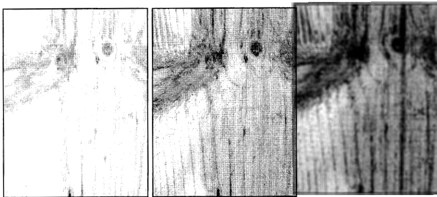
Figure 53. Image of core defects in Arizona White Pine wood shown as red, green, and blue color channel images, respectively.
