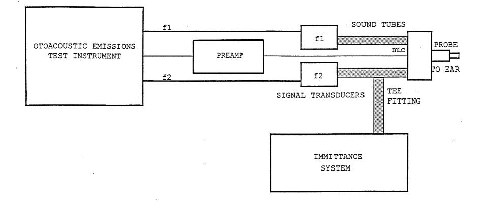
Figure 1. Schematic drawing of probe assembly.
