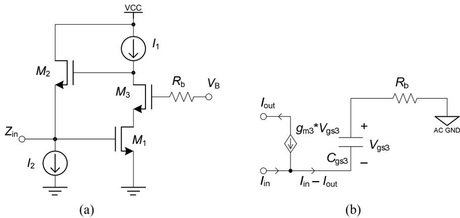
Figure 2-18 (a) Adding  $R_b$  to the cascode active inductor. (b) Small-signal equivalent circuit of  $M_3$  and  $R_b$ .
