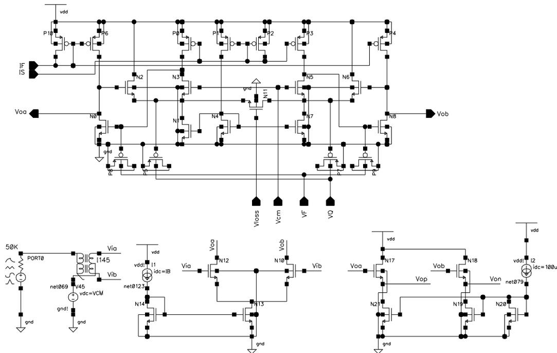
Figure 3-6 Active-inductor bandpass filter example.
