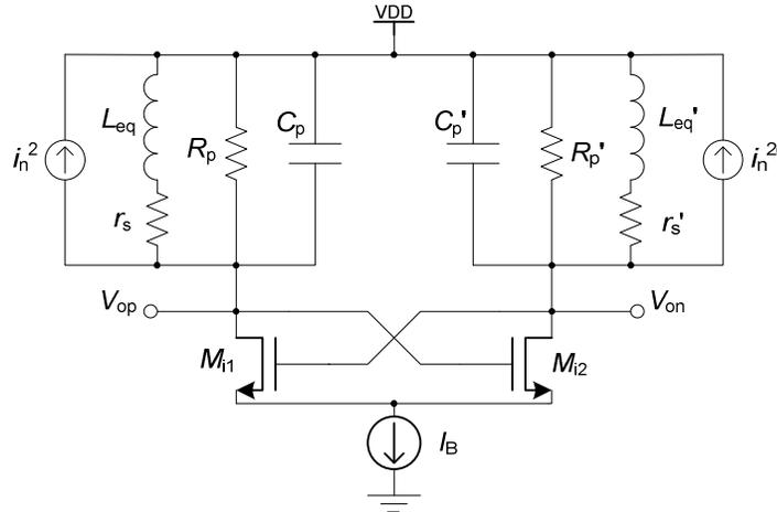
Figure 4-7 The equivalent circuit of the active-inductor oscillator showing the noise elements.
