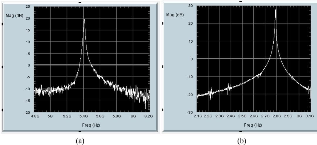
Figure 5-24 Measured frequency responses of the bandpass filters (S21). (a)  $L_{\text{gate}} = 0.2 \mu\text{m}$ ,  $f_0 = 5.4$  GHz,  $Q = 365$ ; (b)  $L_{\text{gate}} = 0.4 \mu\text{m}$ ,  $f_0 = 2.79$  GHz,  $Q = 661$ . The midband gain is set at 20 to 30 dB for high SNR and can be adjusted via  $I_B$ .
