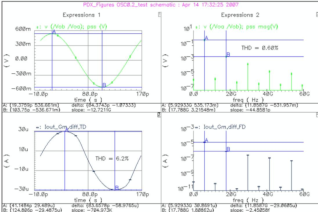
Figure 4-11 PSS simulation results of the oscillator. (1) Output voltage  $V_{oa} - V_{ob}$  in time domain. (2) Spectrum of  $V_{oa} - V_{ob}$ . (3) Output current of differential-pair  $G_M$  in time domain. (4) Spectrum of  $G_M$  output current.
