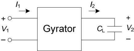
Figure 2-1 Implementing an active inductor using a gyrator.
