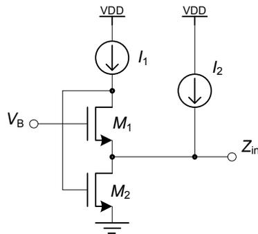
Figure 2-13 Wu and Ismail's solution to dc biasing difficulty: injecting extra current  $I_2$  into  $M_2$  to raise  $V_{GS2}$  without increasing  $V_{GS1}$ , which will increase the  $V_{DS1}$  requirement and defeat the margin gained through the increase in  $V_{GS2}$ .
