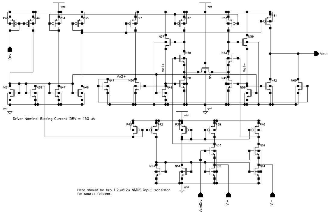
Figure 5-8 The output-driver circuit schematic.
