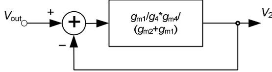
Figure 2-36 The local feedback loop within the circuit.
