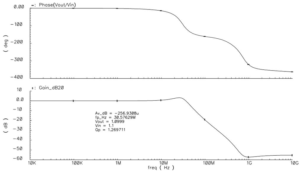
Figure 2-41 The frequency response of the analog signal driver.
