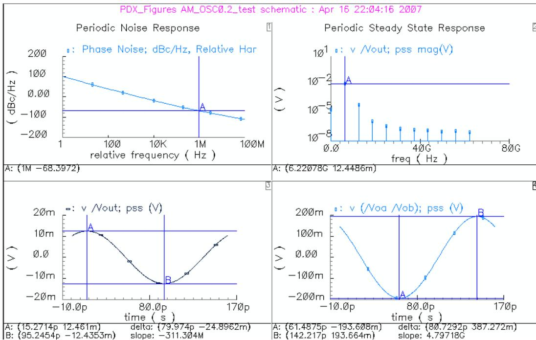
Figure 5-18 Simulation results of the fabricated 5-GHz oscillator with output buffer and load.
