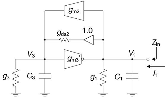
Figure 2-47 Small-signal equivalent circuit of the all-NMOS-II active inductor.
