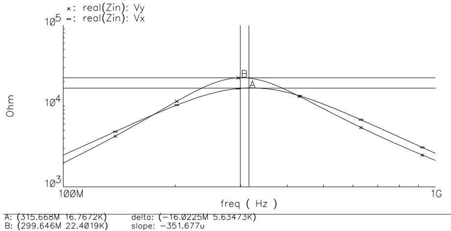
Figure 2-16 Simulated  $R_p$  of the circuits in Fig. 2-15.  $V_x$  and  $V_y$  are from the circuits in Fig. 2-15(a) and (b), respectively.
