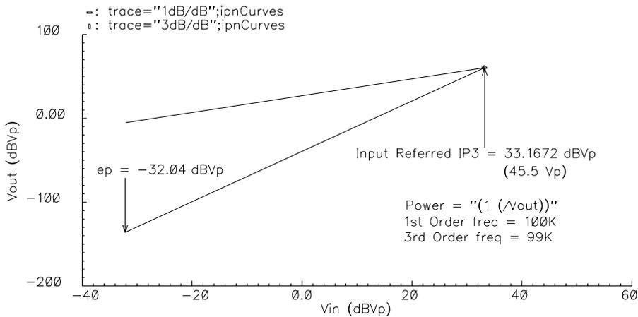
Figure 2-43 The IIP3 of the circuit is 33 dBVp or 45.5 Vp, at 1.8 V power supply, single-ended.
