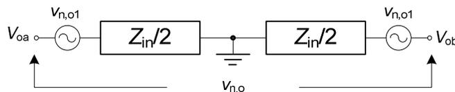
Figure 2-30 The noise model of a pseudo-differential active inductor.
