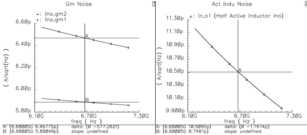
Figure 2-33 Noise simulation results of the  $G_M$  cells in the active inductor in Fig. 2-29(a). The biasing conditions are given in Fig. 2-29. Panel 1 shows the output noise current of  $G_{M1}$  and  $G_{M2}$ , respectively. Panel 2 shows the output noise current of the active inductor. All data are extracted from half of the circuit in a pseudo-differential structure.
