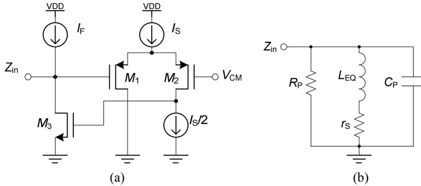
Figure 2-23 (a) Karsilayan's active inductor circuit.  $V_{CM}$  is a dc voltage that sets the circuit's common-mode voltage. (b) Small-signal ac equivalent circuit.
