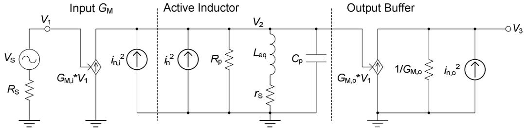
Figure 3-5 Small-signal equivalent circuit of the bandpass filter with noise elements.
