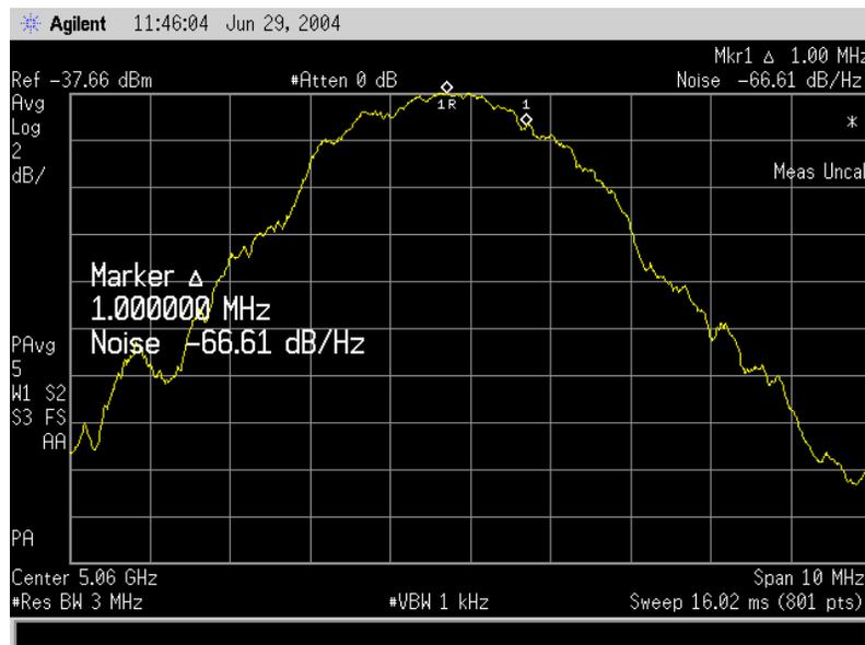
Figure 5-16 Measured phase noise of the 5-GHz oscillator, including the output buffer.
