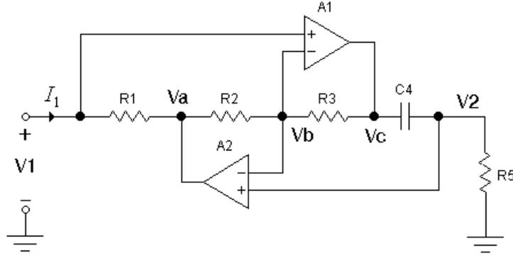
Figure 2-2 Implementing an active inductor using two opamps.
