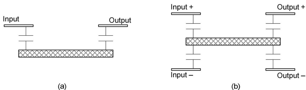
Figure 5-1 Substrate and interconnect coupling. (a) Single-ended circuit. (b) Differential circuit.
