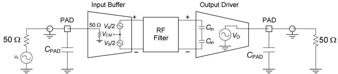
Figure 5-2 The need for input and output buffers/drivers.
