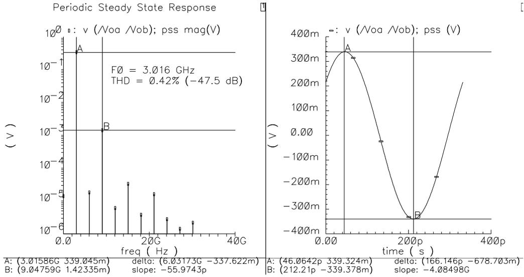
Figure 4-13 Simulation results of the  $L = 0.4 \mu\text{m}$  oscillator (OSC0.4).
