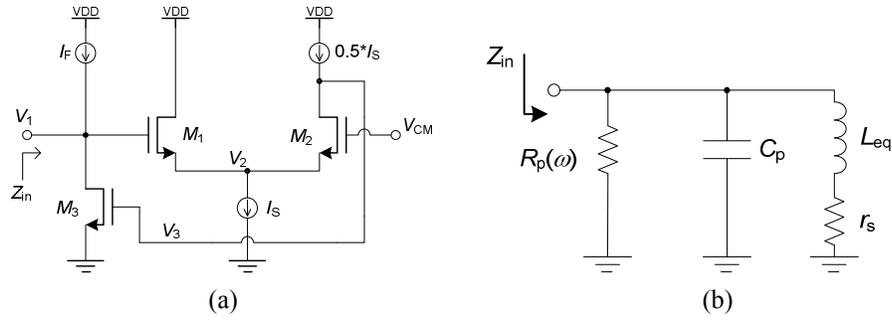
Figure 2-27 (a) The all-NMOS signal-path active-inductor circuit. (b) Equivalent circuit.
