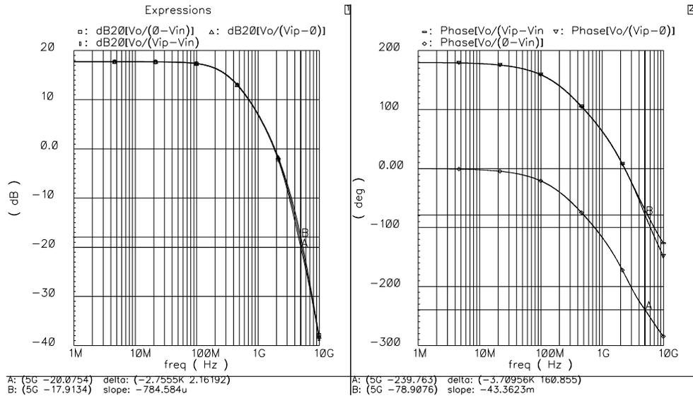
Figure 5-9 The simulation results of the output driver. Panel 1: cursors A and B are gains from single-ended input on the  $V_{ip}$  and  $V_{in}$  terminals, respectively. The differential-input gain,  $V_o/(V_{ip} - V_{in})$ , is  $-19.05$  dB.
