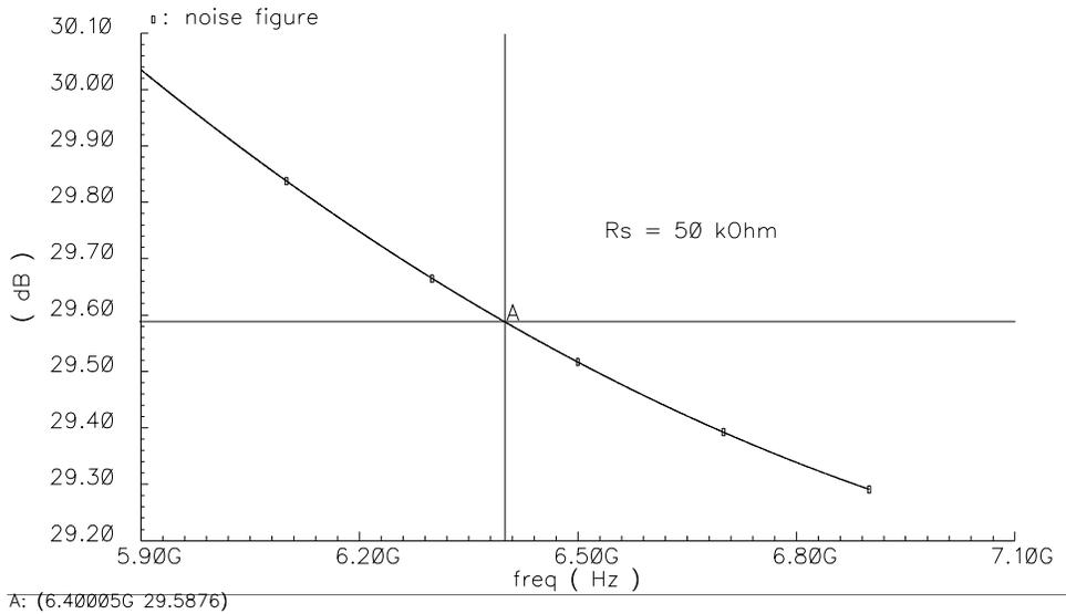
Figure 3-8 Noise simulation results, pseudo-differential, outputs taken at the source-follower output.
