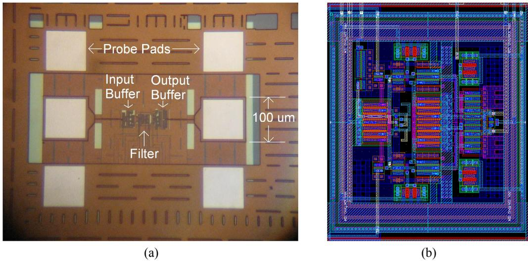
Figure 5-11 (a) The 0.2- $\mu\text{m}$ -bandpass-filter (BP0.2) module layout (microphotograph). (b) The BP0.2 filter-core layout (screen capture).
