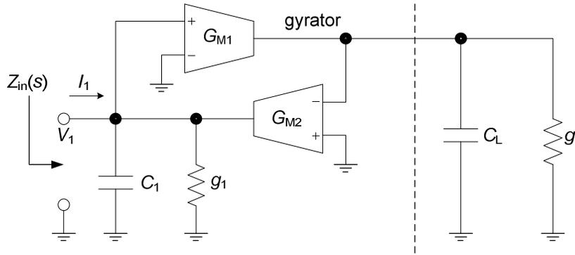
Figure 2-3 Implementing an active inductor using OTAs or  $G_M$ s.
