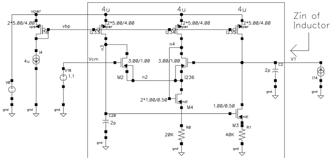
Figure 2-49 The all-NMOS-II circuit configured as an active inductor.
