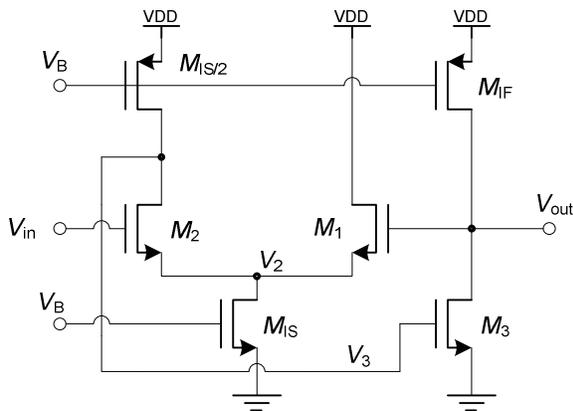
Figure 3-9 Implementing a lowpass filter using the all-NMOS active inductor.
