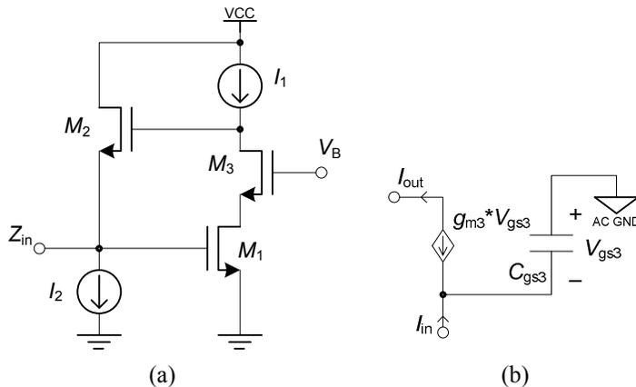
Figure 2-17 (a) Cascode active inductor. (b) small-signal equivalent circuit of  $M_3$ .
