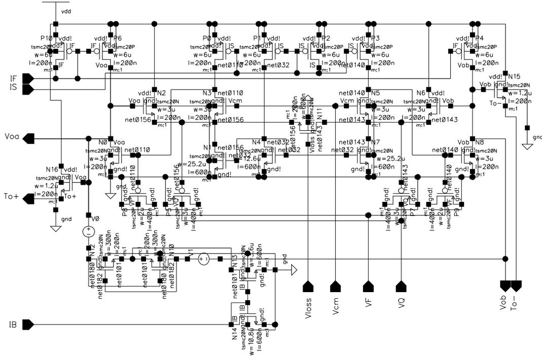
Figure 4-8 The oscillator circuit.  $I_S = I_F = 250 \mu\text{A}$ ,  $I_B = 50 \mu\text{A}$ ,  $V_F = V_Q = 0.5$ ,  $V_{CM} = 1.35$ ,  $V_{loss} = 0$ .
