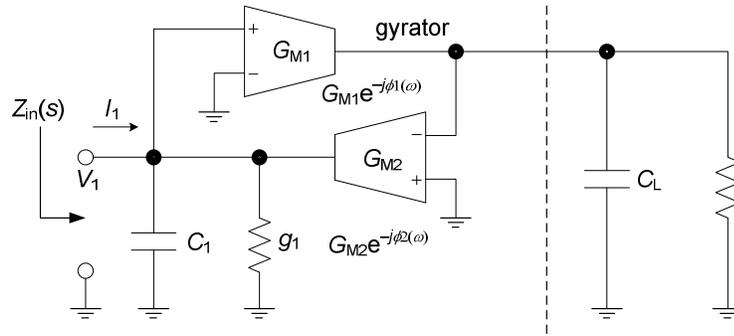
Figure 2-24 The gyrator equivalent circuit of an active inductor. The phase lags of the  $G_M$  cells are shown to analyze their effect on  $Q$ .
