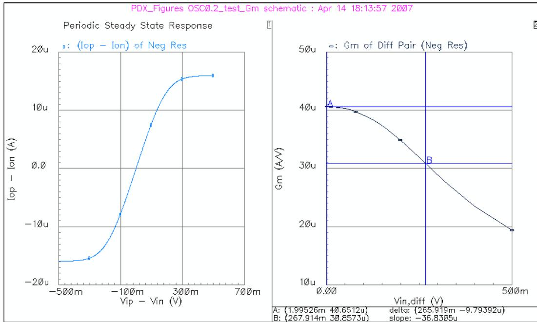
Figure 4-9 The limiting effect of the differential-pair negative resistor. (a) dc simulation results; (b) Periodical Steady State (PSS) simulation results. Markers A and B show the maximum  $G_M$  and steady-oscillator  $G_M$ , respectively.
