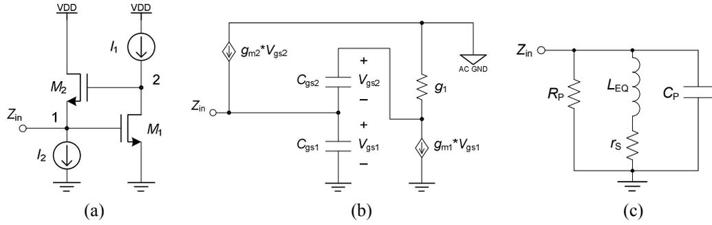
Figure 2-14 Common-Source Common-Drain (CS-CD) active inductor. (a) The circuit. (b) Small-signal ac equivalent circuit.  $g_1$  is  $g_{ds1} + g_{ds1}$ . (c) Equivalent circuit showing the inductor.
