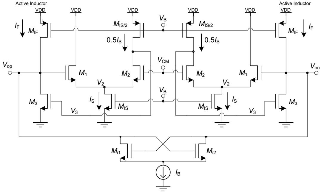
Figure 4-5 The all-NMOS active-inductor oscillator in a pseudo-differential structure.
