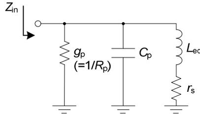
Figure 2-4 Equivalent circuit of a  $G_M$ - $C$  active inductor.
