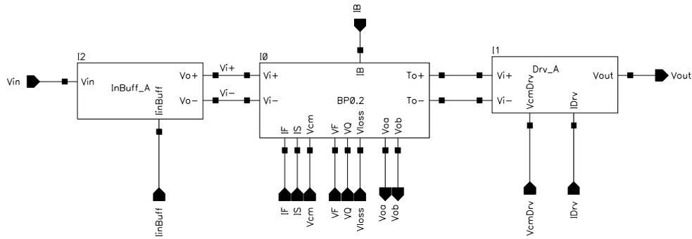
Figure 5-10 Regular- $Q$  0.2- $\mu\text{m}$ -gate-length bandpass-filter module (BP0.2).
