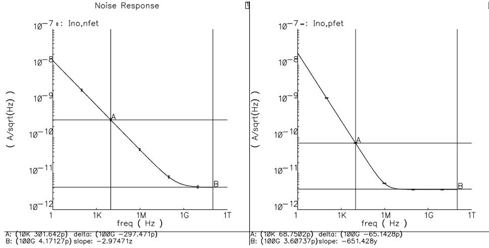
Figure 2-32 The output noise currents of an NFET and a PFET in TSMC 0.18- $\mu\text{m}$  CMOS. Cursor A rests on  $1/f$  noise region; cursor B rests on thermal noise region.
