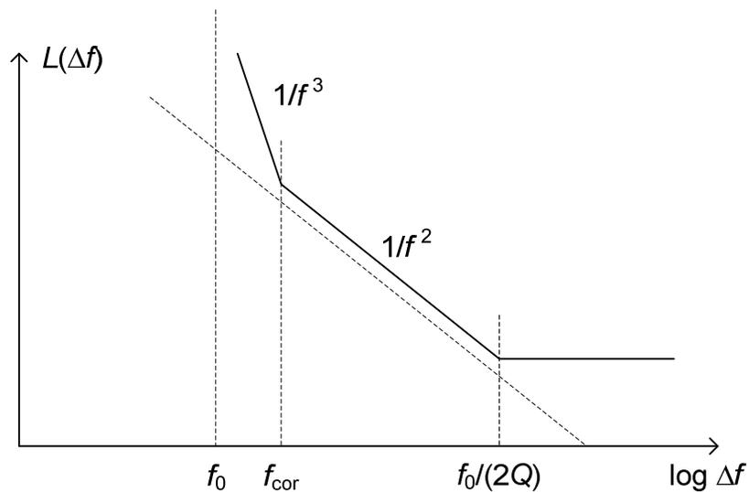
Figure 4-6 A typical oscillator phase-noise profile.
