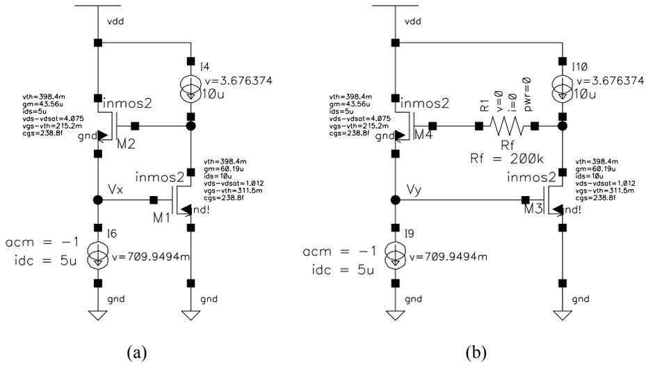
Figure 2-15 (a) A CS-CD active inductor simulation circuit.  $g_{ds1} = 0.597$  pS. (b) With a  $Q$ -enhancing resistor  $R_f$ .
