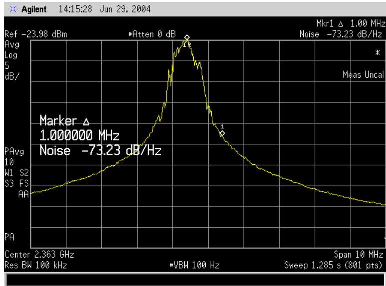
Figure 5-22 Measured phase noise of the 2.6-GHz oscillator (OSC0.4,  $L = 0.4 \mu\text{m}$ ).
