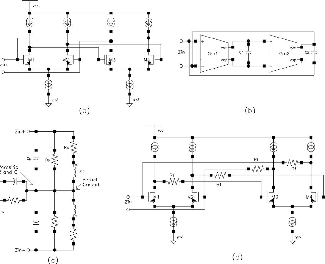
Figure 2-22 The differential-pair active inductor.
