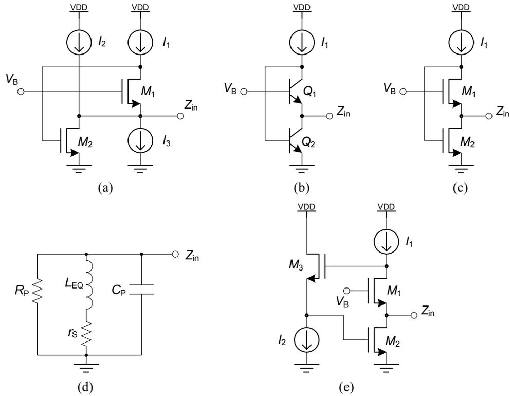
Figure 2-12 Derivation of the cascode CG-CS active inductor. (a) Circuit derived from signal flow. (b) BJT version. (c) CMOS version. (d) Equivalent circuit. (e) Modified cascode CG-CS.
