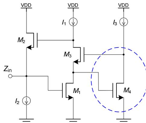
Figure 2-21 Regulated cascode active inductor circuit.
