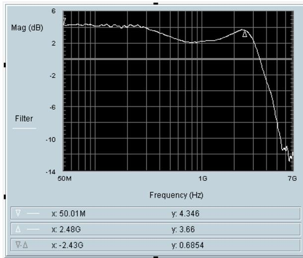
Figure 5-35 0.2- $\mu\text{m}$  lowpass filter frequency response, after subtracting the reference channel. (Data Ref# LP0.2-C28-VNA-00090 and Ref-C26-VNA-00080)
