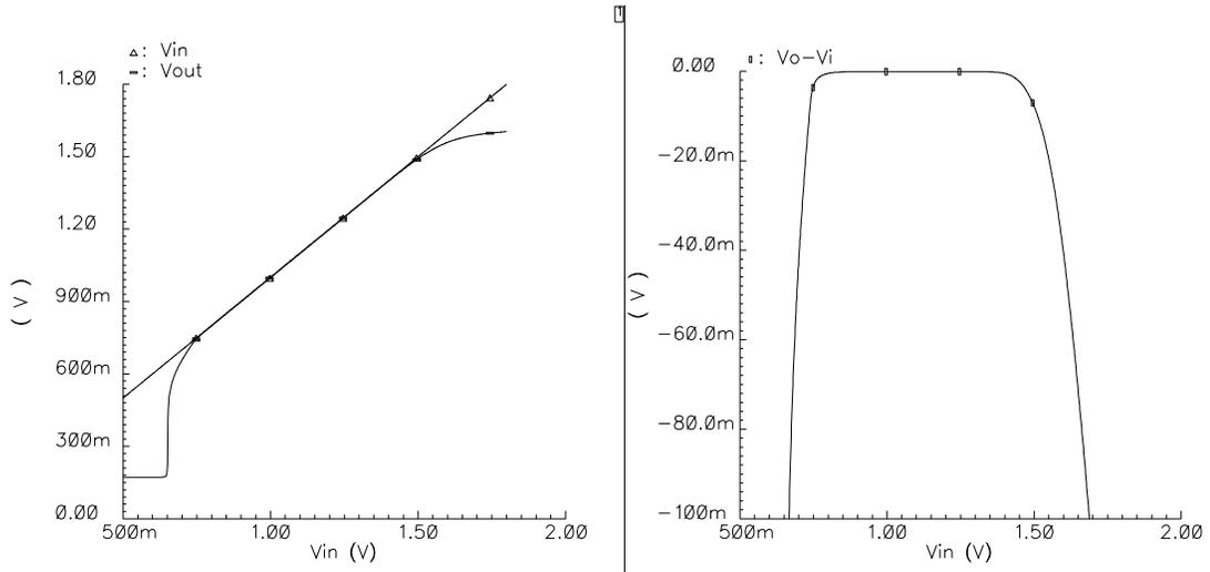
Figure 2-42 dc characteristics of the analog signal driver.
