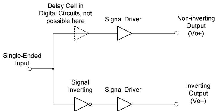
Figure 5-3 The signal path of single-ended to differential conversion.
