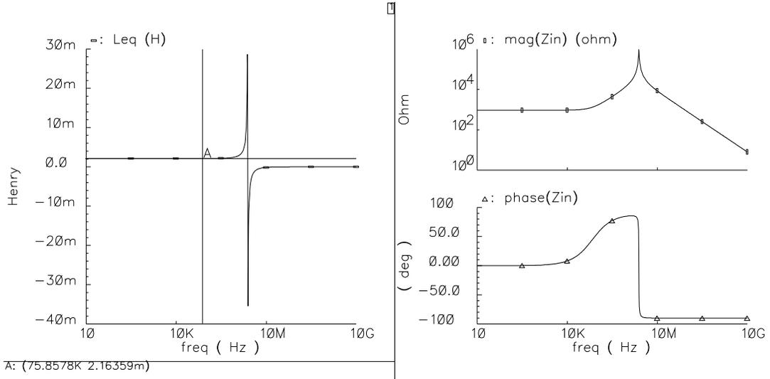
Figure 2-50 Example ac simulation results of the all-NMOS-II active inductor.
