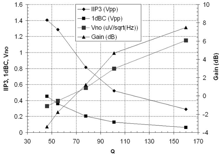
Figure 5-29 Plot of  $IIP3$ , input 1-dB compression point, and equivalent output noise.
