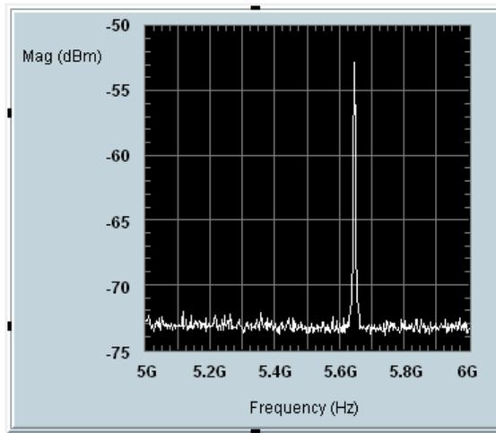
Figure 5-15 Output spectrum of a 5.6-GHz oscillator (including a 50- $\Omega$  output driver). The center frequency is  $f_0 = 5.645$  GHz, the magnitude is  $-52.78$  dBm, corresponding to a peak voltage of 134 mV at the circuit core. The attenuation of the output buffer at 5.645 GHz is 39.3 dB. The 2nd and higher harmonics are below the noise floor ( $\approx -73$  dBm). (Data Ref# OSC0.2-C22-SPA-00040)
