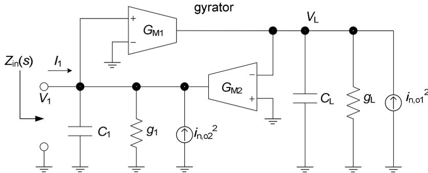
Figure 2-26 A gyrator-based active inductor showing noise elements.
