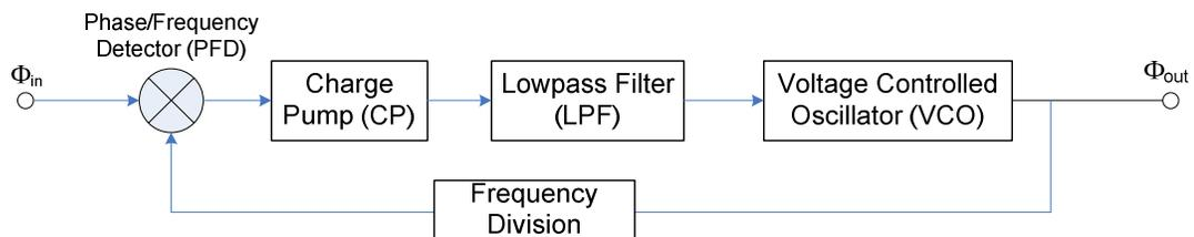
Figure 1-2 Block diagram of a charge-pump PLL.
