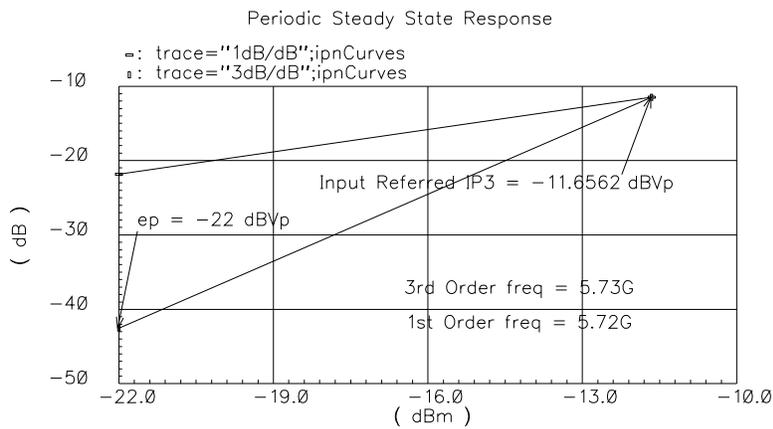
Figure 5-26 Simulation results of  $IIP3$ , which is 0.523  $V_{pp}$ , differentially.
