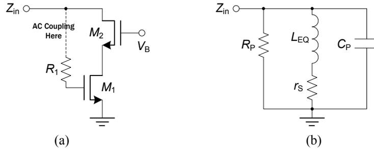
Figure 2-9 Cascode gate- $R$ -II active inductor (Shinji Hara, 1988). (a) Primary circuit with ac coupling shown; (b) Equivalent circuit showing the inductor.
