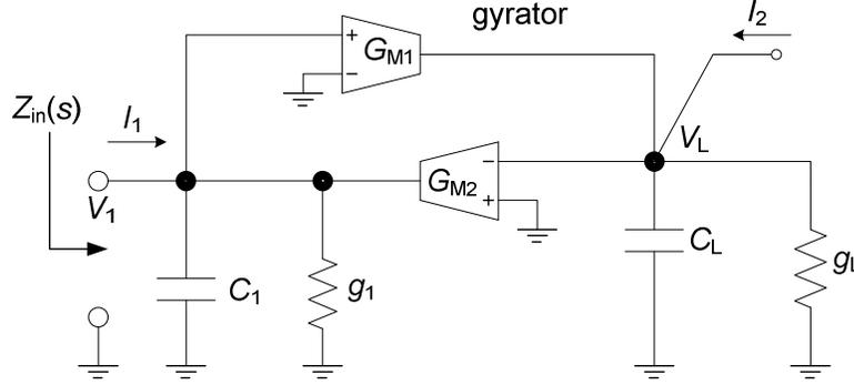
Figure 3-2 Implementing a lowpass filter using the active inductor.
