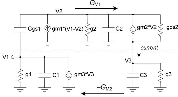
Figure 2-28 Small-signal equivalent circuit of the active inductor in Fig. 2-27(a).  $g_{m1-3}$  are the transconductances of  $M_{1-3}$ , and  $C_{1-3}$  and  $g_{1-3}$  are the total parasitic capacitances/conductances at nodes 1-3, respectively.  $C_2$  also includes the capacitance from a small varactor for  $Q$  tuning.
