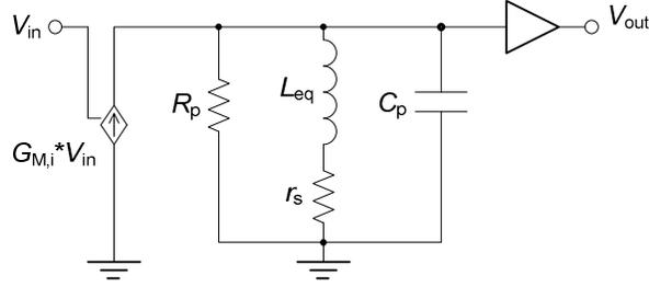
Figure 3-1 Constructing an HF active-inductor bandpass filter.
