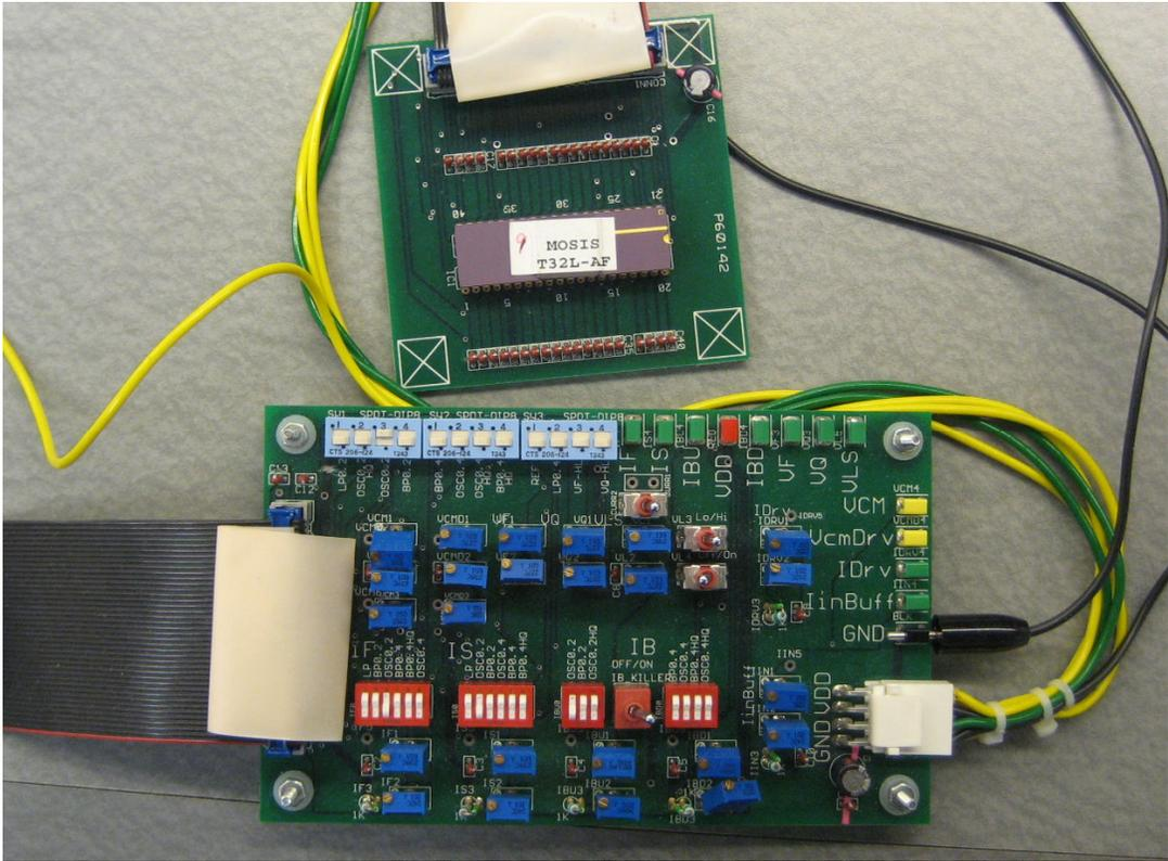
Figure 5-14 Biasing circuit for the test chip. The small circuit board carries the test chip and goes under the microscope. The larger circuit board generates tunable biasing voltage and current.
