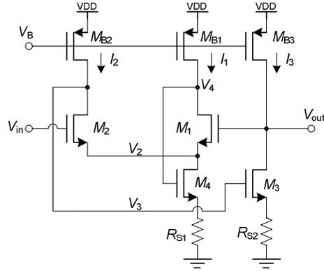
Figure 2-35 The all-NMOS-II circuit configured as a precision analog signal driver.
