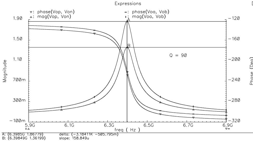
Figure 3-7 Transfer function from ac simulations (pseudo-differential).
