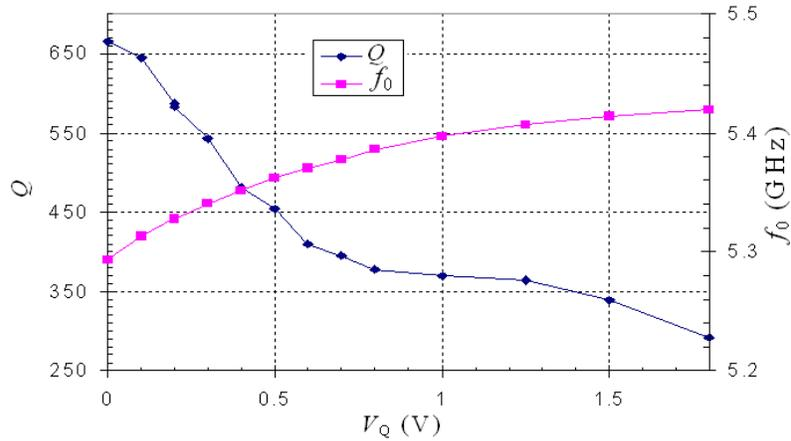
Figure 5-25 Measured  $Q$ -tuning characteristic of the 0.2- $\mu\text{m}$  gate-length bandpass filter vs. the varactor voltage  $V_Q$  for  $292 \leq Q \leq 665$ . Over this range,  $f_0$  decreases from 5.42 GHz to 5.3 GHz (a 2% change). Note that  $Q$  can be tuned over different ranges depending on the baseline  $Q$  as set by the choice of biases. Here, the baseline  $Q$  was set to 410 at  $V_Q = 0.6$  V by choosing  $V_{CM} = 1.29$  V with all other biasing conditions given in Fig. 2-29.
