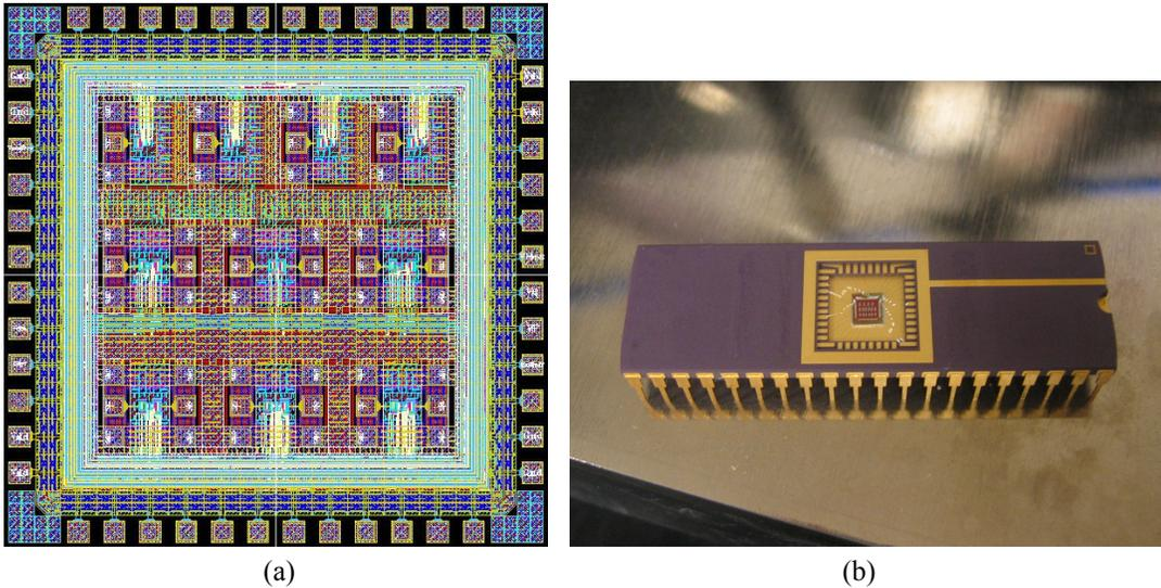
Figure 5-13 (a) The test-chip layout including probe pads and bond pads. (b) The packaged test chip (1 out of a lot of 40).
