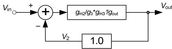
Figure 2-37 The main feedback loop within the circuit.
