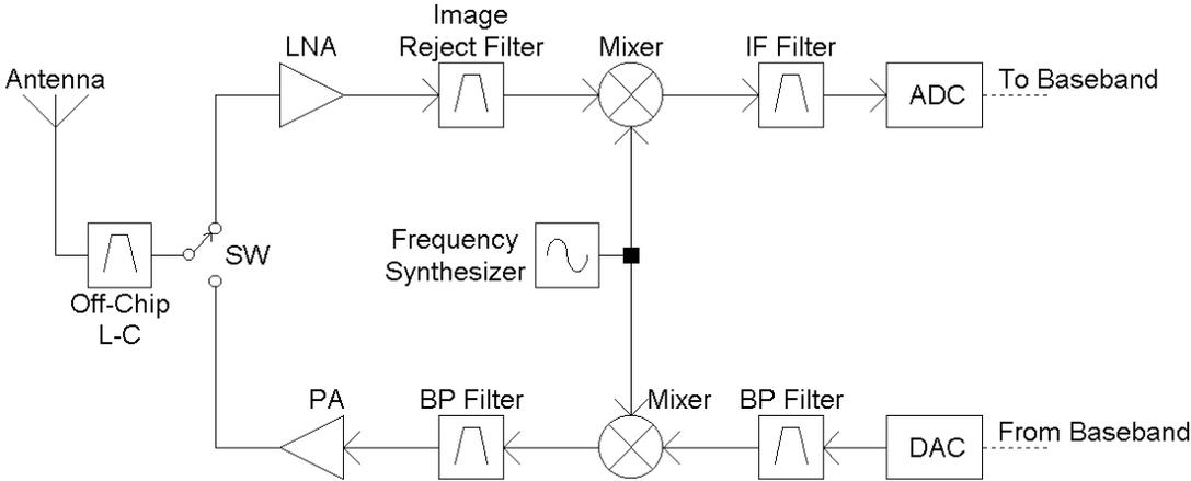
Figure 1-1 The architecture of a wireless communication IC.
