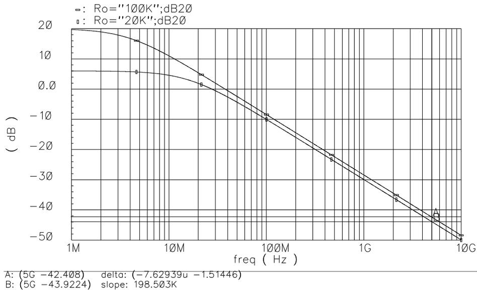
Figure 5-7 The frequency response of the circuit in Fig. 5-6(a).  $C_L = 500$  fF and  $R_O = 20$  k $\Omega$ ;  $C_L = 420$  fF and  $R_O = 100$  k $\Omega$ .
