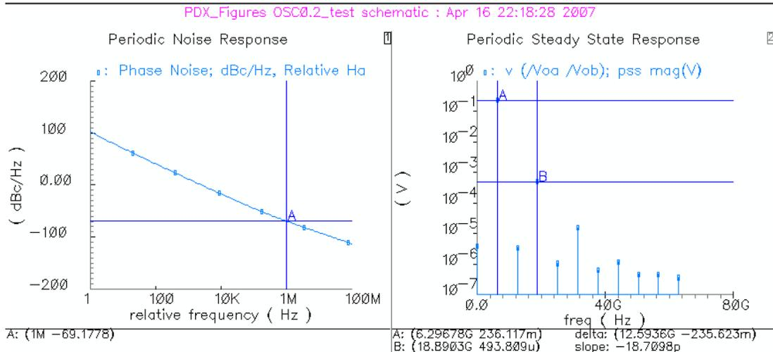
Figure 5-20 The simulated phase noise of the fabricated OSC0.2 core without output buffer is 4.1 dB worse than the example shown in Fig. 4-8 due to the smaller  $L$  in the tail biasing FET.
