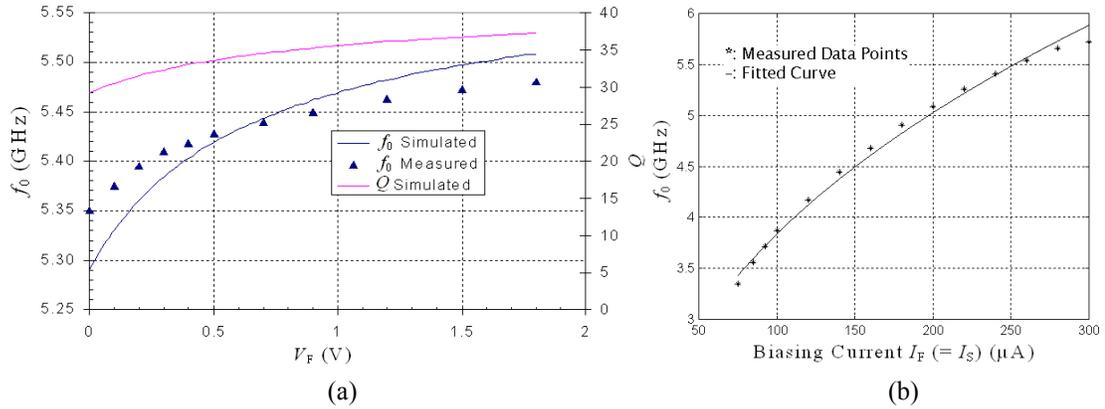
Figure 5-30 Tuning the filter center frequency ( $L_{\text{gate}} = 0.2 \mu\text{m}$ ): (a) frequency-tuning via the varactor voltage  $V_F$ ; (b) frequency-tuning via biasing currents  $I_F$  and  $I_S$ .
