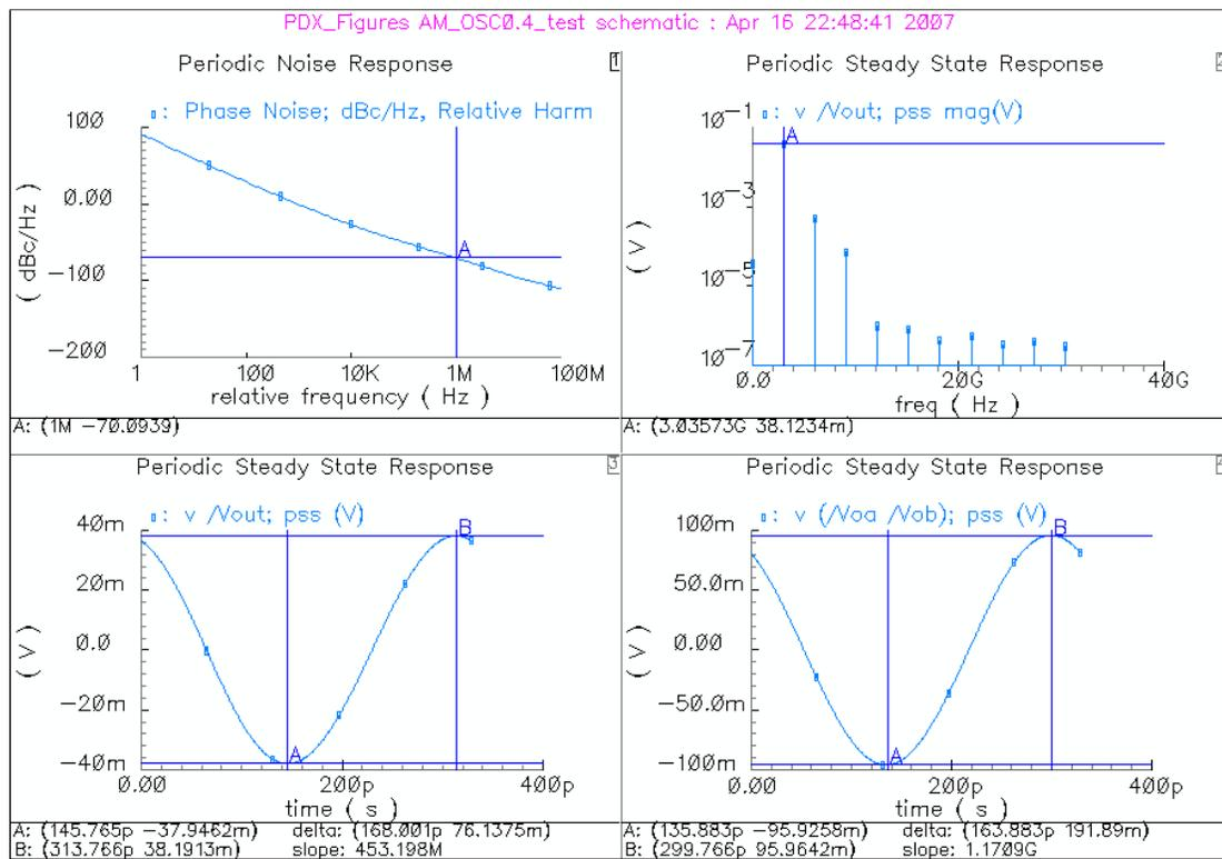
Figure 5-23 Simulation results of the fabricated 2.6-GHz oscillator with output buffer and load.
