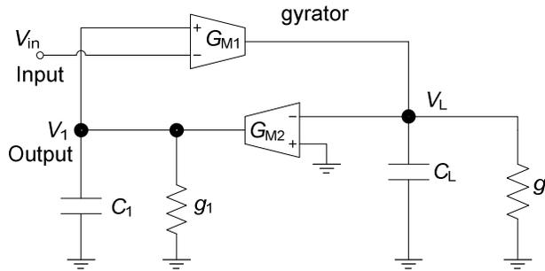
Figure 3-3 Reusing  $G_{M1}$  as input  $G_M$  to implement a lowpass filter.
