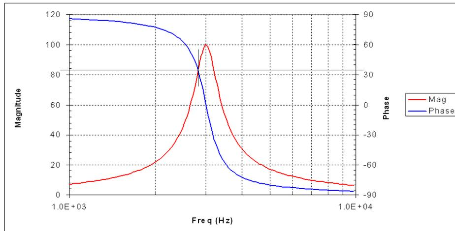
Figure 4-4 The magnitude and phase of an example shunt  $R-L-C$  resonator.
