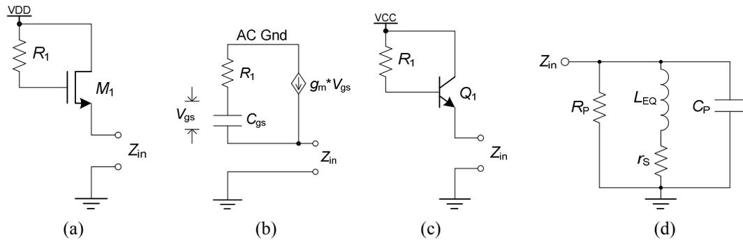
Figure 2-6 (a) CMOS gate- $R$  active inductor. (b) Small-signal ac equivalent circuit. (c) Bipolar version of the same circuit. (d) Equivalent circuit showing the inductor.
