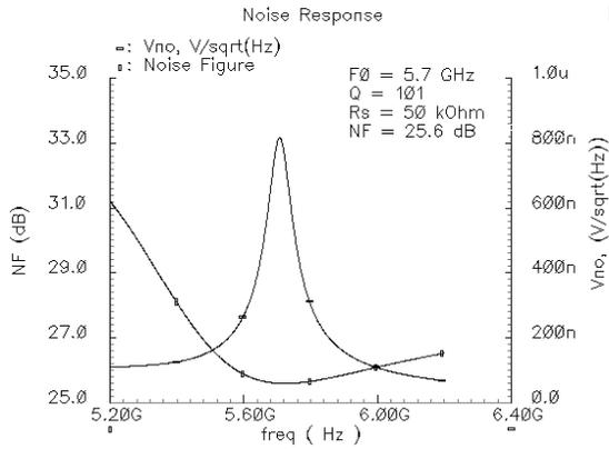
Figure 5-28 Simulated Noise Figure ( $R_S = 50 \text{ k}\Omega$ ) and equivalent output noise.
