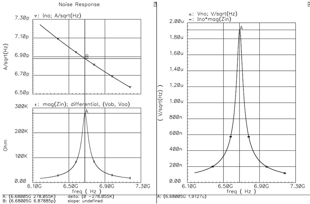
Figure 2-34 The noise of the active inductor shown in Fig. 2-29.
