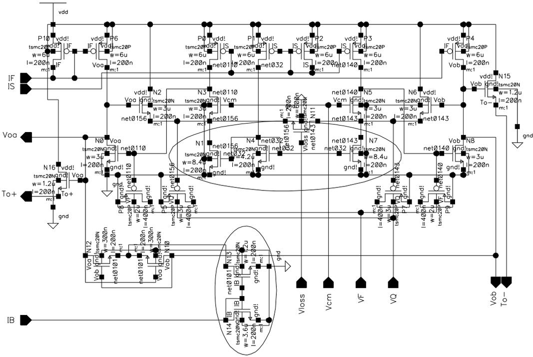
Figure 5-19 A minor design flaw in the fabricated oscillator, shown by the circle.
