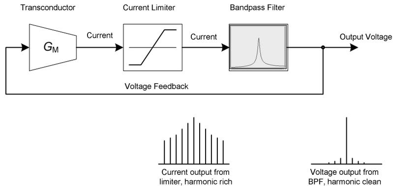
Figure 4-3 Active-inductor oscillator block diagram.
