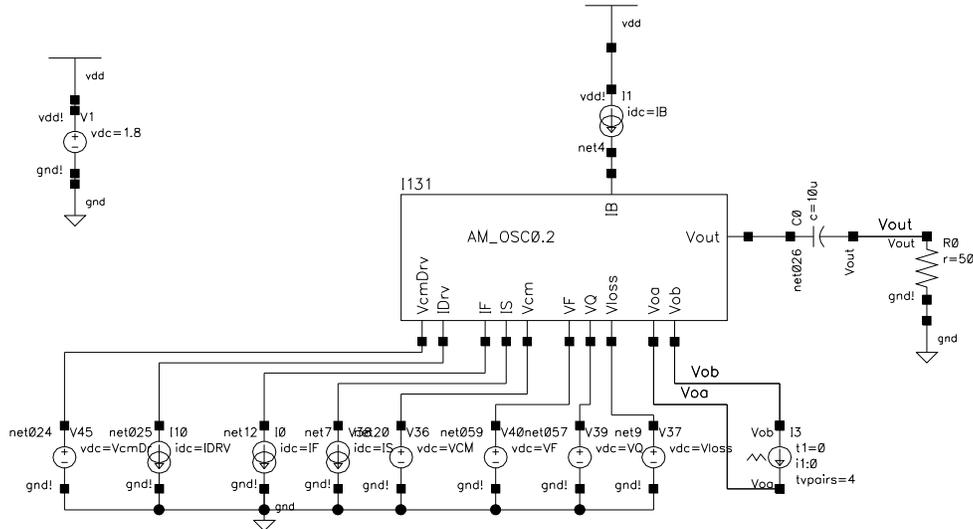
Figure 5-17 Test-bench configuration for the 5-GHz oscillator ( $L = 0.2\text{-}\mu\text{m}$ ).
