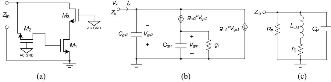
Figure 2-11 (a) CG-CS active inductor (Shinji Hara, 1989). (b) Small-signal ac circuit.  $g_1$  is mainly from the  $g_{ds}$  of the biasing transistor (not shown) for  $M_2$ . (c) Equivalent circuit.
