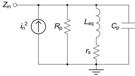
Figure 2-25 The noise model of an active inductor.
