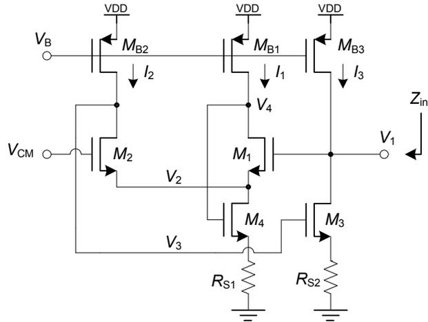
Figure 2-46 The all-NMOS-II circuit configured as an active inductor.
