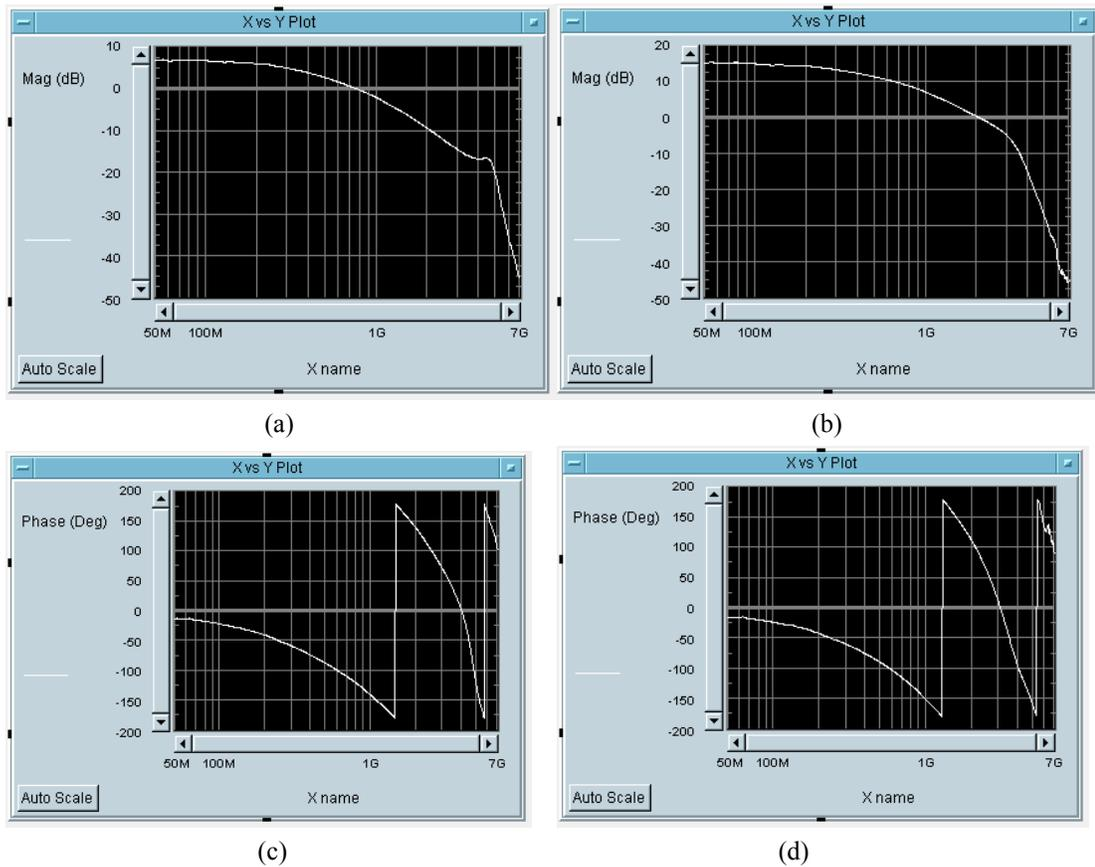
Figure 5-32 Examples of magnitude and phase responses of the module LP0.2, including the input buffer and the output driver. (a, c)  $Q$  is a little too high as shown by the peaking at the passband corner. The pole frequency is about 4.5 GHz; (b, d)  $Q$  is reduced via the loss resistor, resulting in less peaking. (Data Ref# LP0.2-C17-VNA-00010 and LP0.2-C17-VNA-00020)
