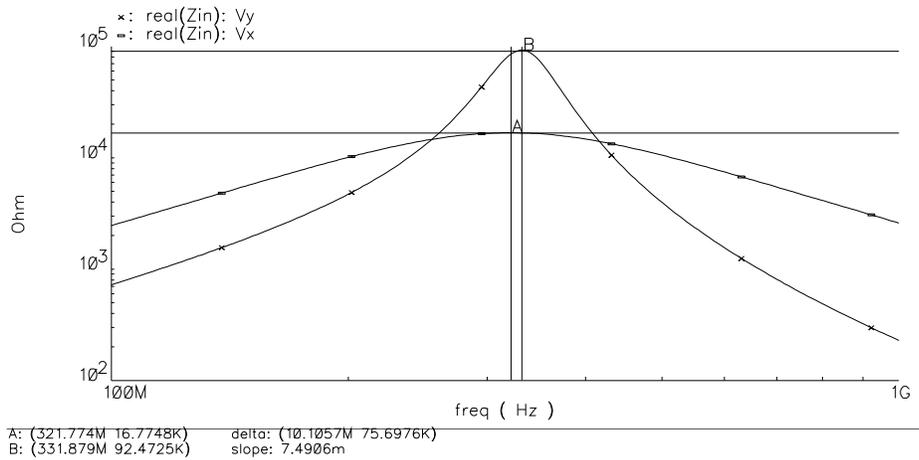
Figure 2-20 Simulated  $R_p$  of the circuits in Fig. 2-19. Cursor A and B are for circuit (a) and (b), respectively.
