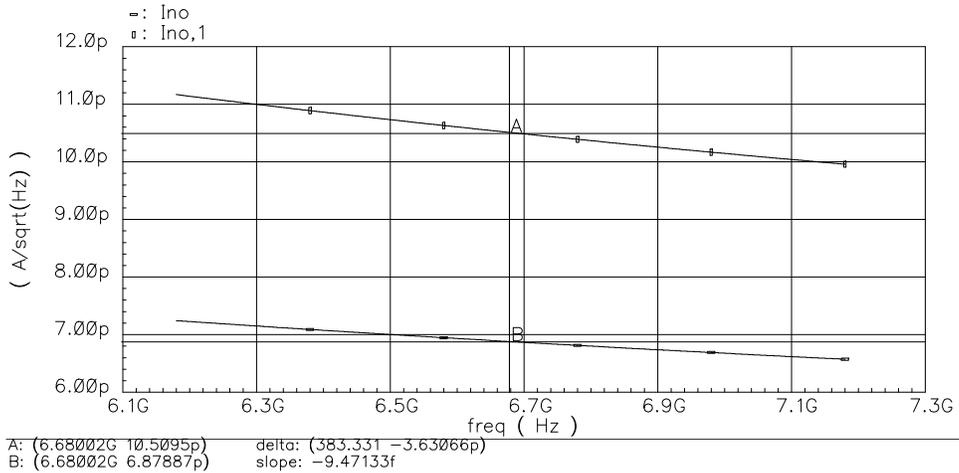
Figure 2-31 The equivalent output noise currents of the all-NMOS active inductor. The biasing conditions are the same as those in Fig. 2-29.
