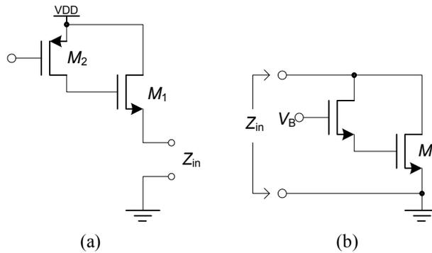
Figure 2-8 Gate-R (a) and Gate-R-II (b) active inductors using a linear-region FET as gate resistor.
