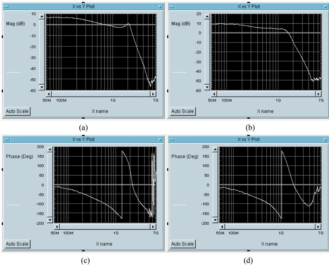
Figure 5-33 Examples of magnitude and phase responses of the module LP0.4, including the input buffer and the output driver. (a, c)  $Q$  is a little high, leading to peaking at the passband corner. The pole frequency is about 2 GHz; (b, d)  $Q$  is reduced via the loss resistor, leading to less peaking. (Data Ref# LP0.4-C17-VNA-00010 and LP0.4-C17-VNA-00020)
