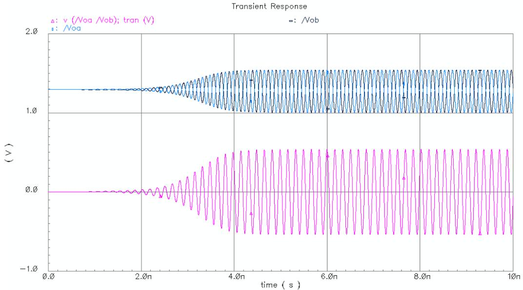
Figure 4-10 Transient simulation results of the oscillator (OSC0.2).
