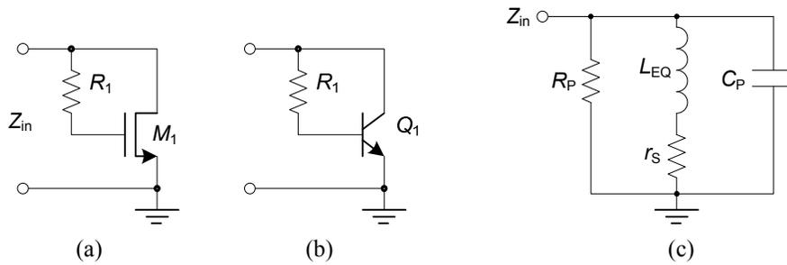
Figure 2-7 Gate-R-II active inductors and their small-signal equivalent circuit.
