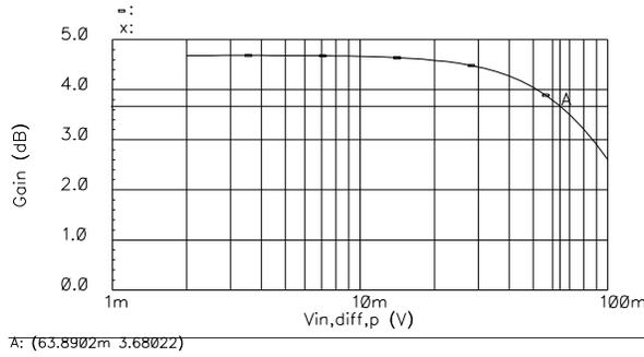
Figure 5-27 Simulation results for deriving the input 1-dB compression point, which is 0.128 Vpp, differentially.
