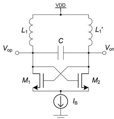
Figure 4-1 A passive  $L$ - $C$  oscillator.
