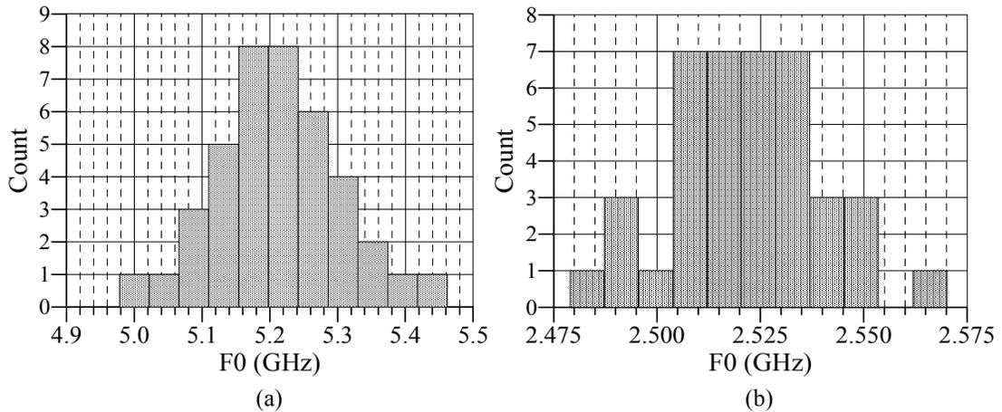
Figure 5-31 Histograms of oscillator  $f_0$  at nominal biasing. (a) 5-GHz oscillator,  $L_{\text{gate}} = 0.2 \mu\text{m}$ , OSC0.2; (b) 2.5-GHz oscillator,  $L_{\text{gate}} = 0.4 \mu\text{m}$ , OSC0.4.
