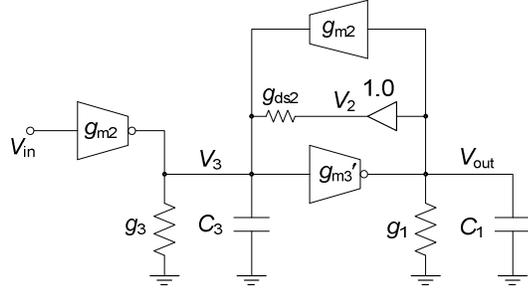
Figure 2-39 Small-signal equivalent circuit of the entire circuit.
