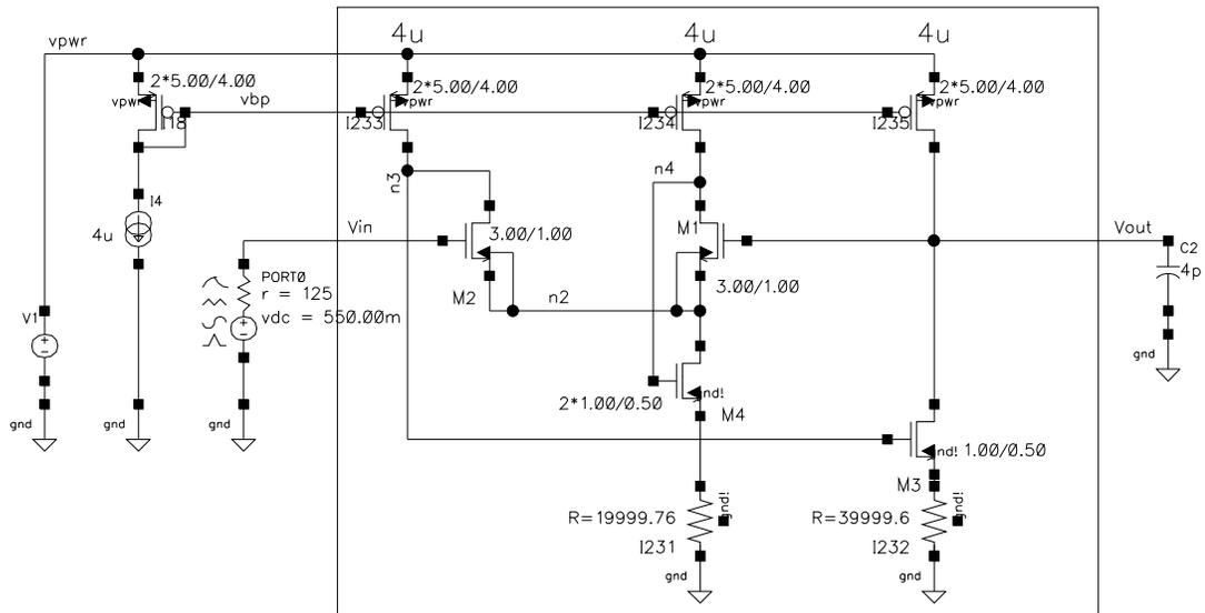
Figure 2-40 Example of All-NMOS-II circuit configured as an analog signal driver.
