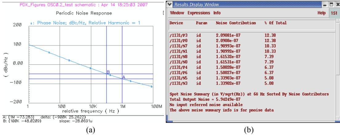
Figure 4-12 (a) Phase noise of the oscillator. (b) Noise summary.
