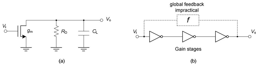
Figure 5-6 (a) A single gain stage. (b) Cascaded gain stages.
