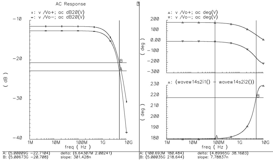
Figure 5-5 ac simulation results of the input buffer: magnitude (left) and phase (right).
