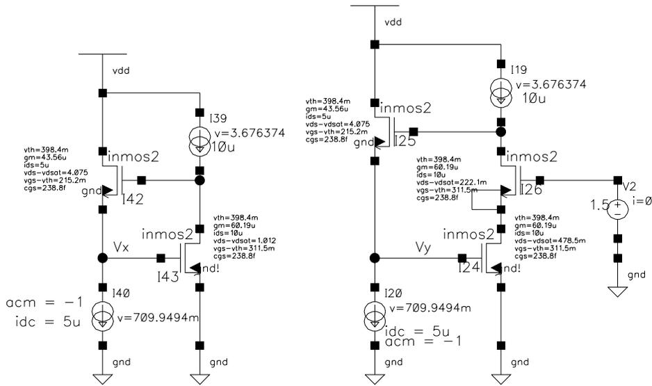
Figure 2-19 Simulation circuits to show the  $Q$  enhancement achieved by cascode. (a) CS-CD active inductor; (b) Cascode active inductor.
