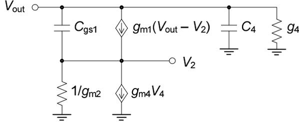
Figure 2-38 Small-signal equivalent circuit from  $V_{out}$  to  $V_2$ .
