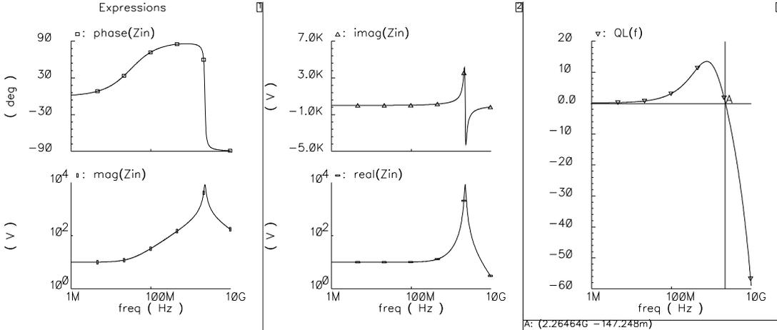
Figure 2-5 Simulation plots of the circuit in Fig. 2-4 with  $R_p = 1/g_p = 10 \text{ k}\Omega$ ,  $C_p = 100 \text{ fF}$ ,  $L_{eq} = 50 \text{ nH}$ ,  $r_s = 10 \Omega$ .
