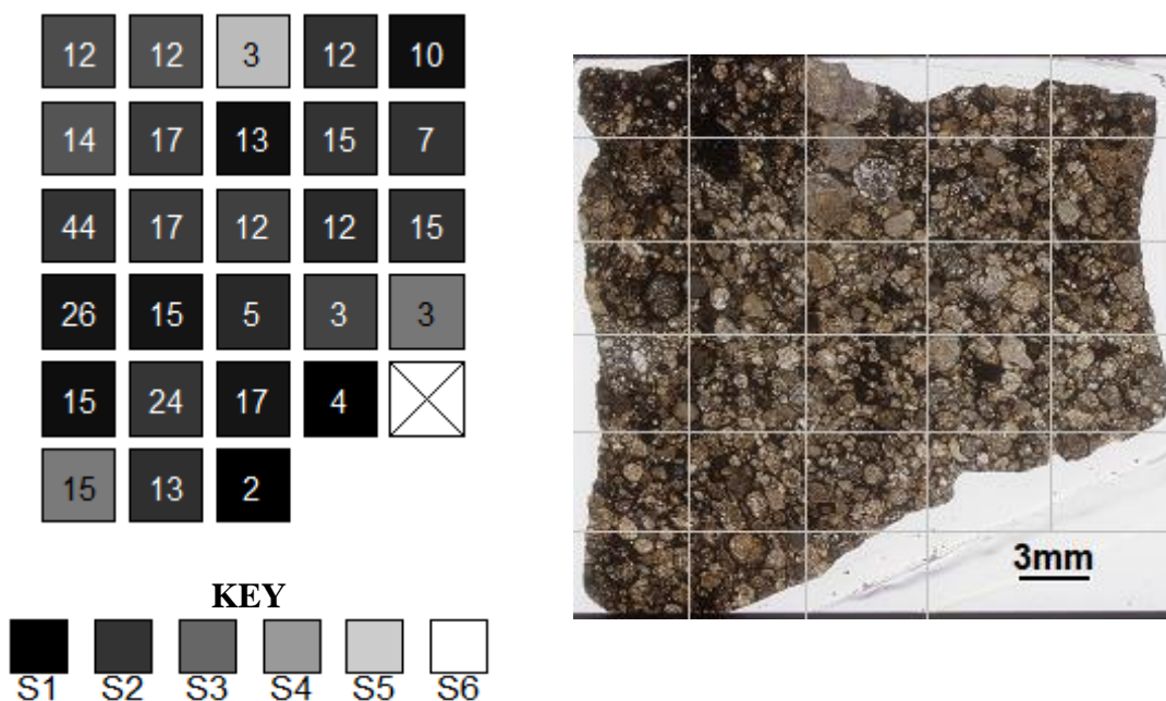
Figure 12. Shock Map of Sample CML 0244-2. Left image is a sectored shock map, and the right is an image of the sample in the same orientation. Numbers in the shock map sectors are the number of measured grains in those cells. Sector color is based on the weighted shock stage of a sector on the scale defined by the key. Sectors with an X have no grains usable for shock stage assessment.
