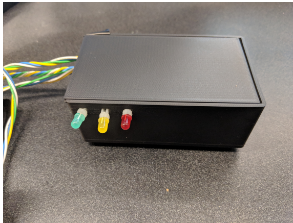
Figure 3.4: Image of the project box, containing the microcontroller inside, with wiring heading out to the IMU sensors.
