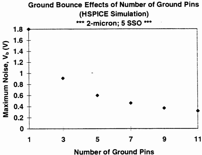
Figure 4.3: Ground Bounce versus Number of Ground Pins (HSPICE)
