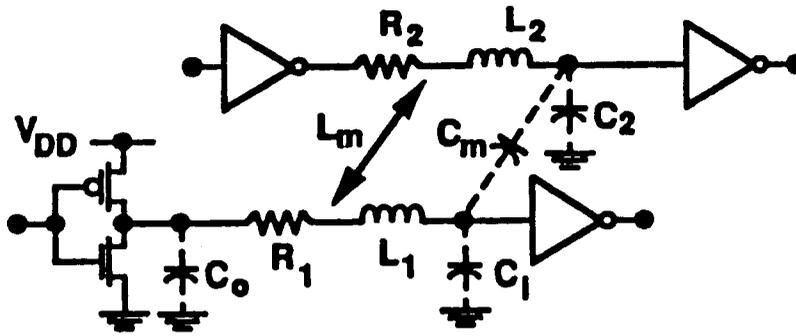
Figure 4.1: Lumped RLC Circuit Model
