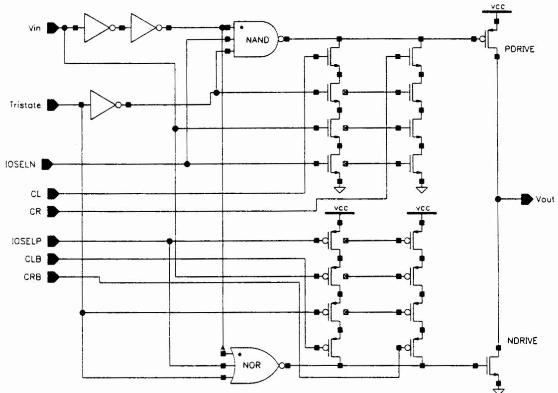
Figure 5.1: I/O Circuit with Self-Adjusting Slew Rate
