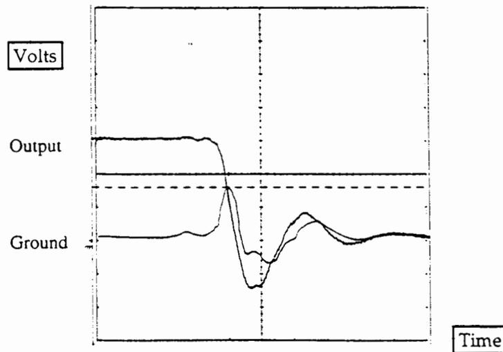
Figure 1.1: IC Noise from Simultaneous Output Switchings
