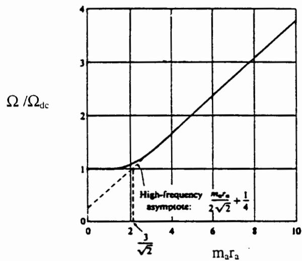
Figure 3.6: Effective Resistance versus Frequency
