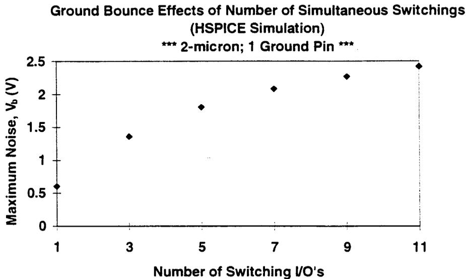
Figure 4.2: Ground Bounce versus Number of Switching I/O's (HSPICE)
