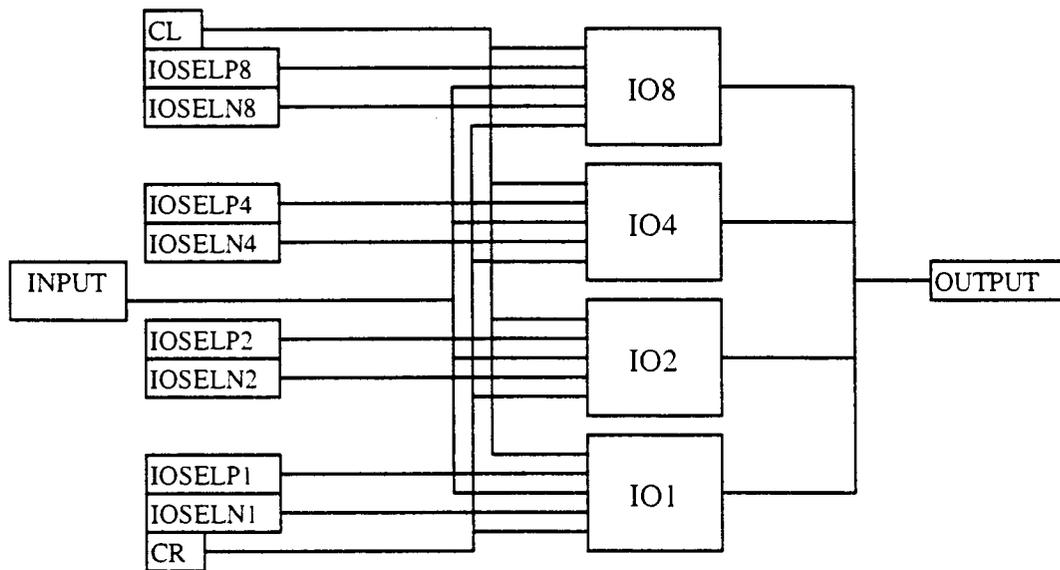
Figure 5.4: Proposed I/O Circuit
