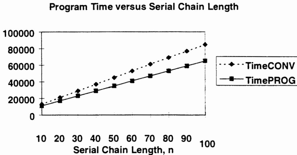
Figure 5.9: Program Time versus Serial Chain Length
