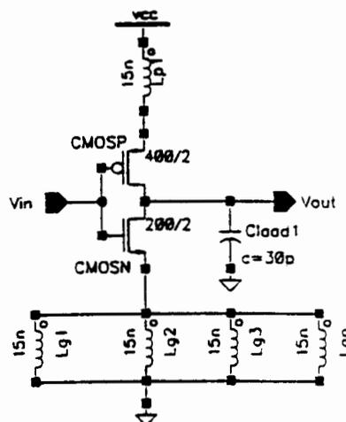
Figure 4.7: Simple Model for Ground Bounce versus Number of Ground Pins
