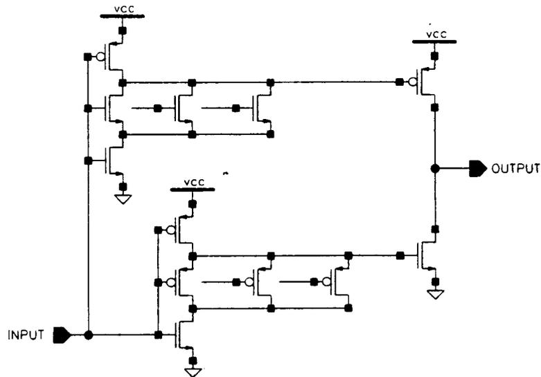
Figure 2.3: Current Controlling Output Buffer
