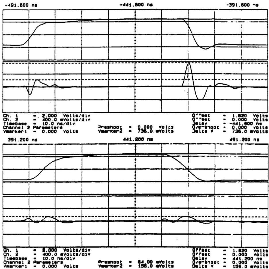
Figure 4.12: Ground Bounce with Different Slew Rates (MEASURED)
