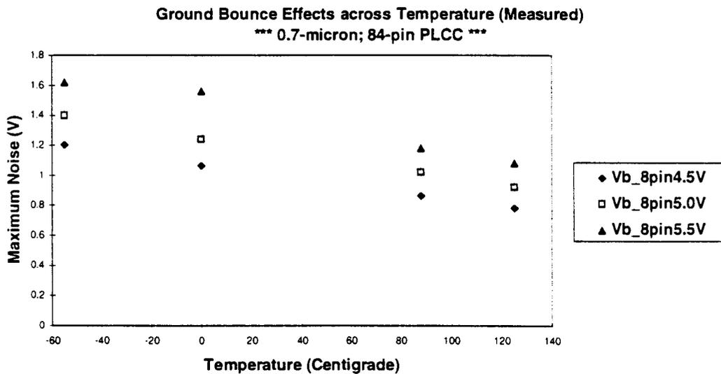
Figure 4.10: Ground Bounce versus Temperature (MEASURED)
