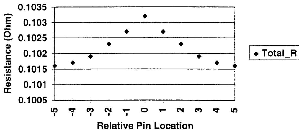
Figure 3.3: Pin Resistance versus Pin Location (PQFP 160)
