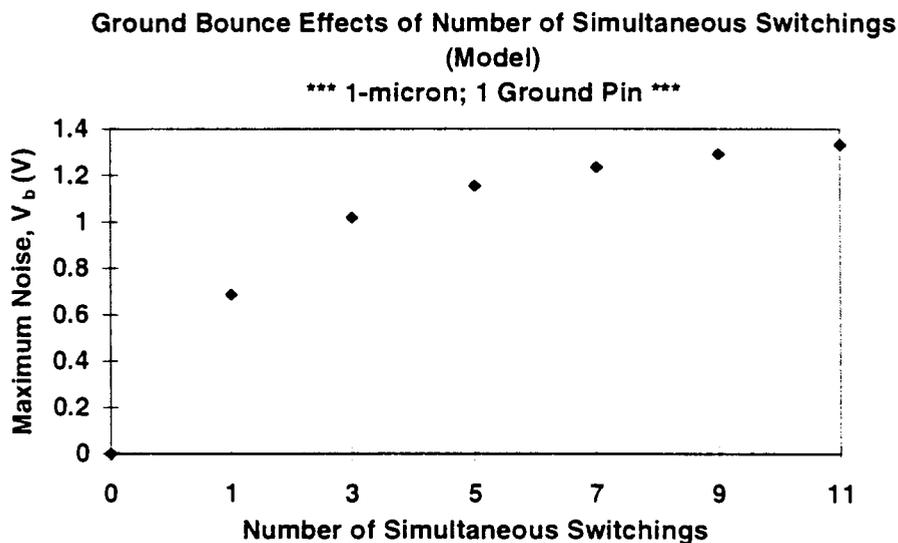
Figure 4.6: Ground Bounce versus Number of Switching I/O's (MODEL)
