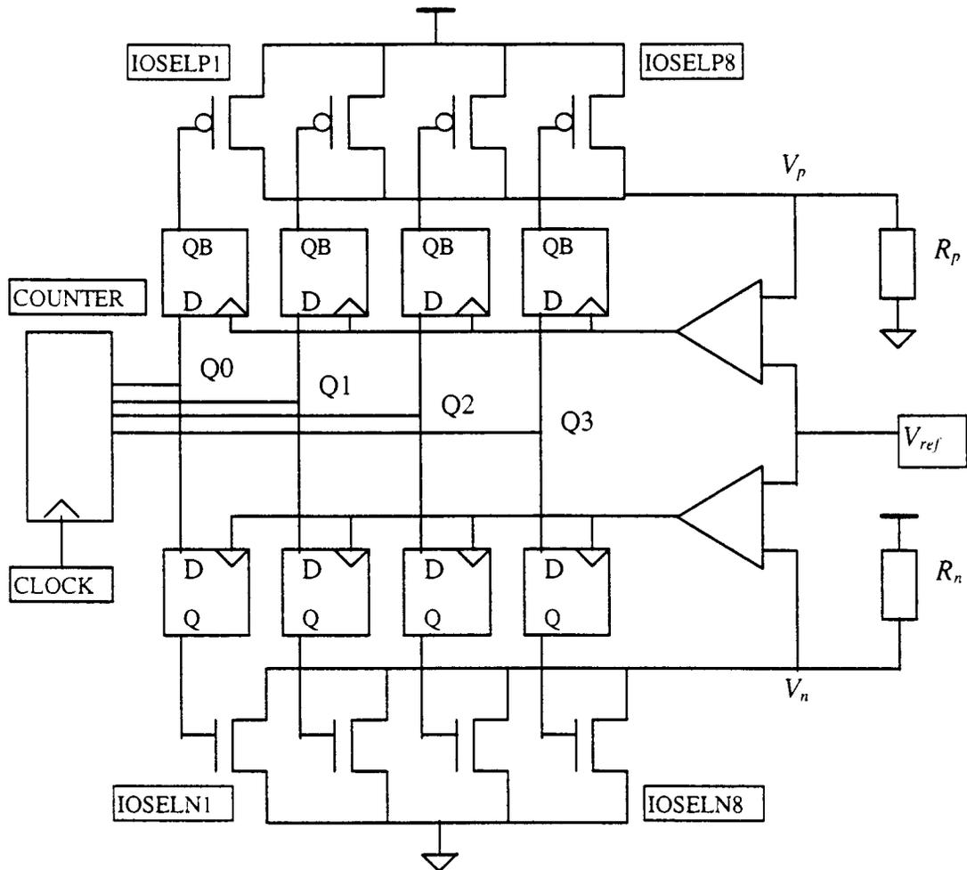
Figure 5.5: PVT-Compensated Control Circuit
