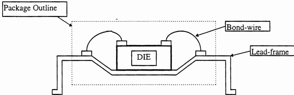
Figure 3.1: Cross-section of an IC Package
