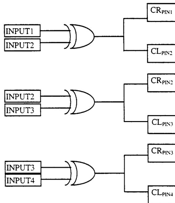
Figure 5.2: Output Switching Detection Circuit
