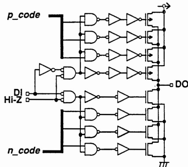
Figure 2.4: Output Buffer with Constant Current
