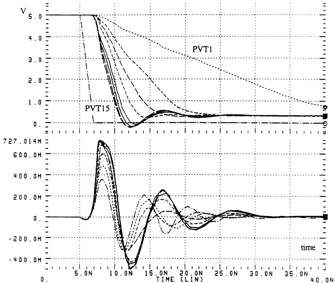
Figure 5.7: Simulation Results for PVT-Compensated I/O Circuit
