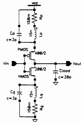
**Figure 2.2: Simplified Ground Bounce Circuit**
