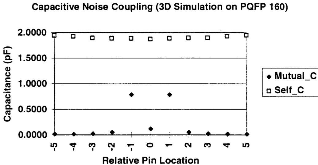
Figure 3.4: Pin Capacitance versus Pin Location (PQFP 160)
