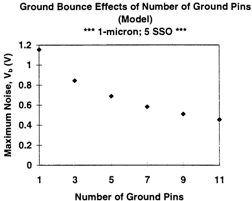
Figure 4.8: Ground Bounce versus Number of Ground Pins (MODEL)
