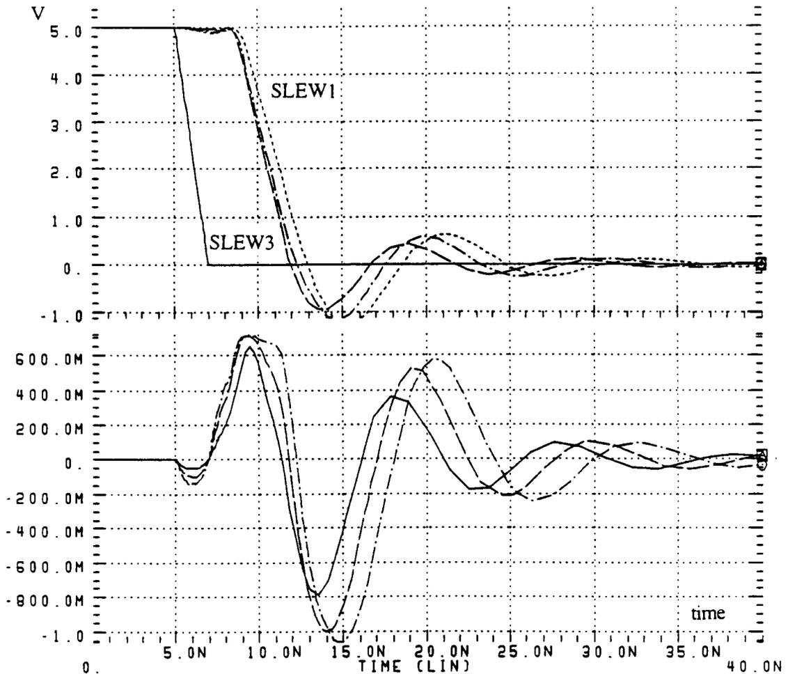
Figure 5.6: Simulation Results for I/O Circuit with Self-Adjusting Slew rate
