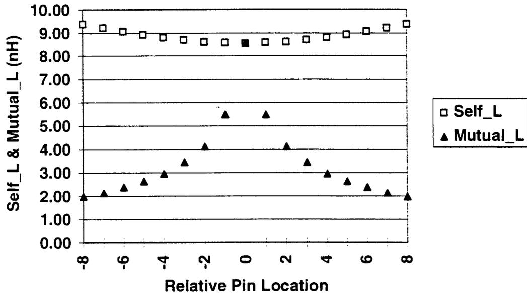
Figure 3.2: Pin Self and Mutual Inductance versus Pin Location (PQFP 160)
