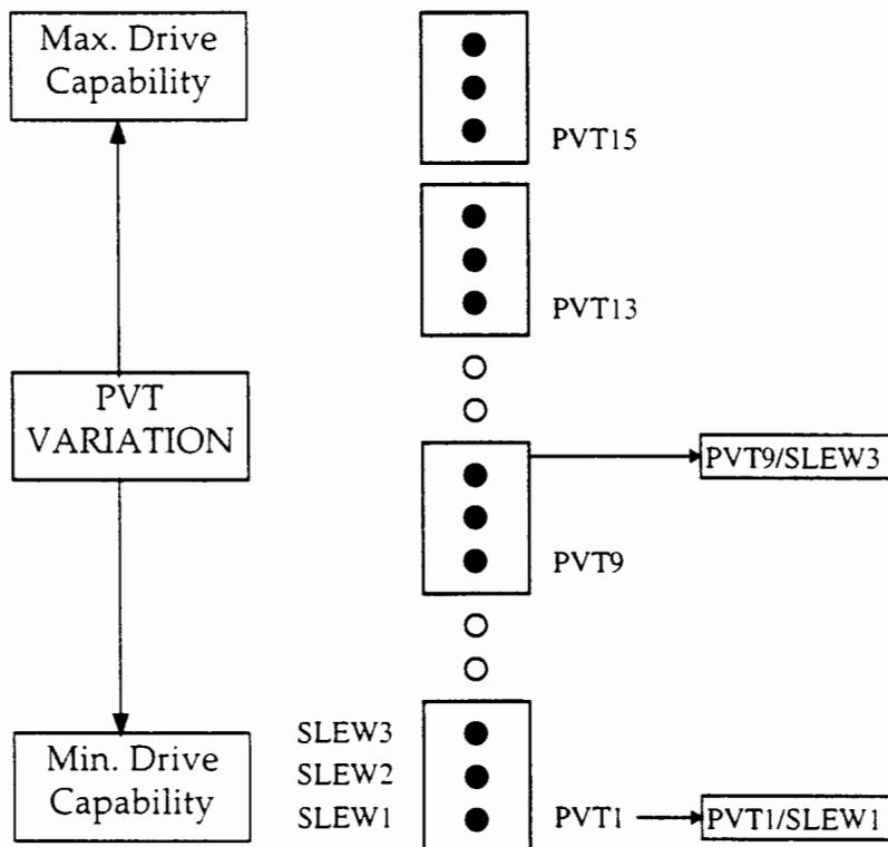
Figure 5.3: Current Control in the Proposed I/O Circuit
