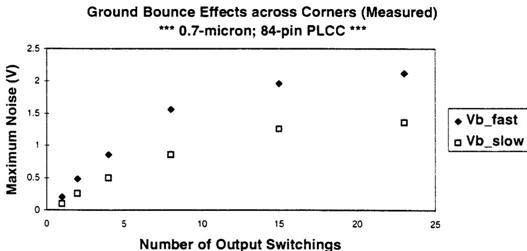
Figure 4.11: Ground Bounce versus Process Corners
