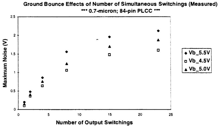
Figure 4.9: Ground Bounce versus Number of Switching I/O's (MEASURED)
