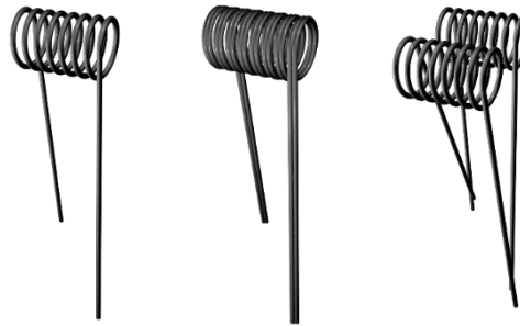
Figure 2. Illustration of single (left), parallel (middle) and dual coils. The parallel and dual coil contains two identical wires; however, the dual coils are wrapped individually with respective wicks. Each style can be oriented vertically or horizontally.
