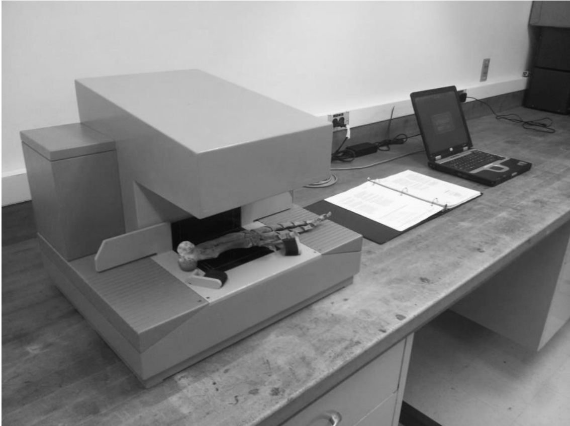
Figure 2-1. Bottlenose dolphin pectoral flipper skeletal specimen on a Norland Sabre pDEXA densitometer (Norland Medical Systems, Fort Atkinson, WI).
