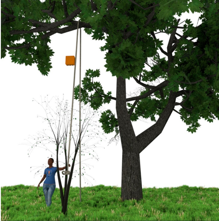
Figure 2.8. Installation of microclimate data loggers. Data logger (orange box) and rope enlarged to show detail.
