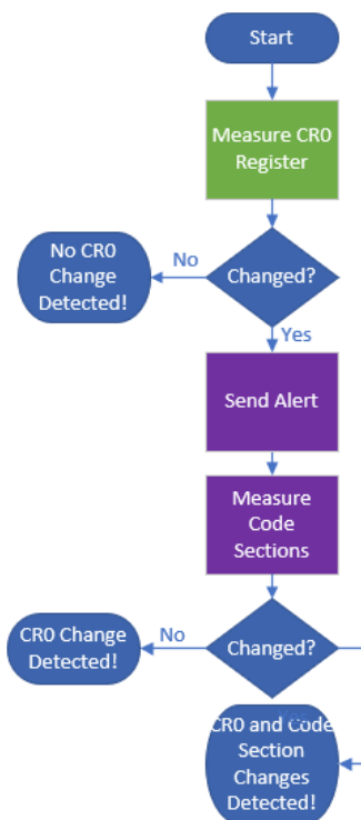
FIGURE 7.4: Persistent Kernel Code Section and CR0 Trigger. Purple boxes are dependent actions.
