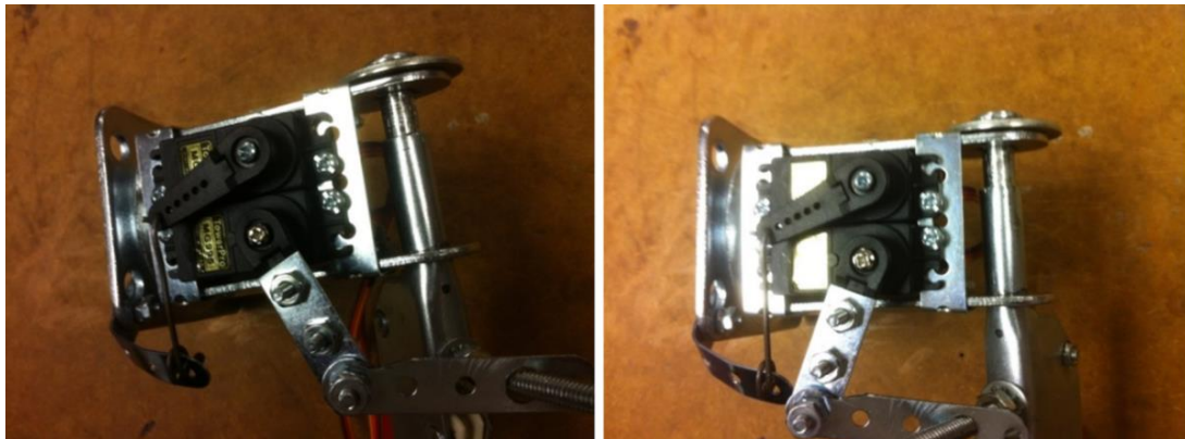
Figure 23 – Robot Shoulder Left/Right Motion. The servo arm moves a jointed bracket forward and back over a bolt attached to the shoulder. This translates to left/right shoulder motion.
