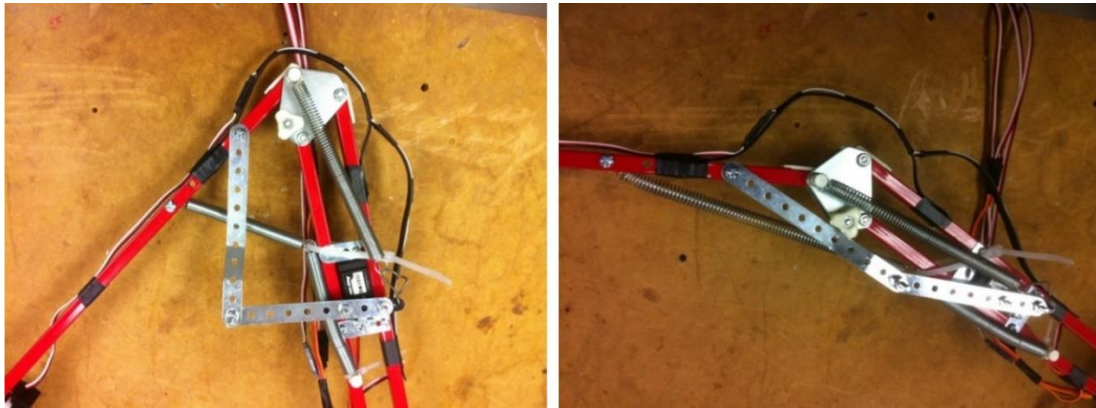
Figure 22 – Robot Elbow Range of Motion . A hinged bracket is attached to the elbow servo arm and reduces the torque and power needed to flex and extend the robot drumming arm.
